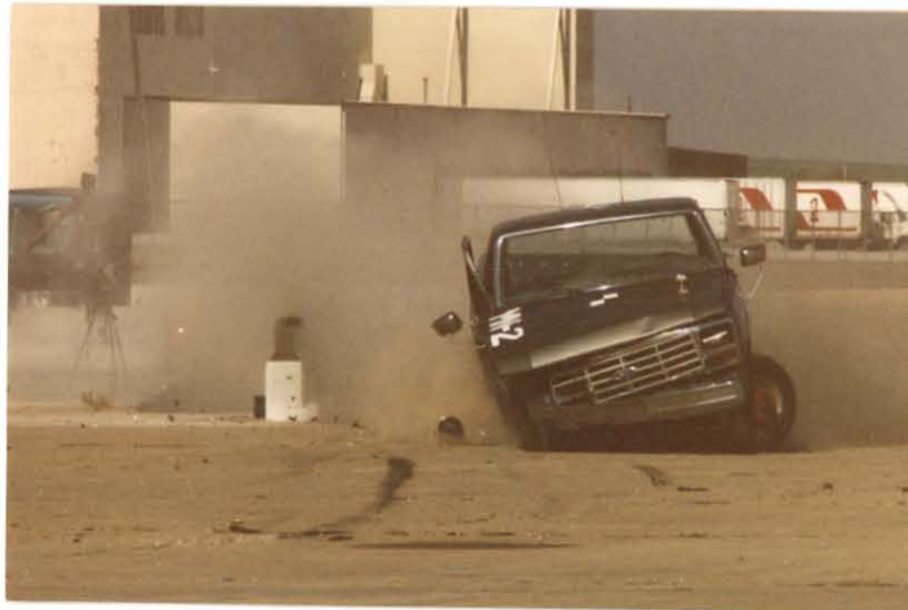
Figure 20. Full-scale Vehicle Crash Test MN-2.
