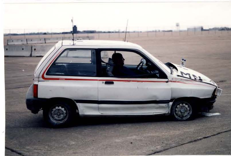
Figure 31. Vehicle Damage, Test MN-4.
