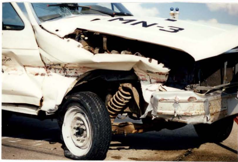
Figure 27. Vehicle Damage, Test MN-3.
