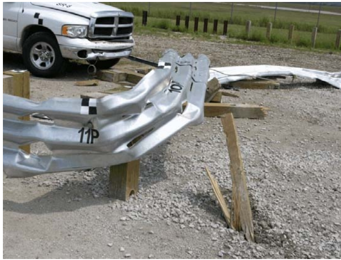
Figure 86. System Damage, Test SR-8
