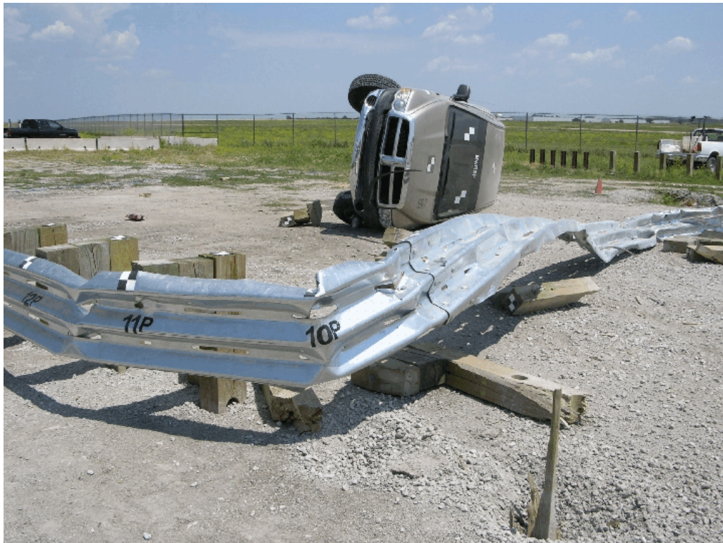
Figure 44. System Damage, Test SR-7
