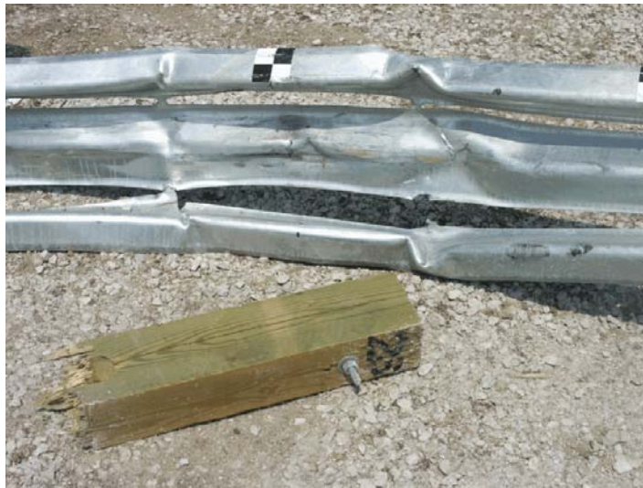
Figure 87. System Damage, Test SR-8
