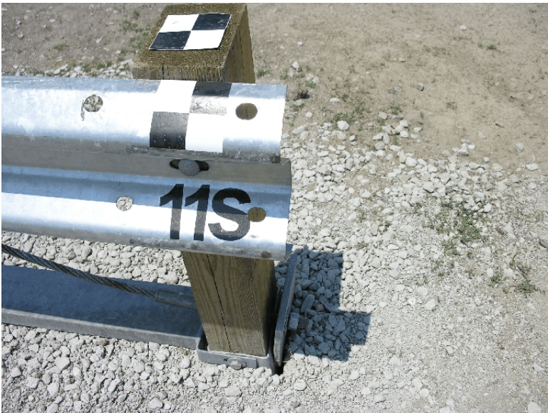
Figure 49. Post Nos. 10 and 11 Damage, Test SR-7
