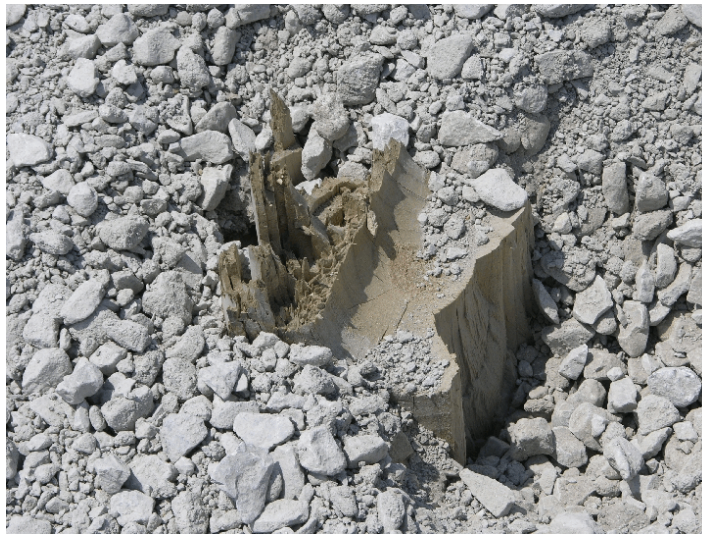
Figure 52. Post Nos. 3S through 5S Damage, Test SR-7
