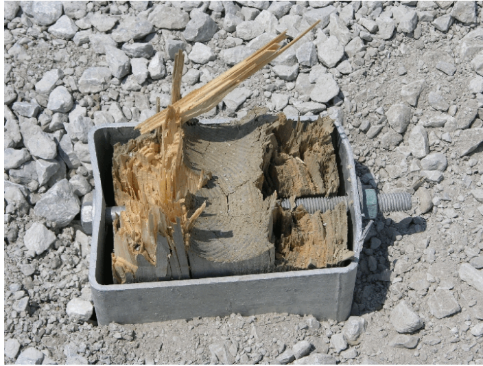
Figure 53. Post Nos. 1P, 1S and 2S Damage, Test SR-7
