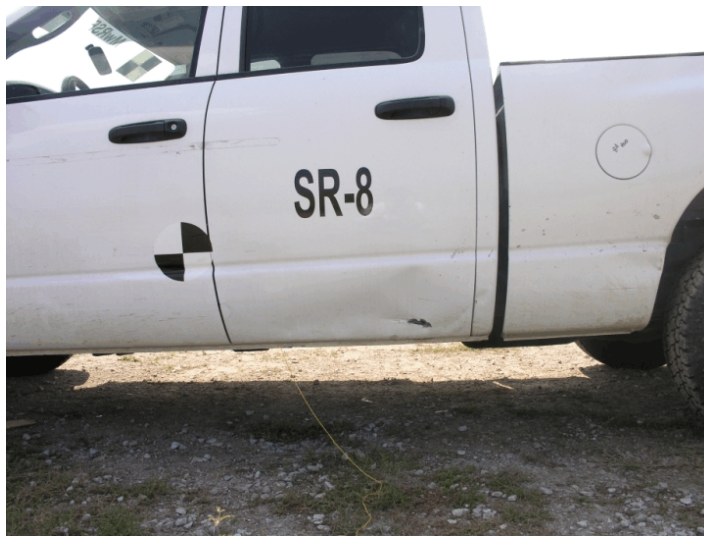
Figure 95. Vehicle Damage, Test SR-8
