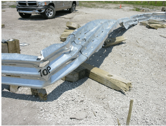
Figure 45. System Damage, Test SR-7
