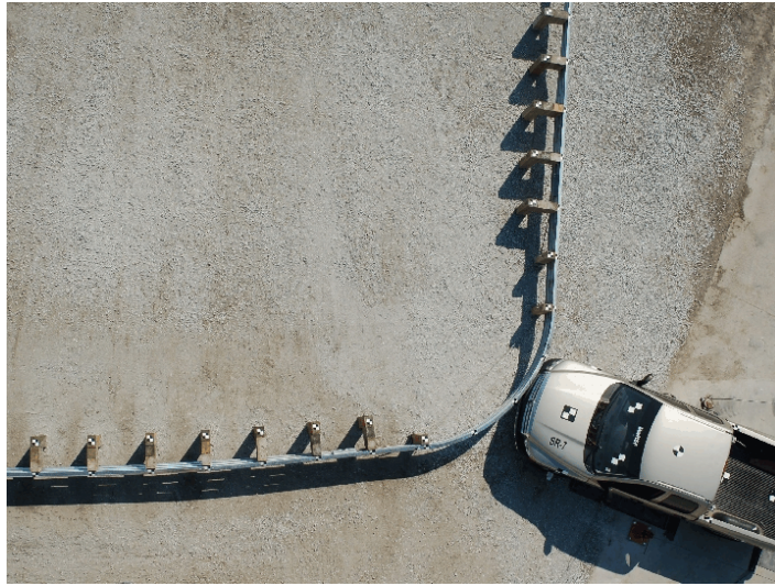
Figure 39. Impact Location, Test SR-7
