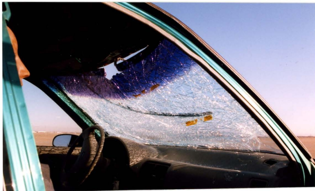
Figure 28. Windshield Damage, Test M-2
