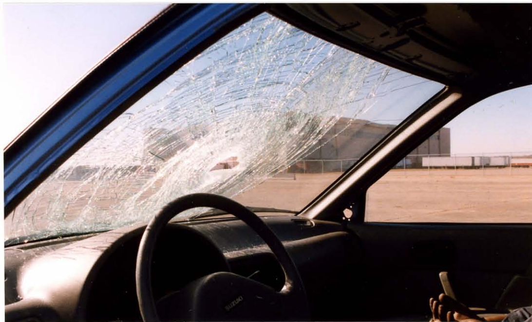
Figure 20. Windshield Damage, Test M-1
