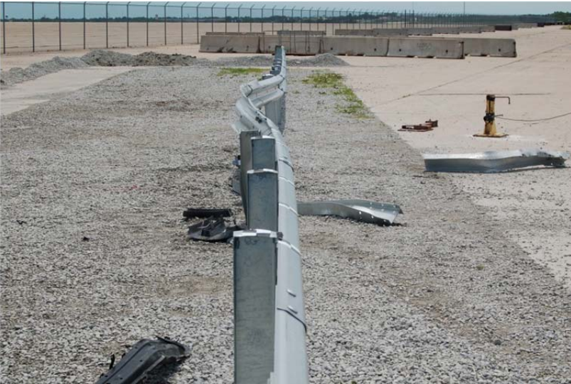
Figure 54. System Barrier Damage, Test No. MGSNB-2
