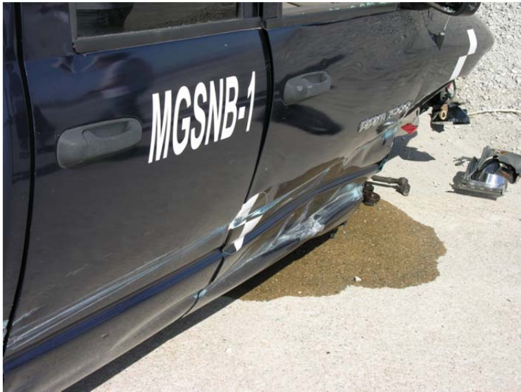
Figure 45. Vehicle Damage, Test No. MGSNB-1
