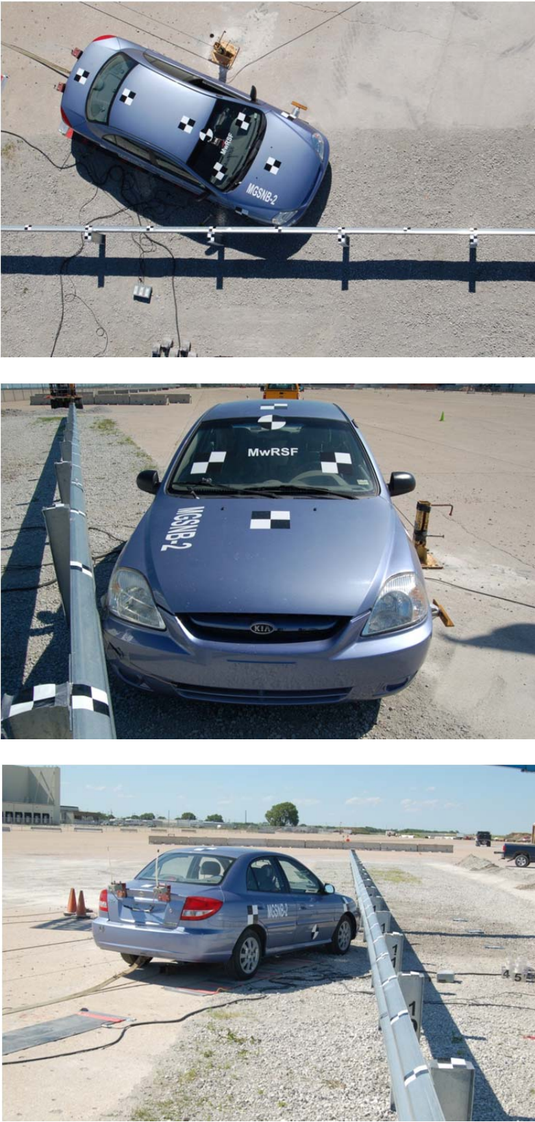
Figure 52. Impact Location, Test No. MGSNB-2
