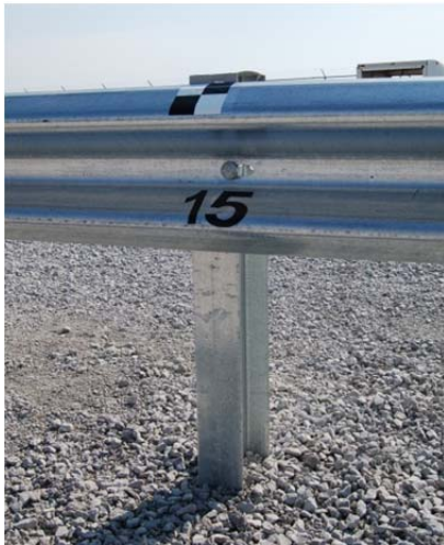
Figure 65. Bolt Located in Worst Case Location – Pull-Through Behavior Still Occurred
