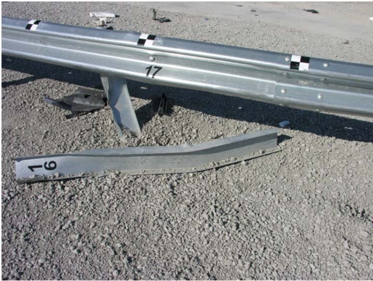
Figure 56. Post Damage between Posts 15 and 17, Test No. MGSNB-2
