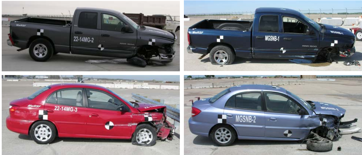
FIGURE 7 Vehicle Damage (left – blocked tests, right – non-blocked tests)
