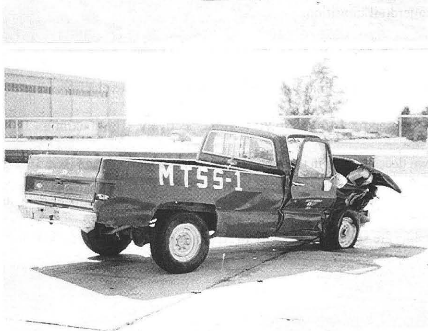
Figure 21. Vehicle Damage, Test MTSS-1
