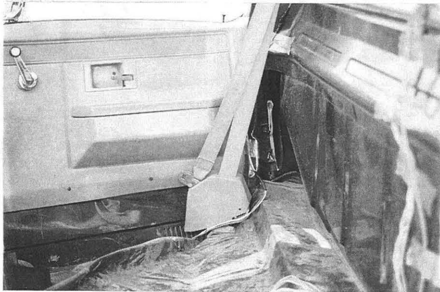
Figure 27. Occupant Compartment Deformation, Test MTSS-1 (Con't)
