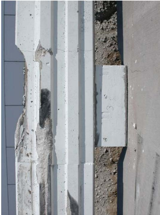
Figure 42. Traffic-Side Bridge Rail Damage at Post Nos. 1 through 4, Test ACBR-1
