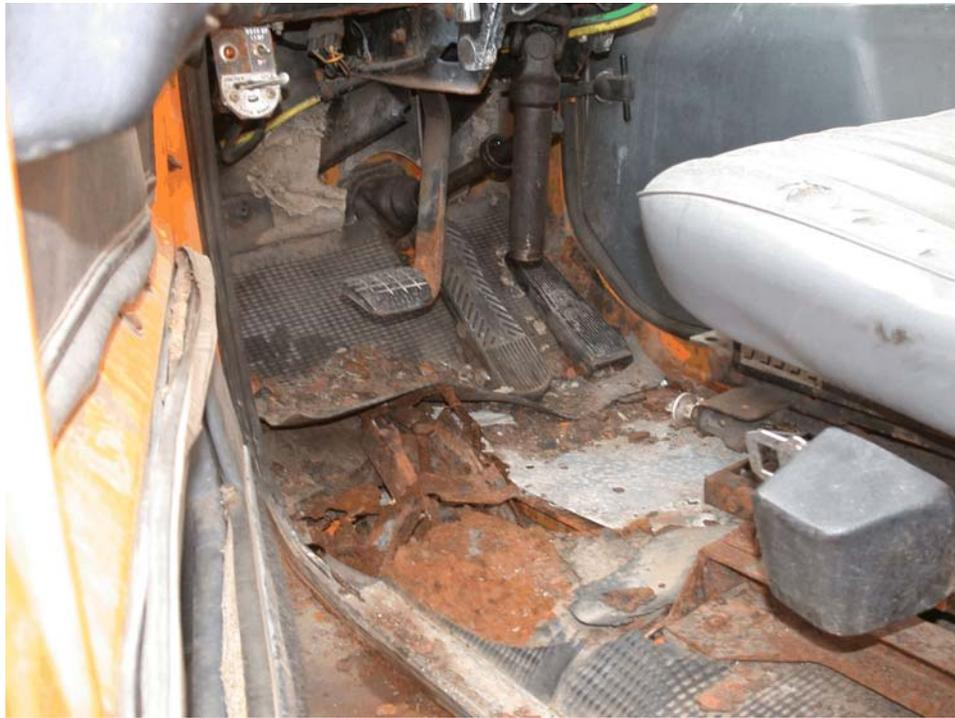
Figure 58. Occupant Compartment Damage, Test ACBR-1
