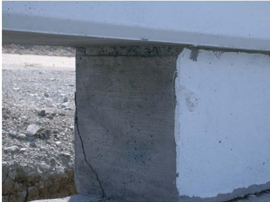
Figure 52. Bridge Post No. 7 Damage, Test ACBR-1
