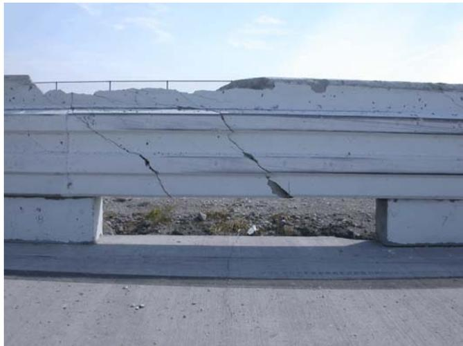
Figure 39. Traffic-Side Bridge Rail Damage at Spans Between Post Nos. 5 through 8, Test ACBR-1
