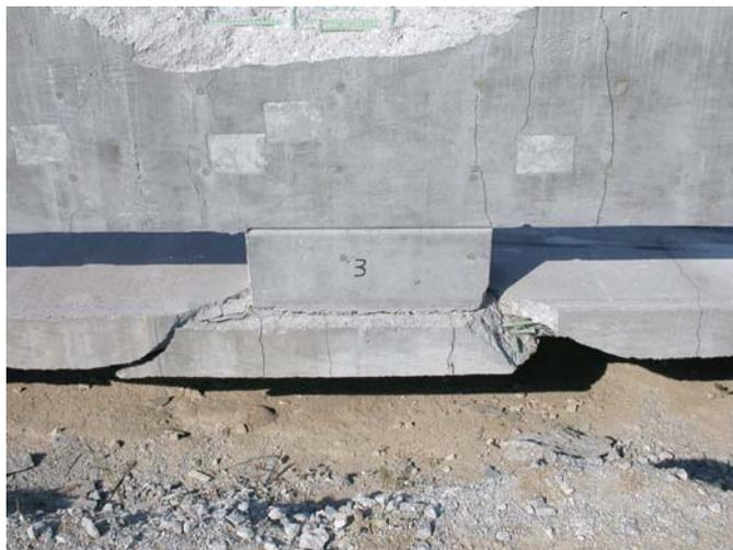
Figure 46. Back-Side Bridge Rail and Deck Damage at Post Nos. 1 through 3, Test ACBR-1
