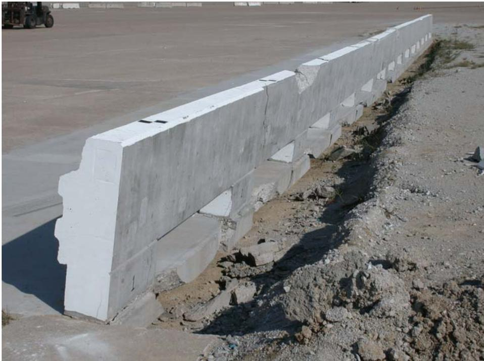
Figure 34. Bridge Rail Damage, Test ACBR-1
