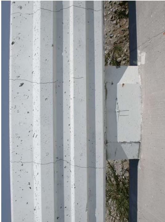
Figure 44. Traffic-Side Bridge Rail Damage at Post Nos. 9 through 12, Test ACBR-1
