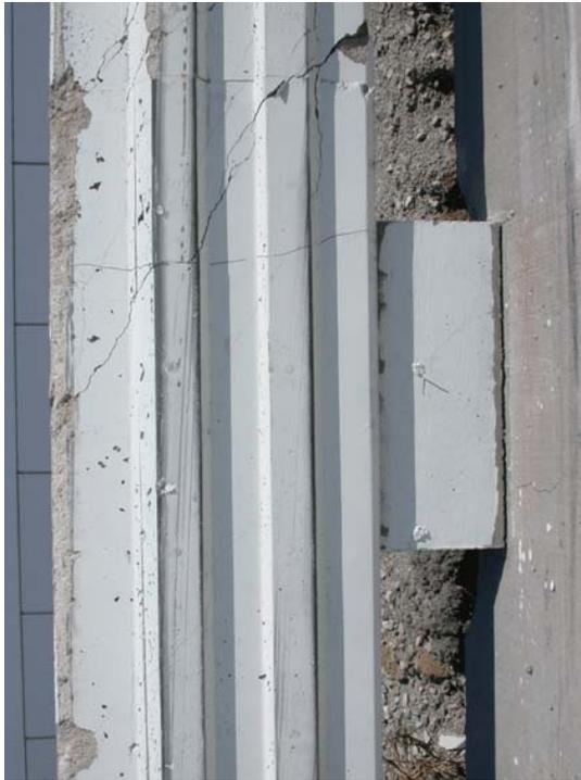
Figure 43. Traffic-Side Bridge Rail Damage at Post Nos. 5 through 8, Test ACBR-1
