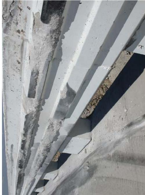
Figure 37. Bridge Rail Damage, Test ACBR-1
