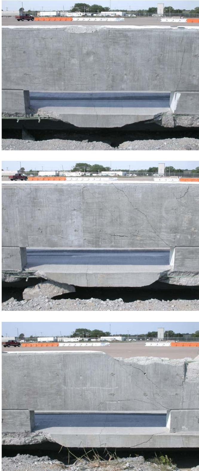
Figure 41. Back-Side Bridge Rail Damage at Spans Between Post Nos. 5 through 8, Test ACBR-1
