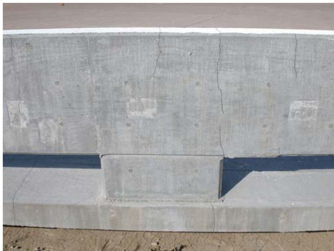
Figure 48. Back-Side Bridge Rail and Deck Damage at Post Nos. 7 through 9, Test ACBR-1
