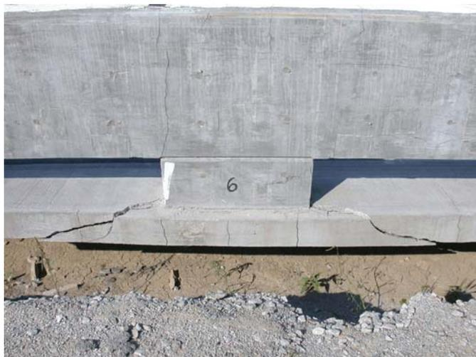
Figure 47. Back-Side Bridge Rail and Deck Damage at Post Nos. 4 through 6, Test ACBR-1
