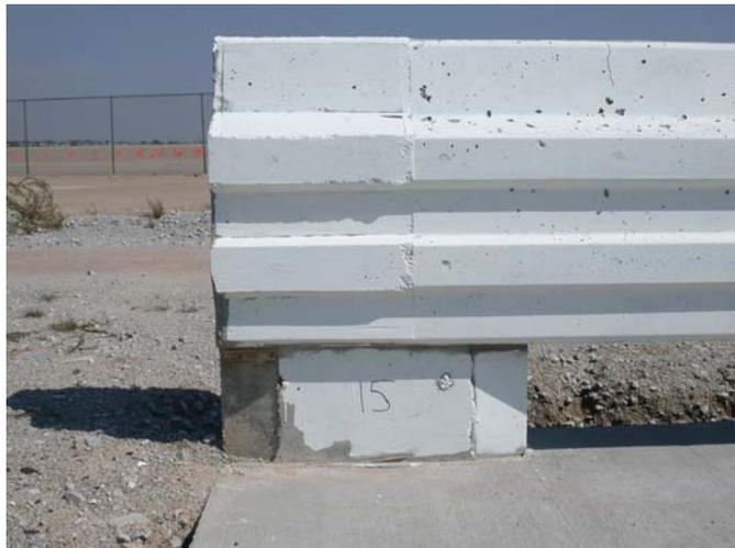
Figure 45. Traffic-Side Bridge Rail Damage at Post Nos. 13 through 15, Test ACBR-1
