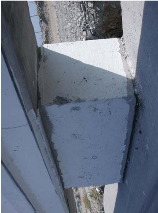
Figure 51. Bridge Post Nos. 5 and 6 Damage, Test ACBR-1
