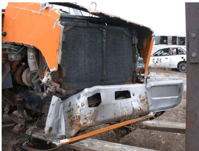
Figure 54. Vehicle Damage, Test ACBR-1
