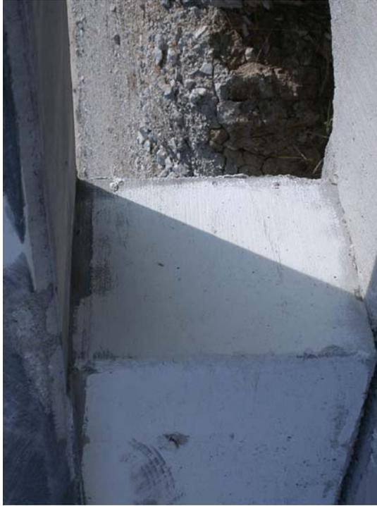
Figure 50. Bridge Post Nos. 3 and 4 Damage, Test ACR-1
