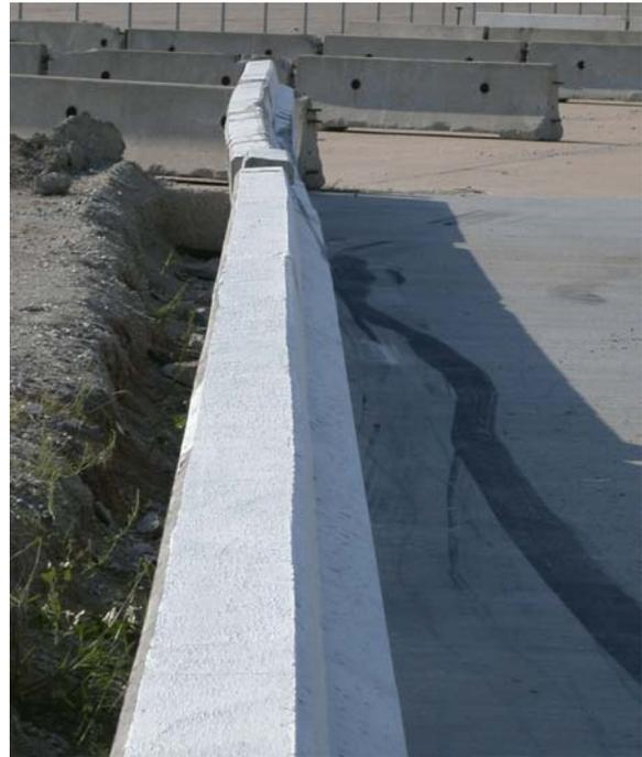
Figure 35. Bridge Rail Damage, Test ACBR-1
