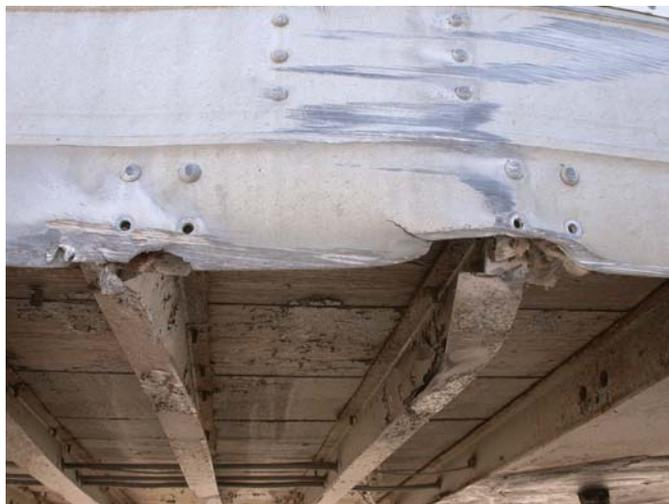
Figure 56. Vehicle Damage, Test ACBR-1
