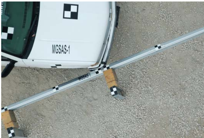
Figure 25. Impact Location, Test No. MGSAS-1
