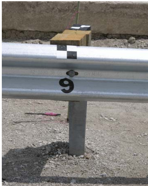
Figure 29. Post Nos. 9 through 11 Damage, Test No. MGSAS-1
