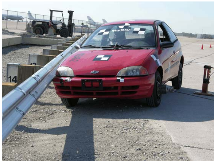
Figure 41. Impact Location, Test No. MGSAS-2
