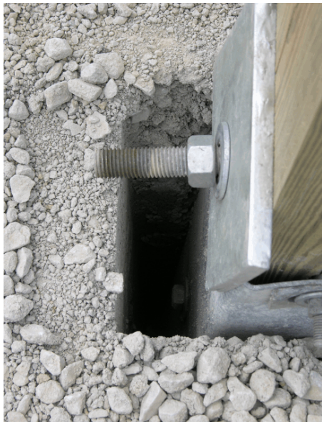
Figure 32. Anchorage Damage, Test No. MGSAS-1
