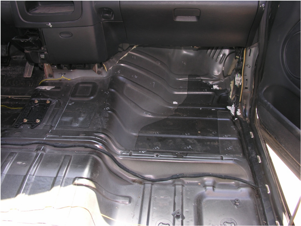
Figure 36. Interior Occupant Compartment Deformation, Test No. KSFRP-1
