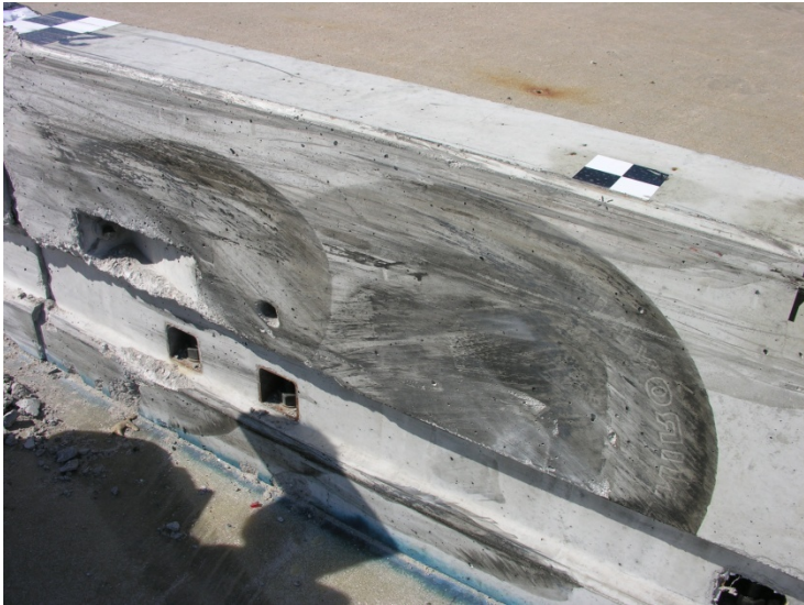
Figure 29. Barrier No. 2 Damage, Test No. KSFRP-1
