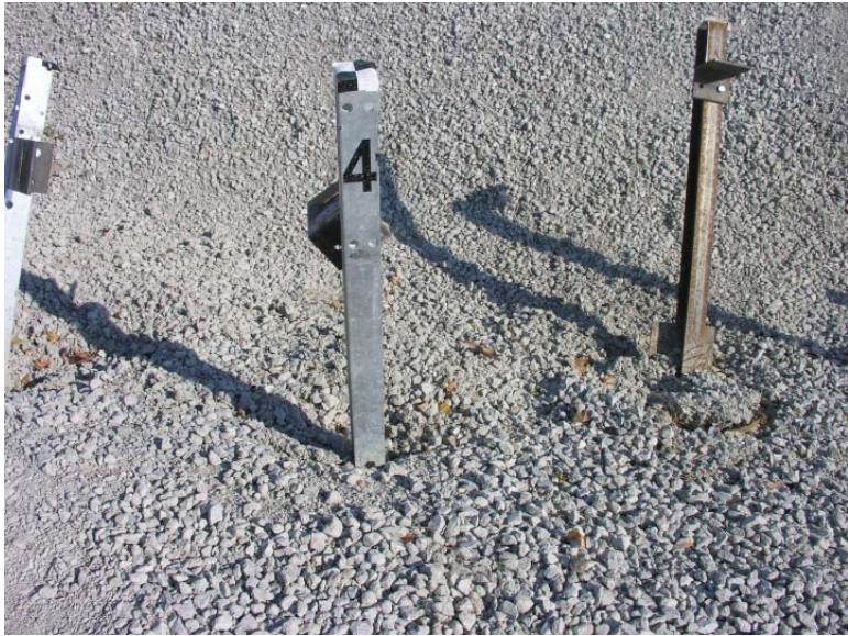
Figure 215. Post Nos. 3 and 4 Damage, Test No. NYBBT-7
