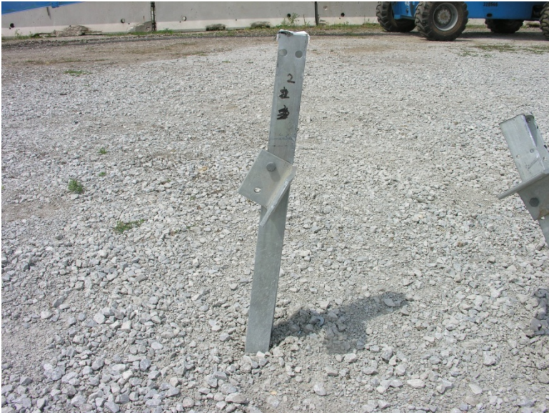
Figure 284. Post Nos. 1 and 2 Damage, Test No. NYBBT-9
