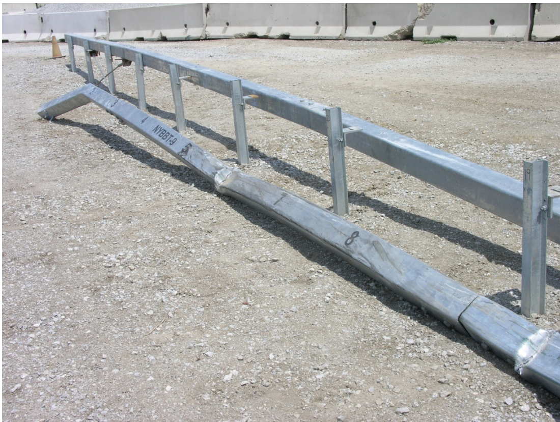
Figure 281. Barrier Damage, Test No. NYBBT-9
