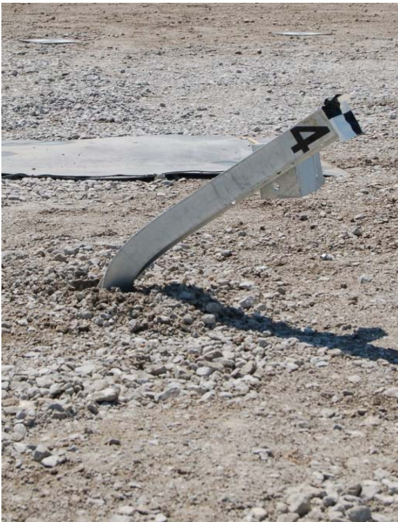
Figure 126. Post Nos. 3 and 4 Damage, Test No. NYBBT-4
