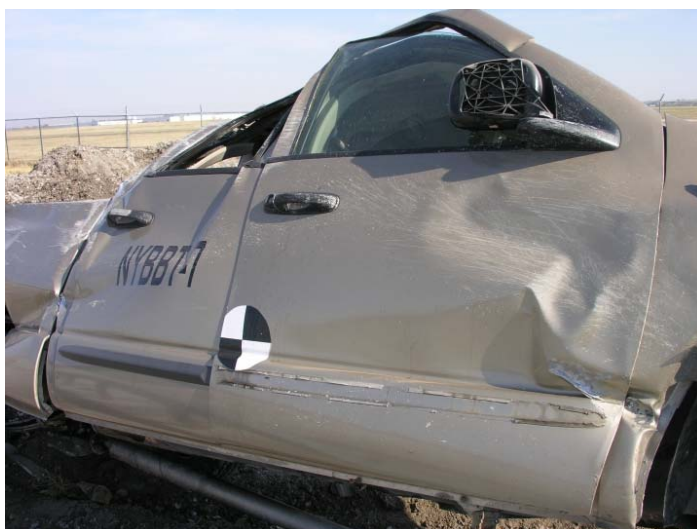
Figure 225. Vehicle Damage, Test No. NYBBT-7 (Note: Vehicle shown is after it was rolled back over)
