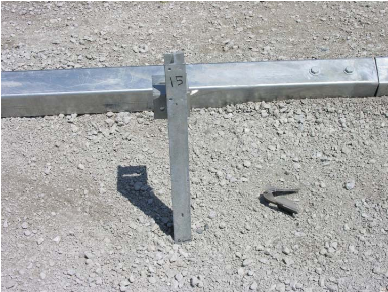
Figure 261. Post Nos. 13 through 16 Damage, Test No. NYBBT-8
