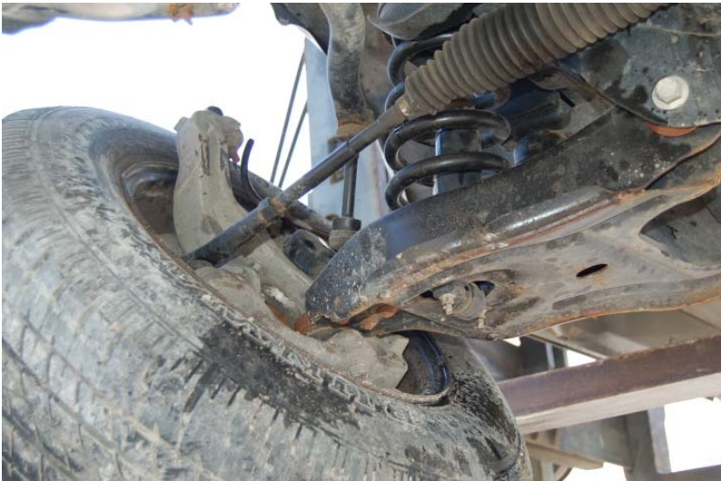
Figure 168. Undercarriage Damage, Test No. NYBBT-5
