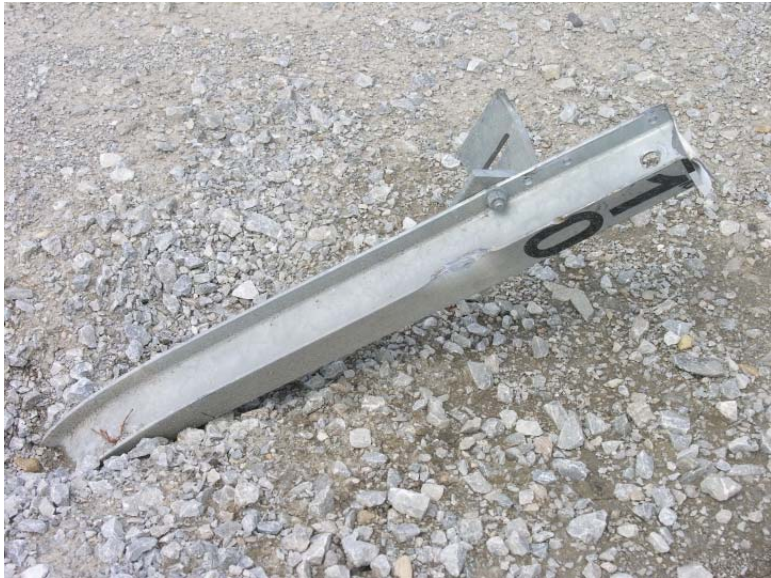
Figure 129. Post Nos. 9 and 10 Damage, Test No. NYBBT-4
