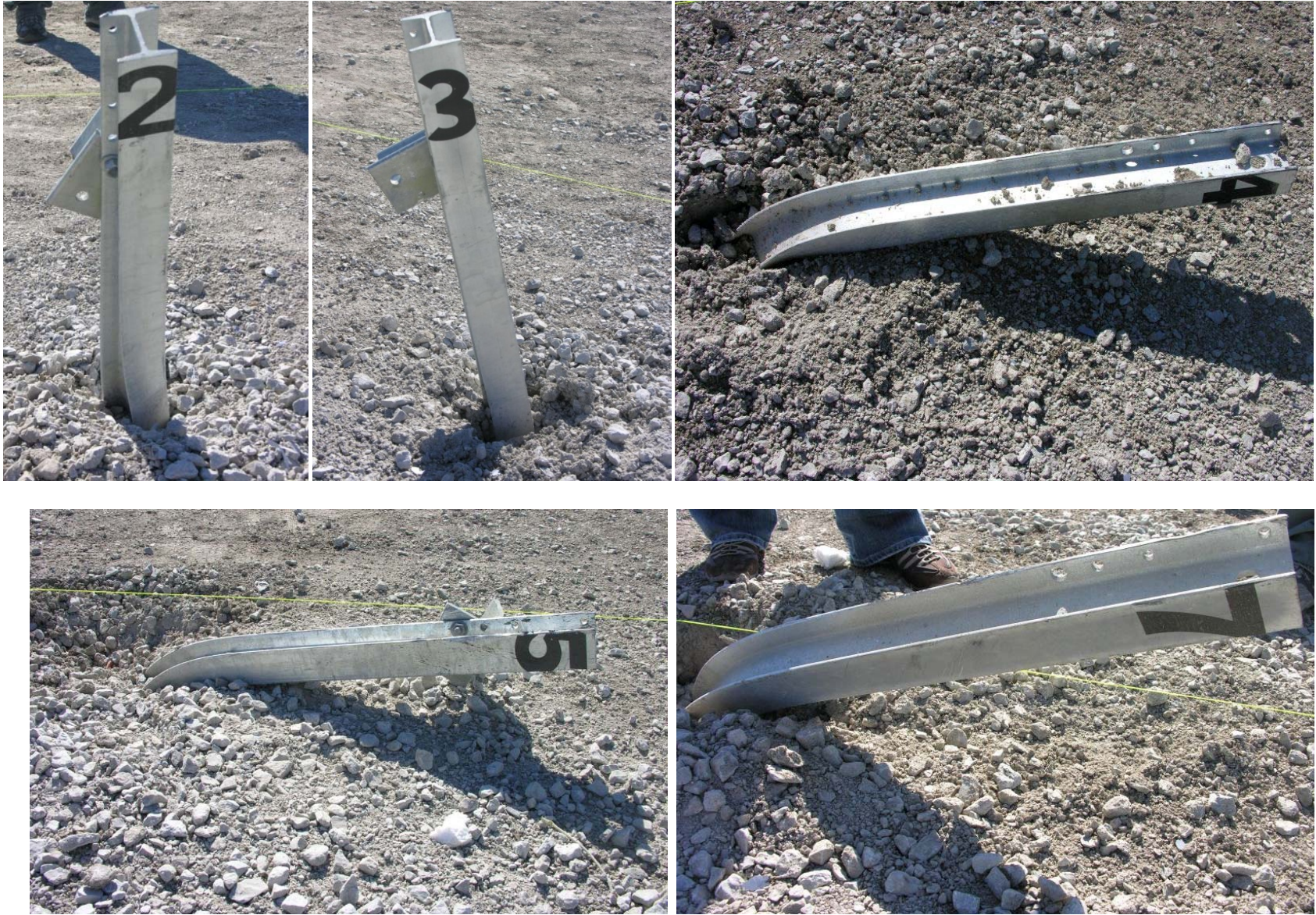
Figure 101. Post Damage – Back View, Test No. NYBBT-3
