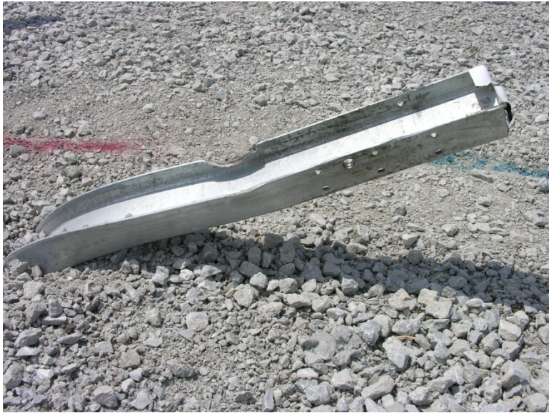
Figure 286. Post Nos. 5 and 6 Damage, Test No. NYBBT-9
