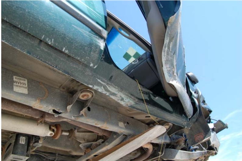
Figure 139. Undercarriage Damage, Test No. NYBBT-4
