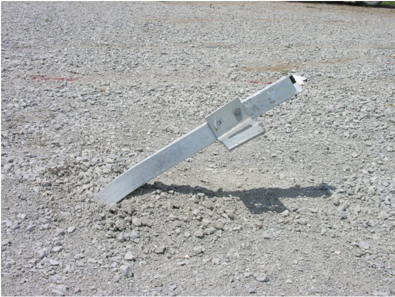
Figure 288. Post Nos. 9 and 10 Damage, Test No. NYBBT-9
