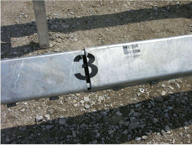
Figure 293. End Plate and Splice No. 1 Damage, Test No. NYBBT-9
