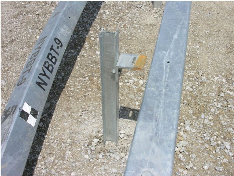
Figure 292. Post Nos. 19 through 22 Damage, Test No. NYBBT-9
