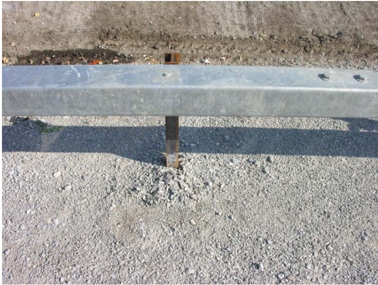
Figure 222. Post Nos. 17 and 18 Damage, Test No. NYBBT-7
