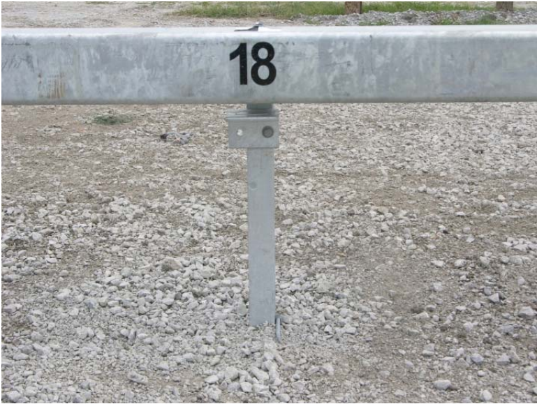
Figure 165. Post Nos. 17 and 18 Damage, Test No. NYBBT-5
