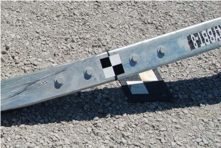
Figure 264. End Plate and Splice No. 1 Damage, Test No. NYBBT-8
