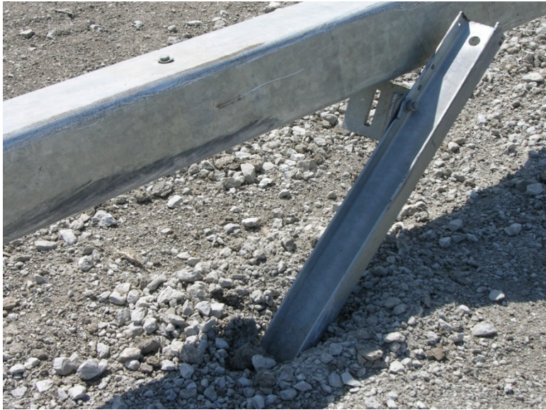
Figure 133. Post Nos. 17 and 18 Damage, Test No. NYBBT-4
