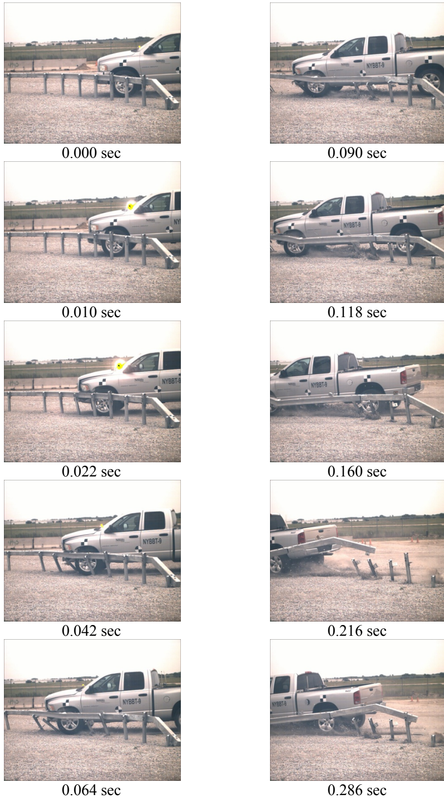
Figure 272. Additional Sequential Photographs, Test No. NYBBT-9
