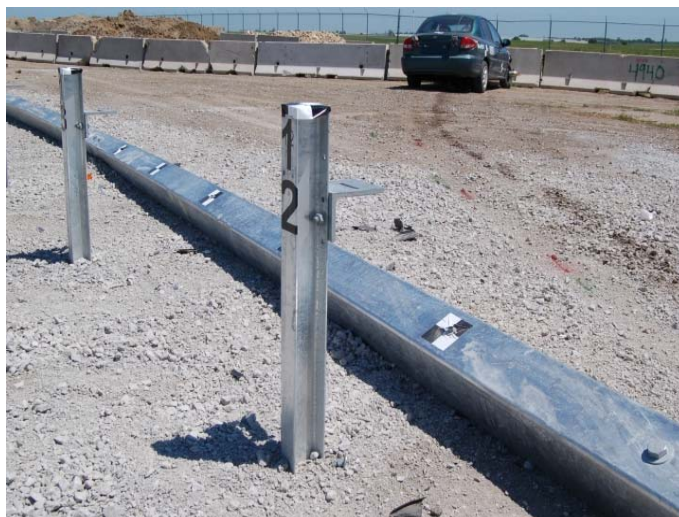
Figure 260. Post Nos. 11 and 12 Damage, Test No. NYBBT-8
