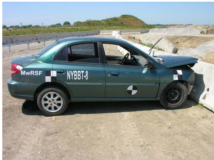
Figure 268. Vehicle Damage, Test No. NYBBT-8
