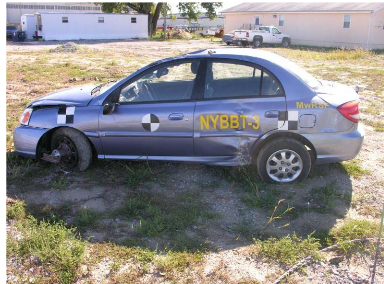
Figure 104. Vehicle Damage, Test No. NYBBT-3 (The roof, windshield, and left side damage was due to the secondary impact with the setup from another system.)
