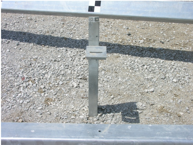
Figure 291. Post Nos. 15 through 18 Damage, Test No. NYBBT-9
