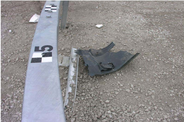
Figure 90. System Damage, Test No. NYBBT-2
