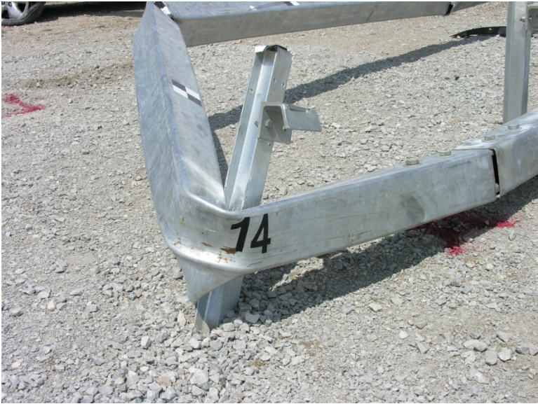
Figure 290. Post Nos. 13 and 14 Damage, Test No. NYBBT-9
