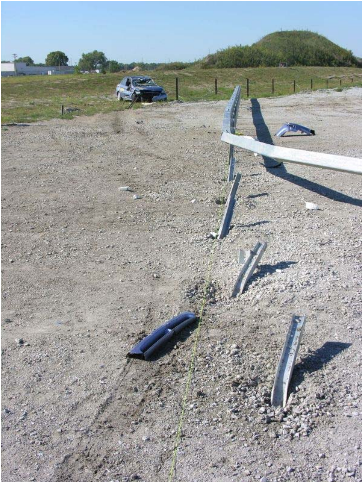
Figure 99. Vehicle Final Position and Trajectory Marks, Test NYBBT-3
