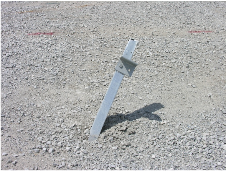
Figure 289. Post Nos. 11 and 12 Damage, Test No. NYBBT-9
