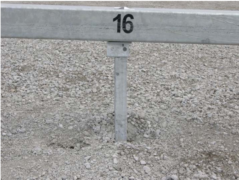
Figure 164. Post Nos. 15 and 16 Damage, Test No. NYBBT-5
