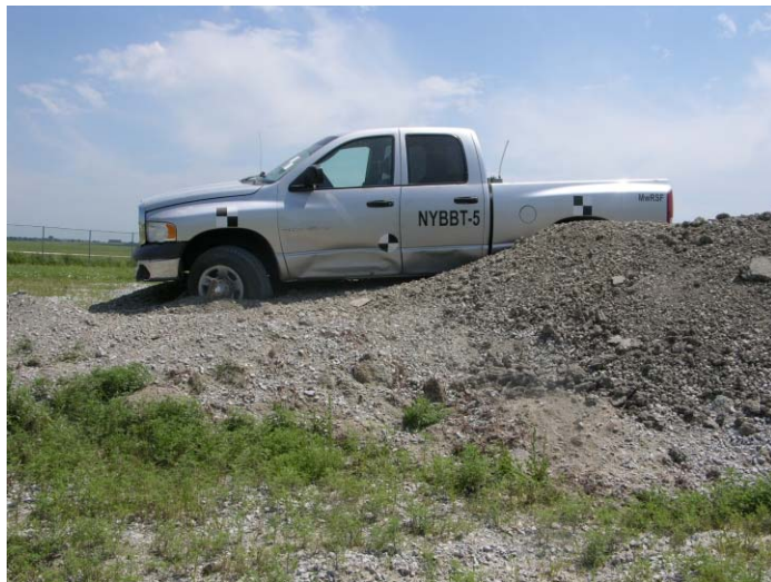
Figure 166. Vehicle Damage, Test No. NYBBT-5
