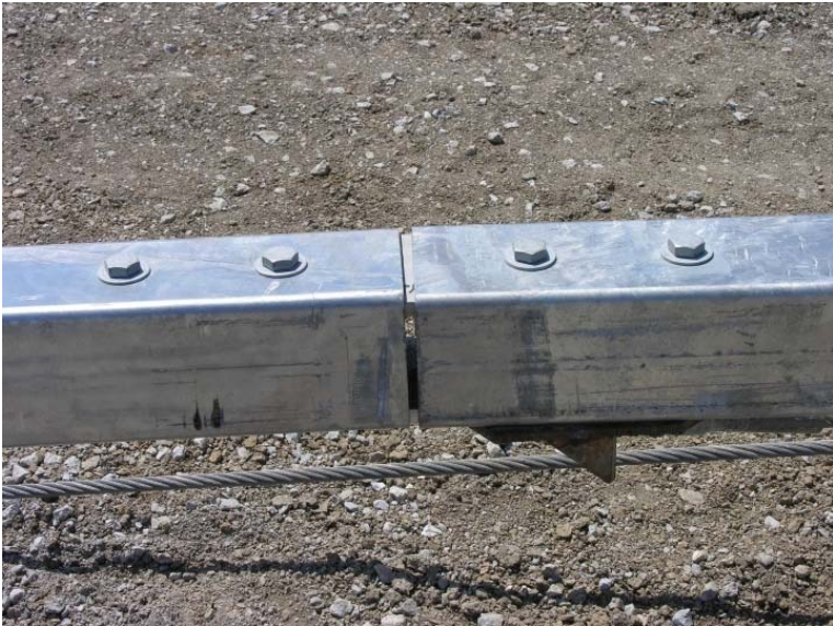
Figure 267. Splice Nos. 6 and 7 Damage, Test No. NYBBT-8
