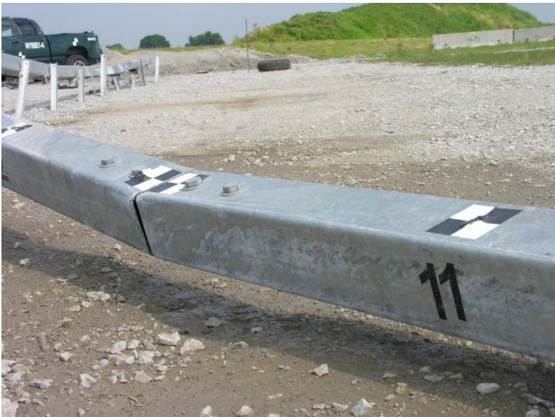
Figure 124. Barrier Damage, Test No. NYBBT-4
