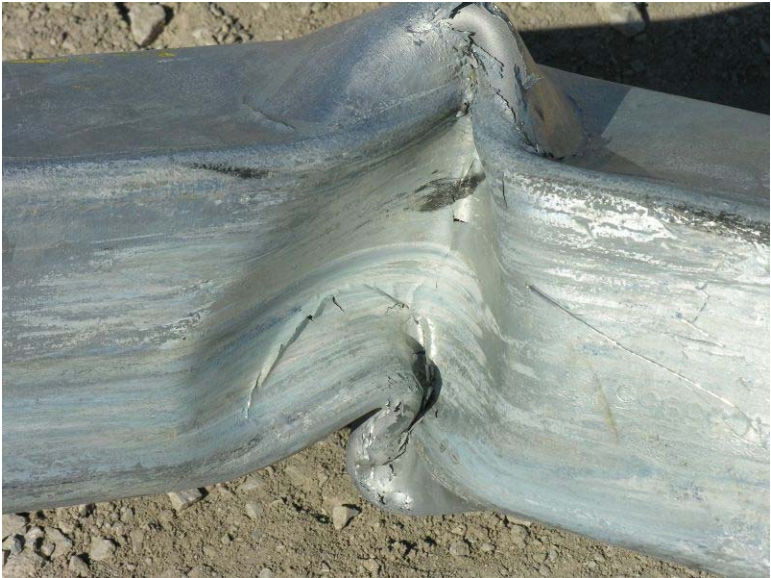
Figure 103. Rail Damage, Test No. NYBBT-3
