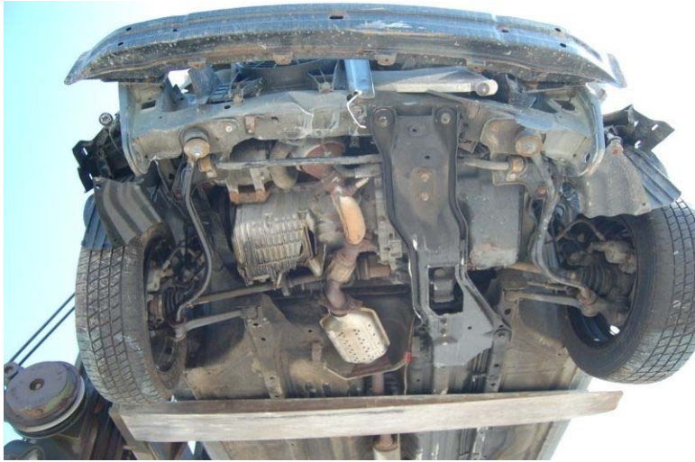
Figure 65. Undercarriage Damage, Test No. NYBBT-1
