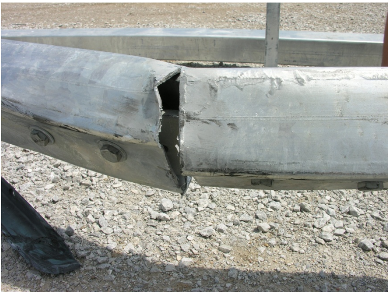
Figure 294. Splice Nos. 2 and 3 Damage, Test No. NYBBT-9
