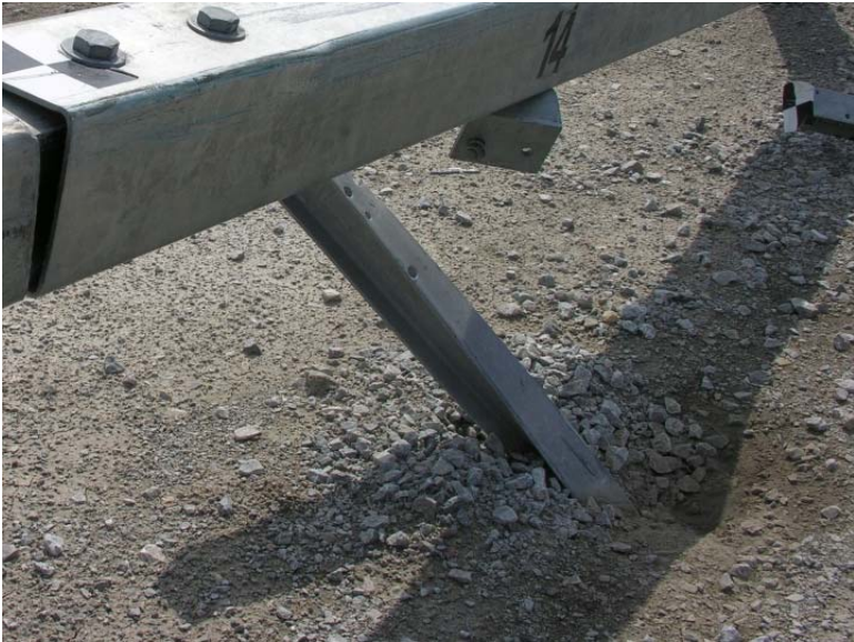
Figure 131. Post Nos. 13 and 14 Damage, Test No. NYBBT-4
