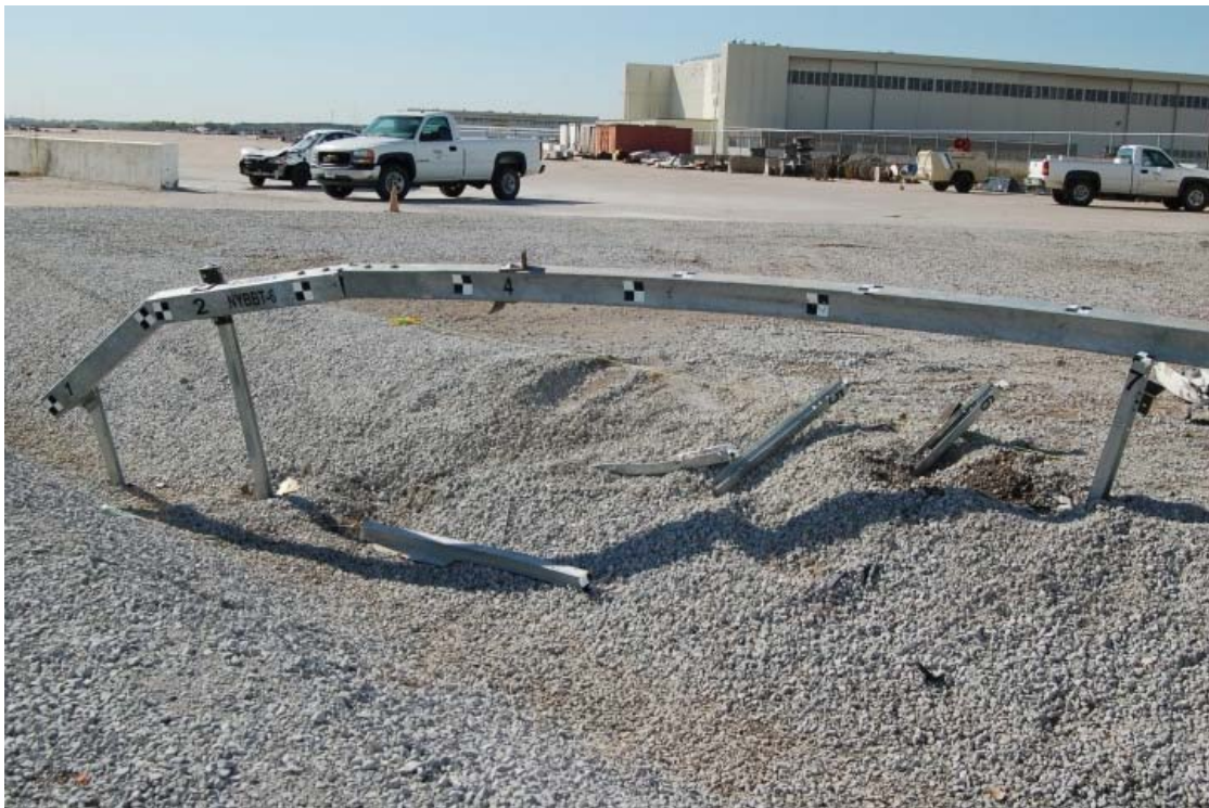
Figure 197. Barrier Damage, Test No. NYBBT-6
