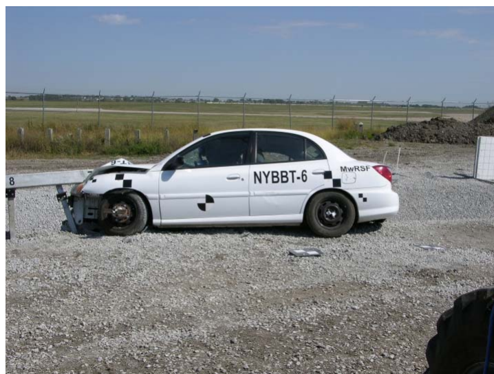
Figure 199. Vehicle Damage, Test No. NYBBT-6
