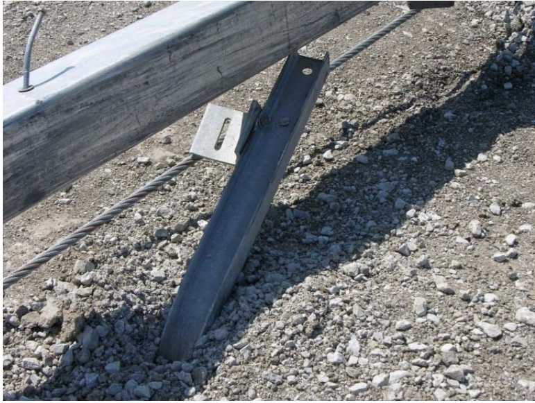
Figure 134. Post Nos. 19 and 20 Damage, Test No. NYBBT-4
