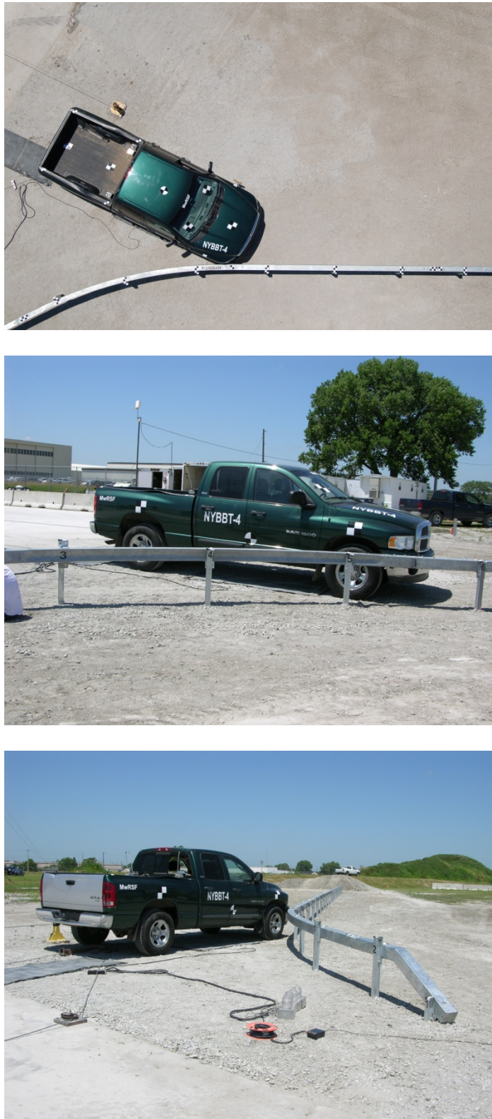
Figure 120. Impact Location, Test No. NYBBT-4
