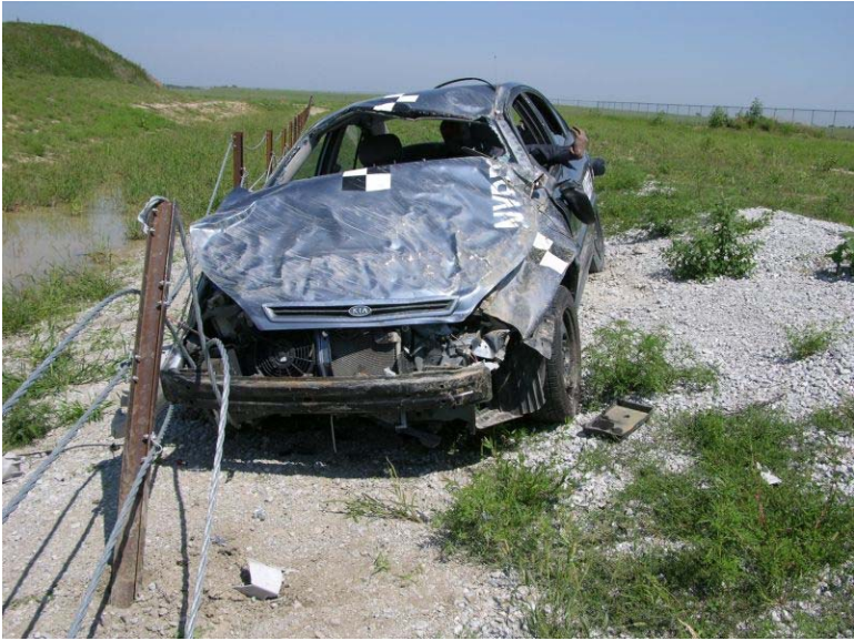
Figure 64. Vehicle Damage, Test No. NYBBT-1
