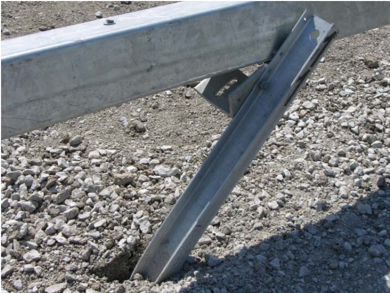
Figure 132. Post Nos. 15 and 16 Damage, Test No. NYBBT-4
