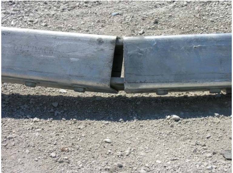
Figure 265. Splice Nos. 2 and 3 Damage, Test No. NYBBT-8
