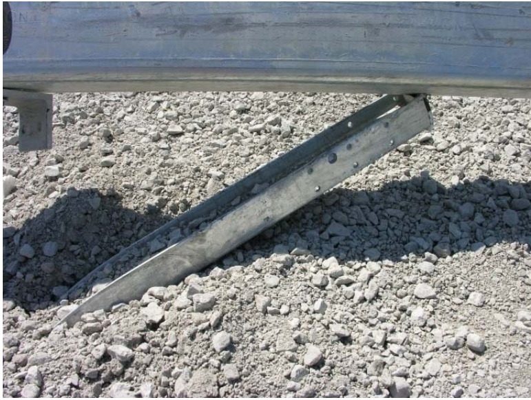
Figure 259. Post Nos. 9 and 10 Damage, Test No. NYBBT-8
