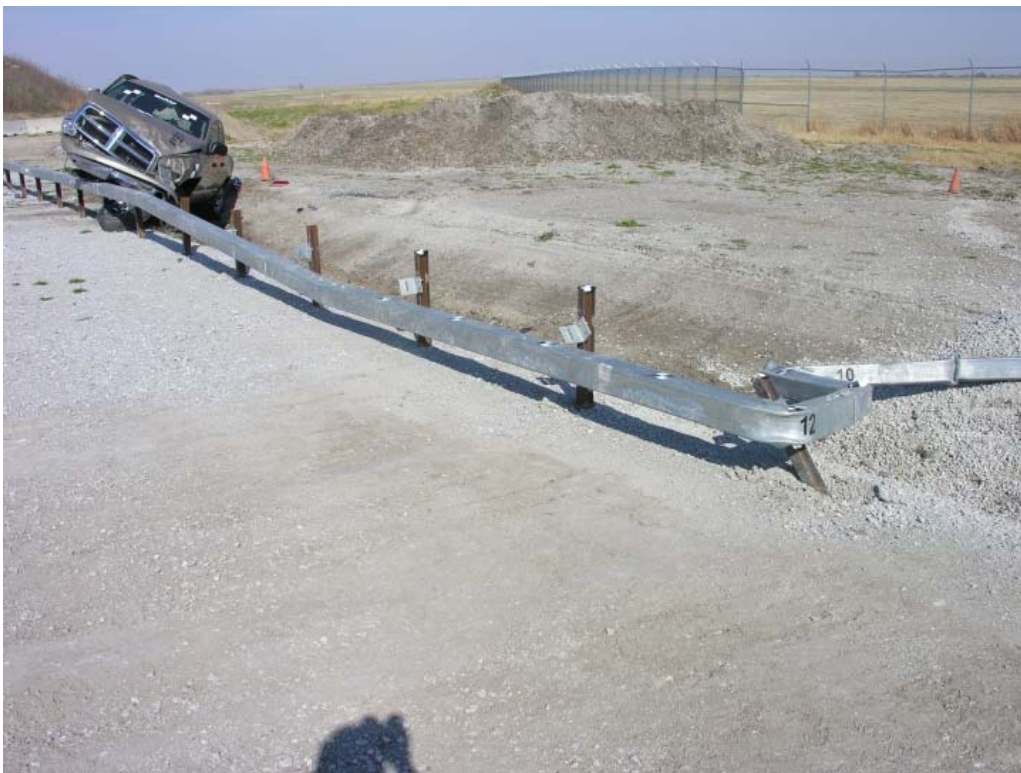
Figure 209. Barrier Damage, Test No. NYBBT-7
