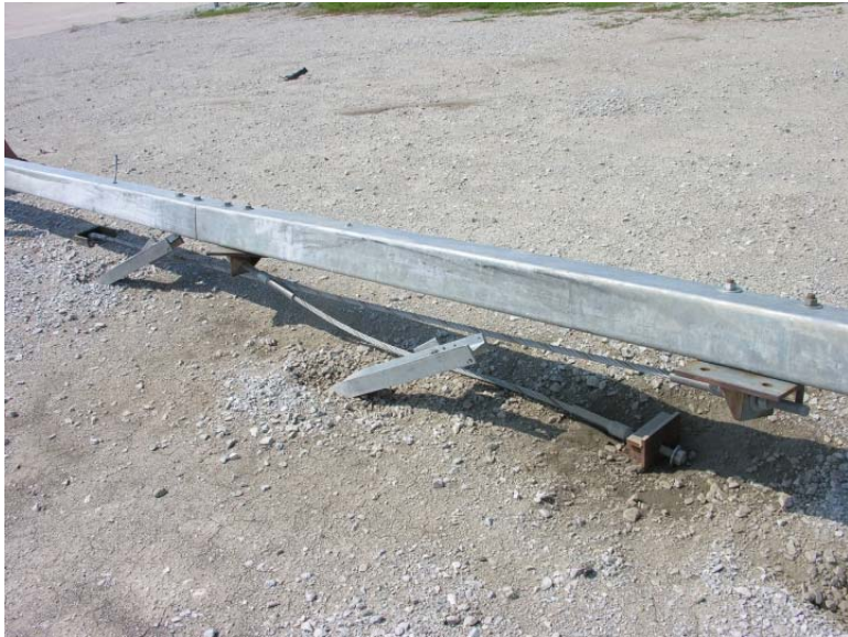
Figure 136. Post No. 23 and End Anchorage Damage, Test No. NYBBT-4
