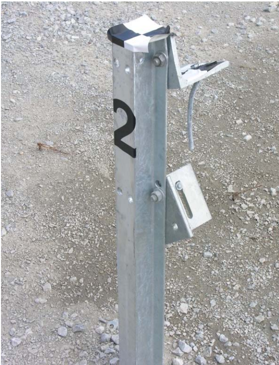
Figure 125. Post Nos. 1 and 2 Damage, Test No. NYBBT-4
