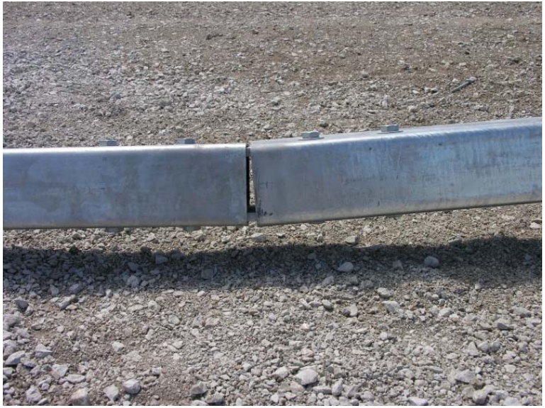
Figure 266. Splice Nos. 4 and 5 Damage, Test No. NYBBT-8
