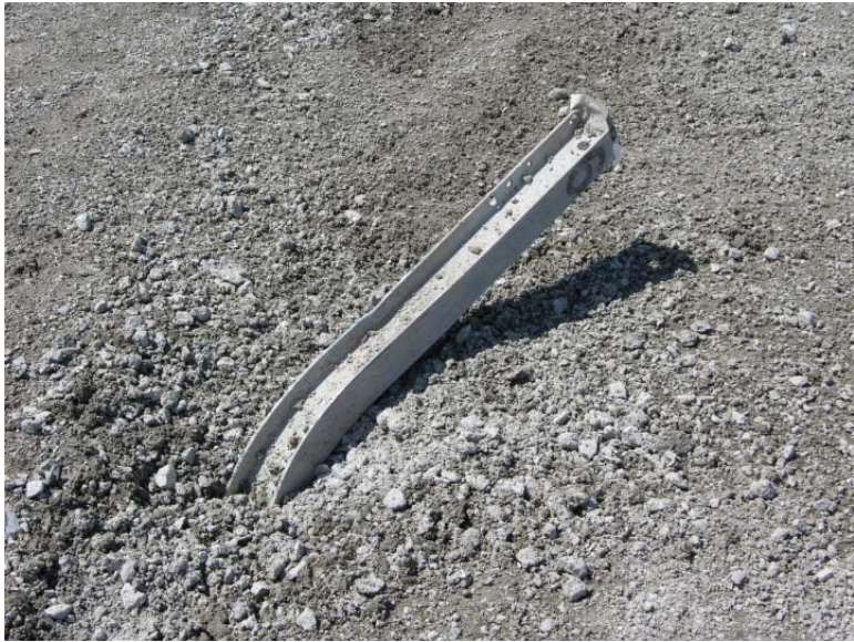
Figure 127. Post Nos. 5 and 6 Damage, Test No. NYBBT-4
