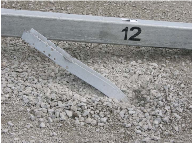
Figure 162. Post Nos. 11 and 12 Damage, Test No. NYBBT-5
