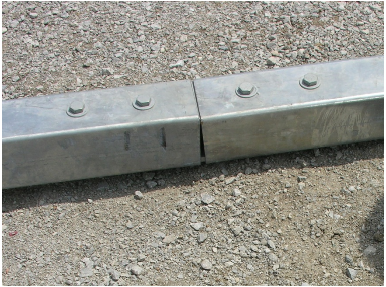
Figure 295. Splice Nos. 4 and 5 Damage, Test No. NYBBT-9
