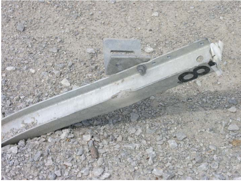
Figure 128. Post Nos. 7 and 8 Damage, Test No. NYBBT-4
