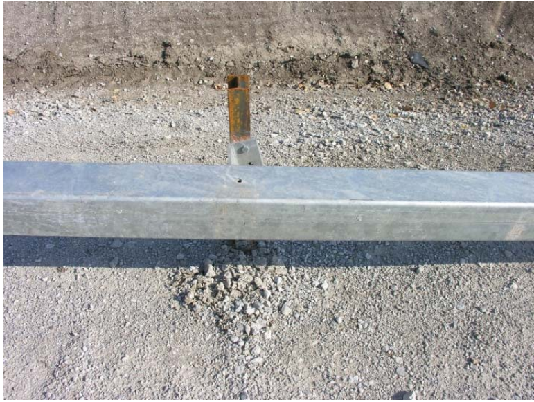
Figure 221. Post Nos. 15 and 16 Damage, Test No. NYBBT-7
