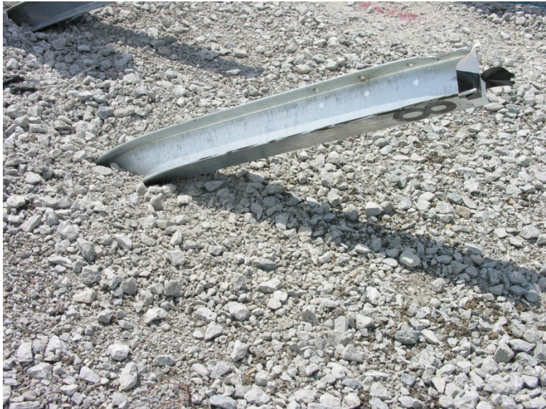
Figure 287. Post Nos. 7 and 8 Damage, Test No. NYBBT-9
