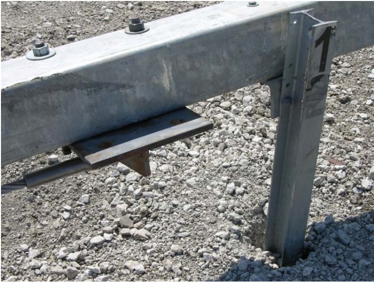
Figure 135. Post Nos. 21 and 22 Damage, Test No. NYBBT-4
