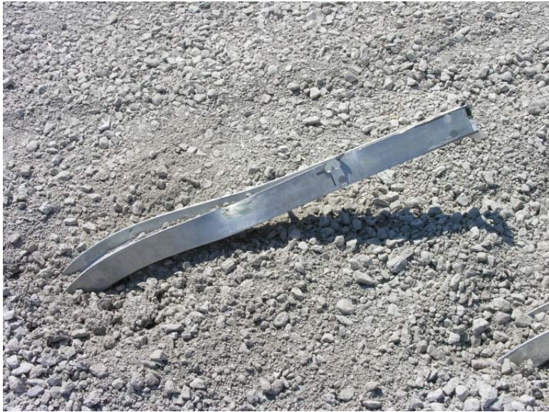
Figure 256. Post Nos. 3 and 4 Damage, Test No. NYBBT-8
