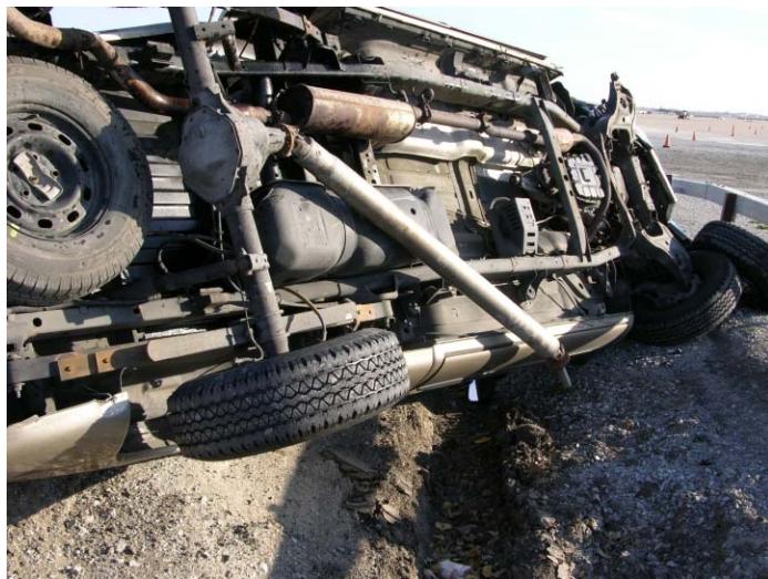
Figure 223. Vehicle Damage, Test No. NYBBT-7
