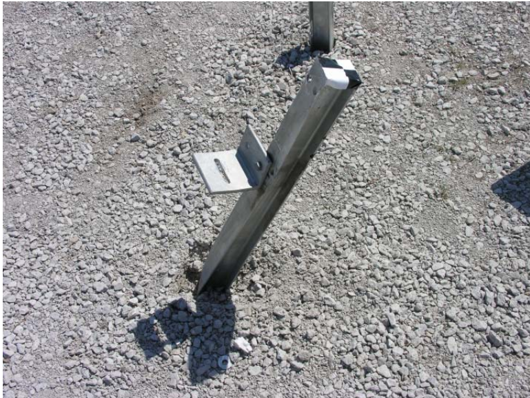
Figure 255. Post Nos. 1 and 2 Damage, Test No. NYBBT-8
