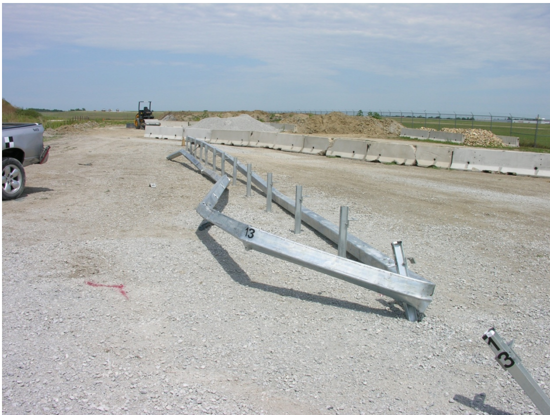
Figure 280. Barrier Damage, Test No. NYBBT-9
