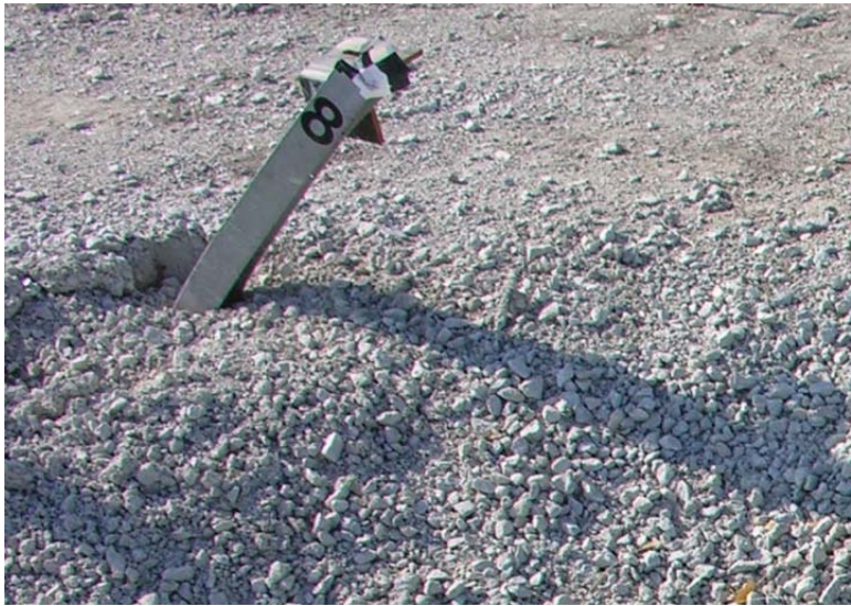
Figure 217. Post Nos. 7 and 8 Damage, Test No. NYBBT-7
