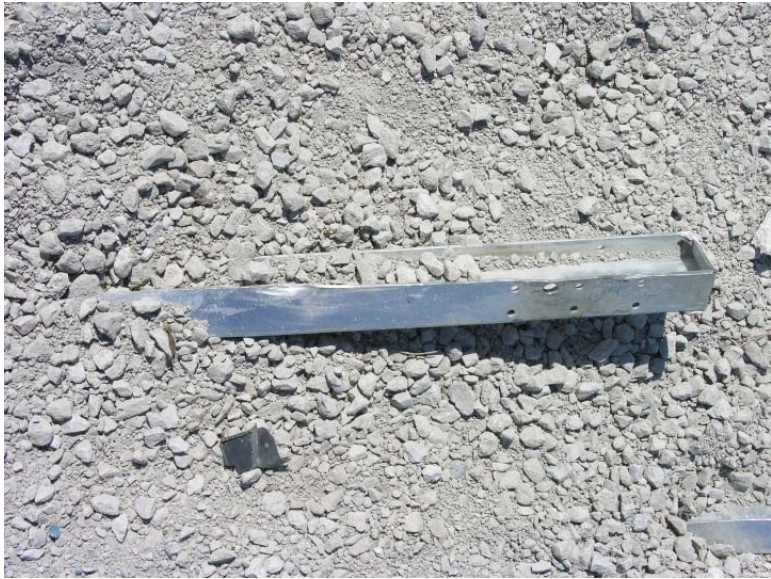
Figure 257. Post Nos. 5 and 6 Damage, Test No. NYBBT-8
