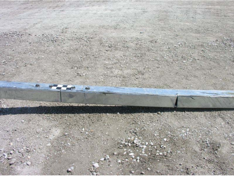
Figure 62. System Damage, Test No. NYBBT-1
