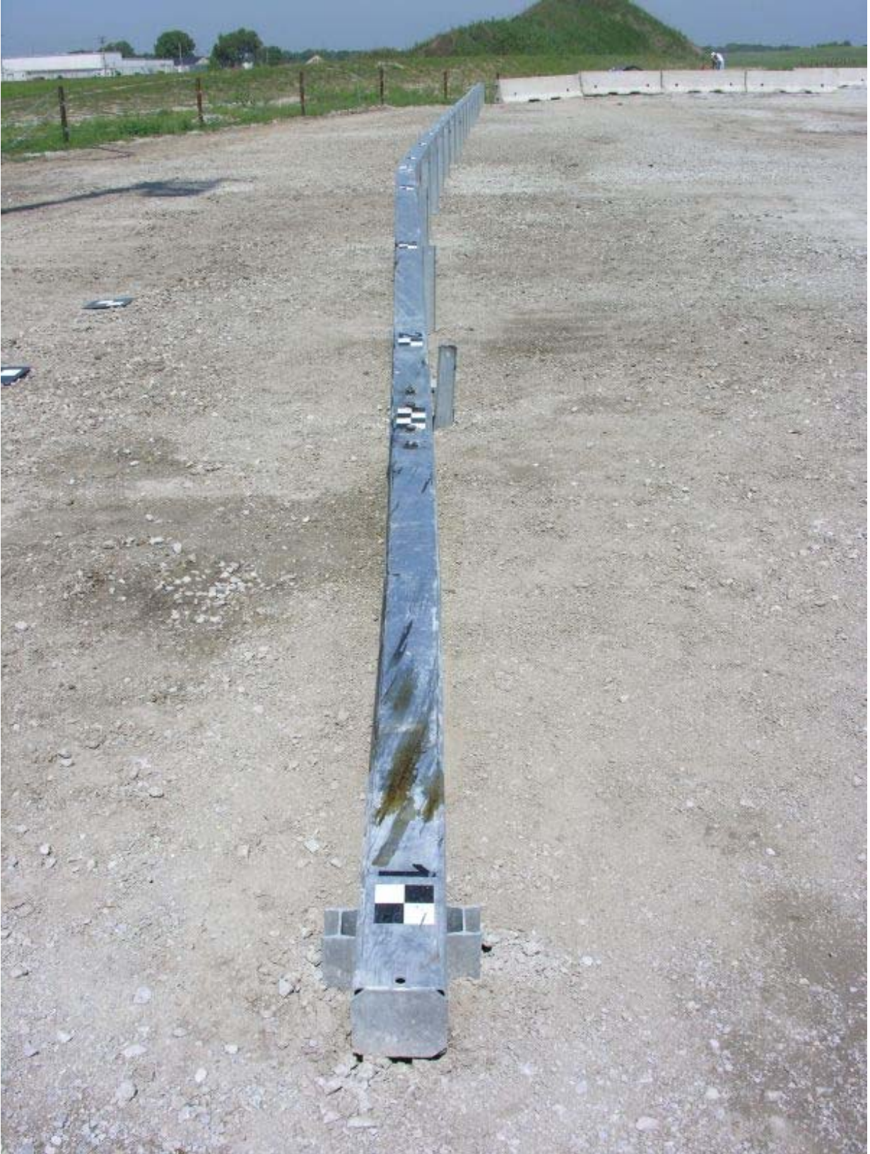
Figure 61. System Damage, Test No. NYBBT-1
