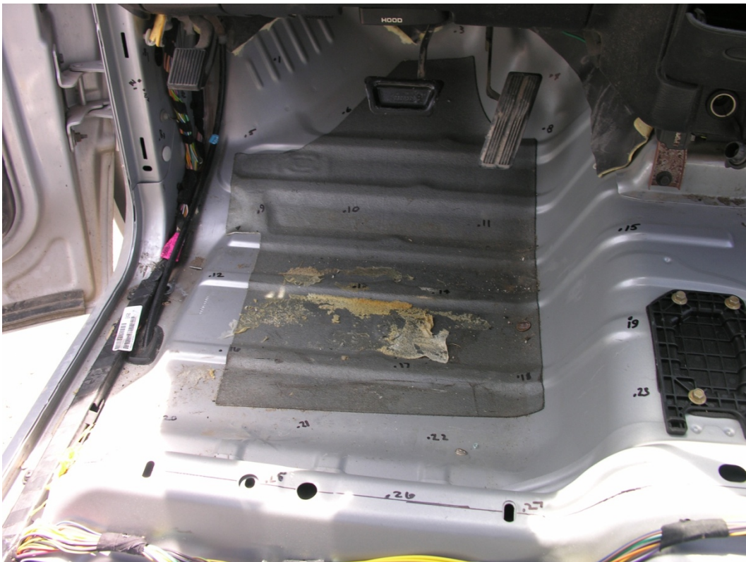
Figure 299. Occupant Compartment Deformation, Test No. NYBBT-9
