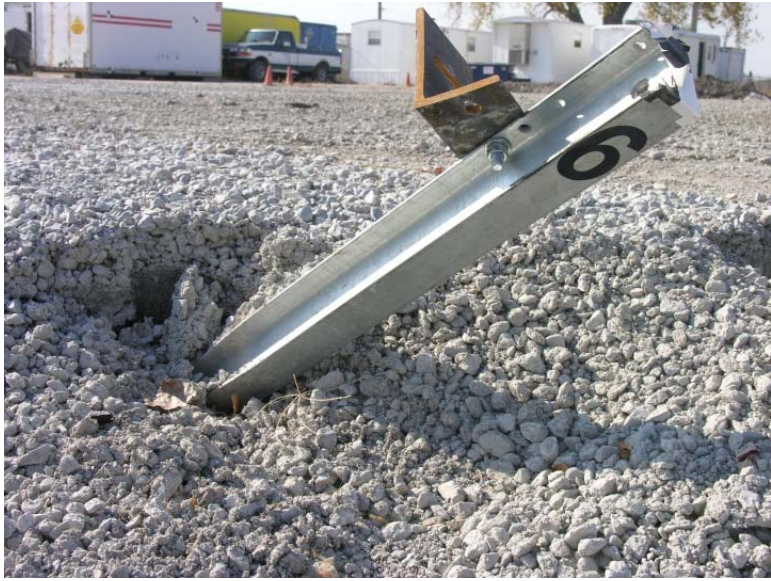
Figure 216. Post Nos. 5 and 6 Damage, Test No. NYBBT-7
