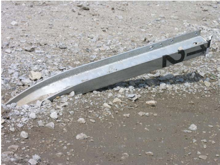
Figure 130. Post Nos. 11 and 12 Damage, Test No. NYBBT-4
