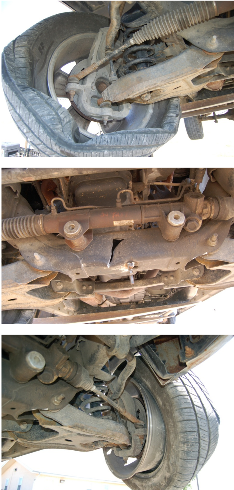
Figure 298. Vehicle Undercarriage Damage, Test No. NYBBT-9
