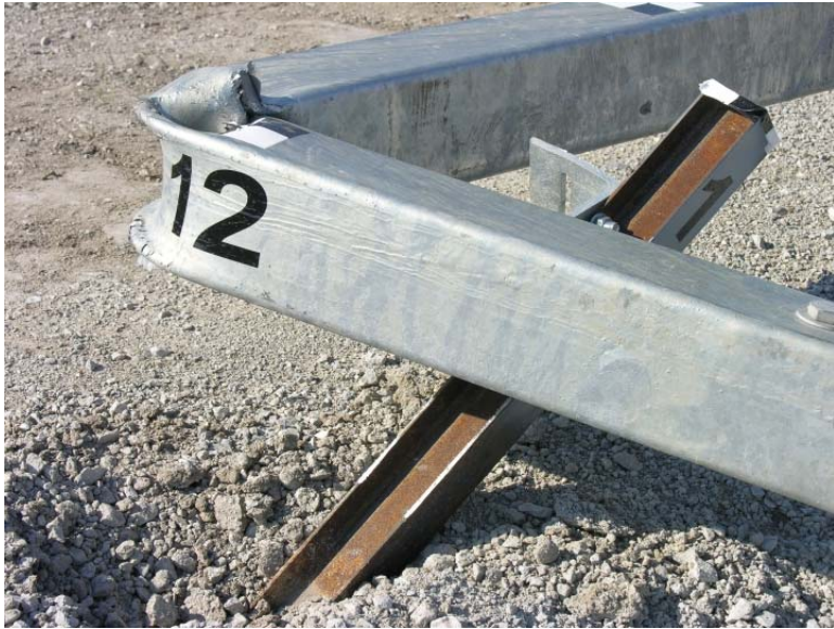
Figure 219. Post Nos. 11 and 12 Damage, Test No. NYBBT-7
