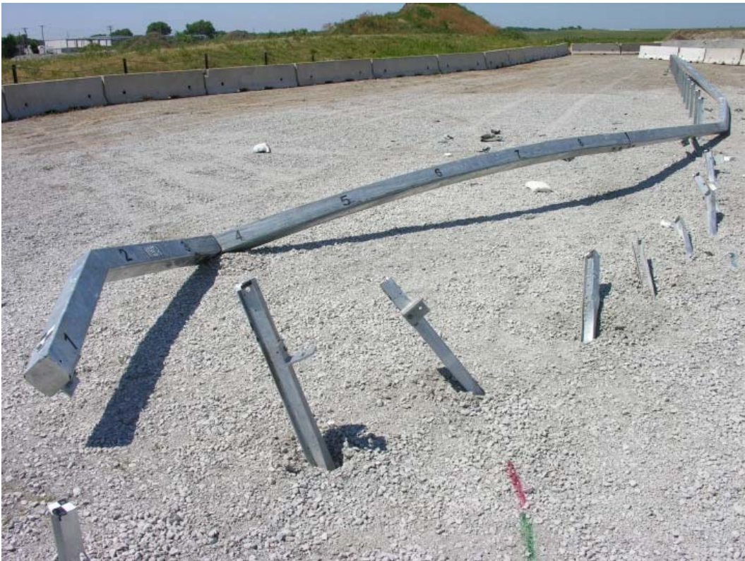
Figure 252. Barrier Damage, Test No. NYBBT-8
