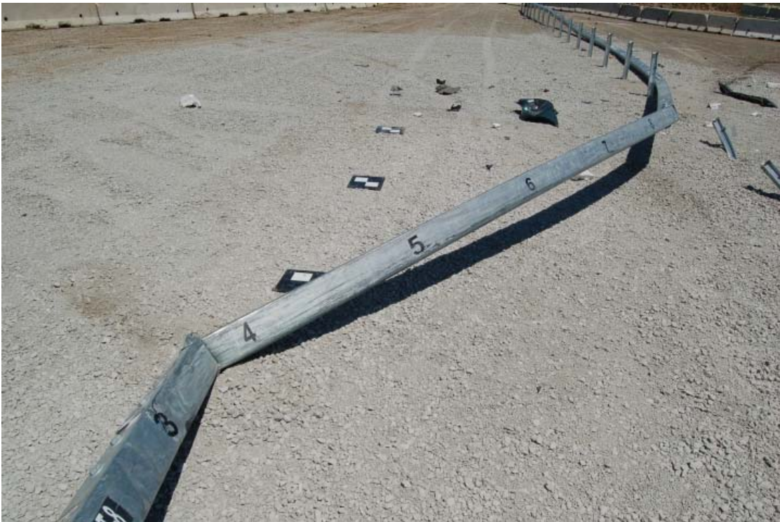
Figure 253. Barrier Damage, Test No. NYBBT-8
