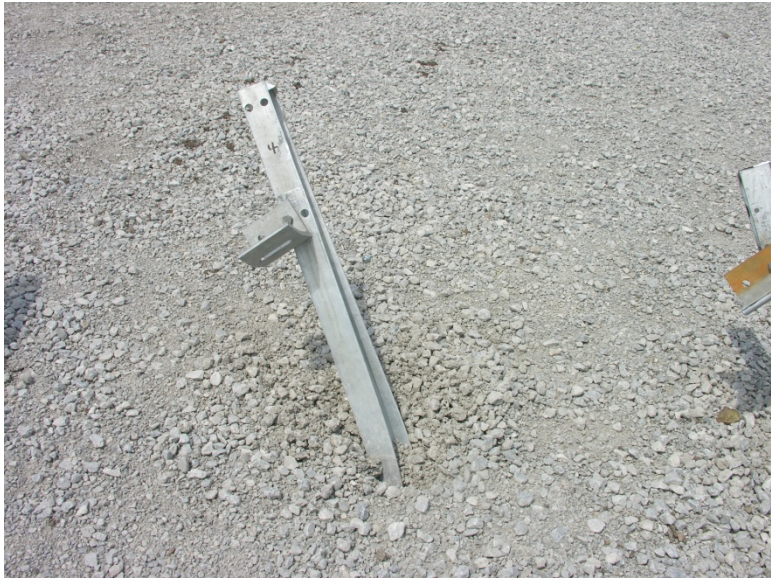
Figure 285. Post Nos. 3 and 4 Damage, Test No. NYBBT-9
