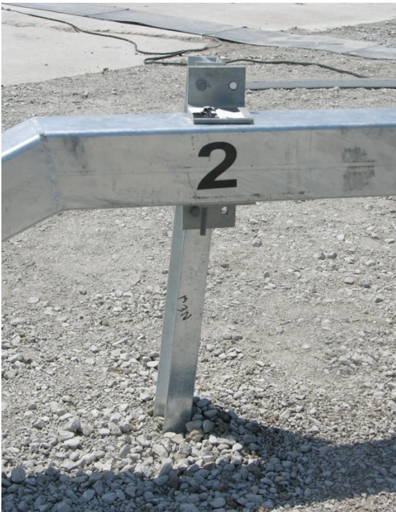
Figure 157. Post Nos. 1 and 2 Damage, Test No. NYBBT-5
