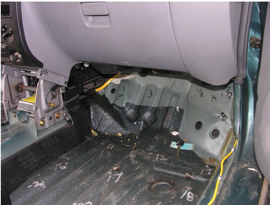
Figure 93. Occupant Compartment Damage, Test No. NYBBT-2
