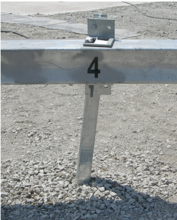
Figure 158. Post Nos. 3 and 4 Damage, Test No. NYBBT-5
