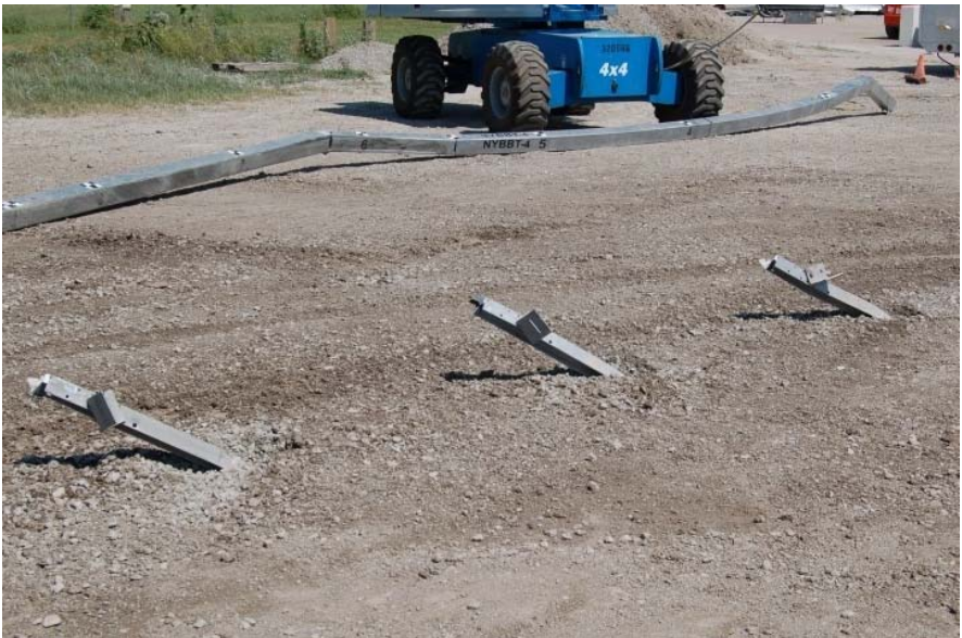
Figure 123. Barrier Damage, Test No. NYBBT-4
