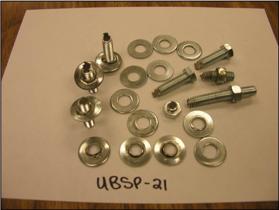
Figure 134. Additional Images of Bolt and Washer Damage of UBSP-21
