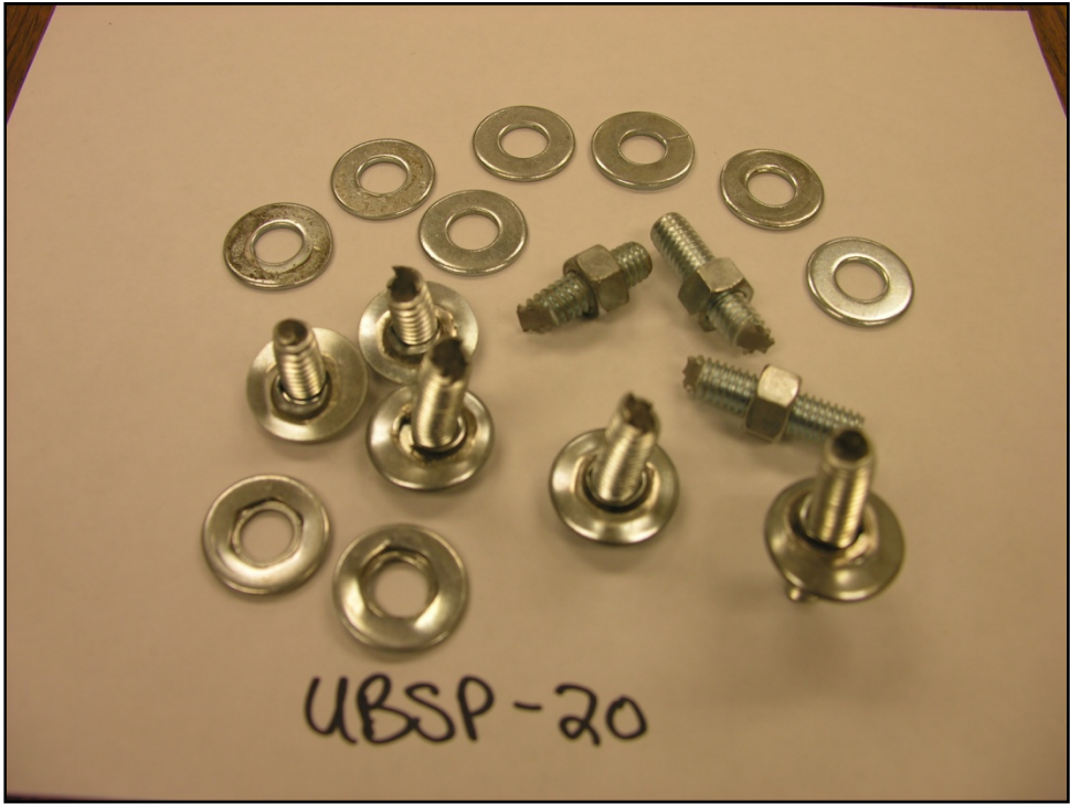
Figure 129. Additional Images of Bolt and Washer Damage of UBSP-20
