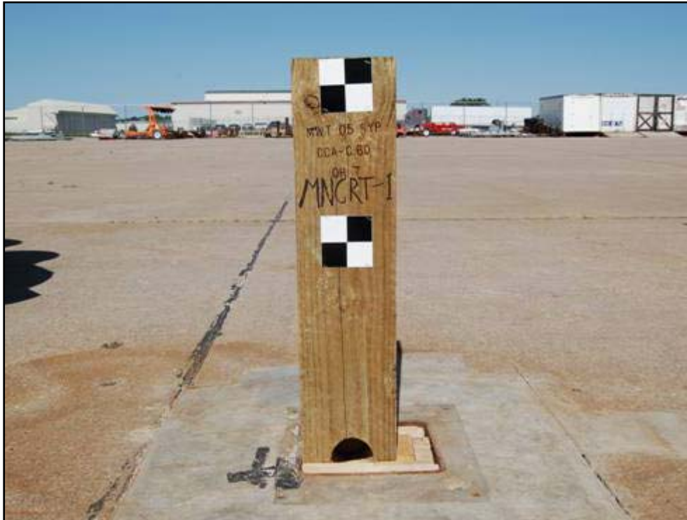
Figure 1. CRT Wood Post in Rigid Sleeve
