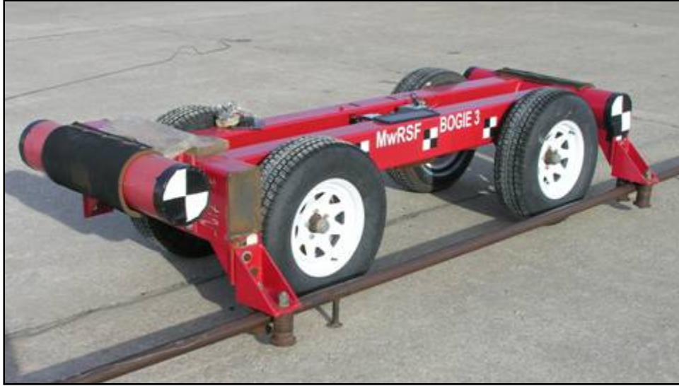
Figure 35. Rigid Frame Bogie on Guidance Track
