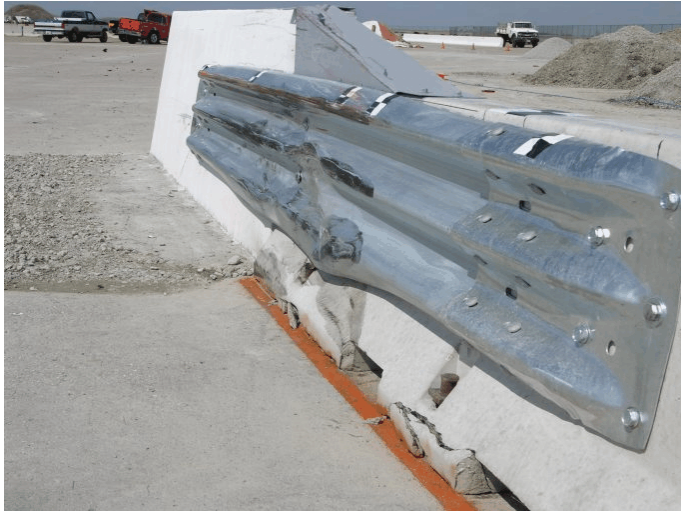
Figure 45. System Damage, Test No. TCBT-1
