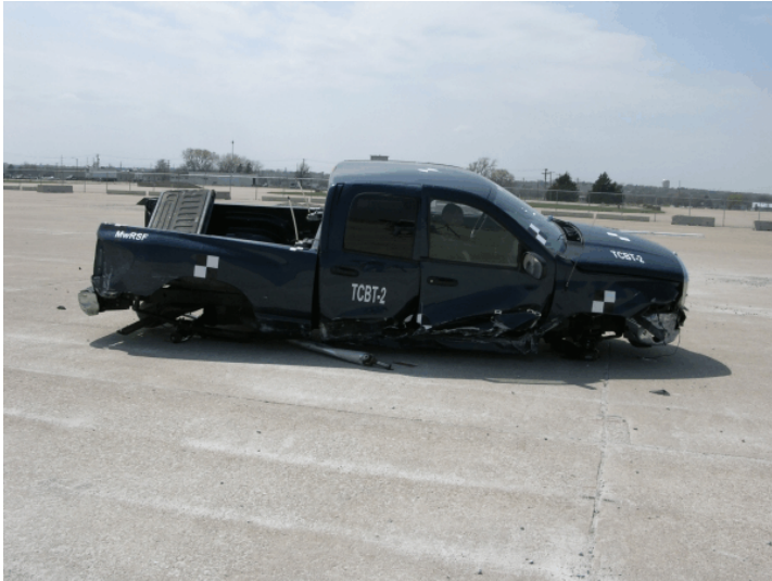
Figure 65. Vehicle Damage, Test No. TCBT-2
