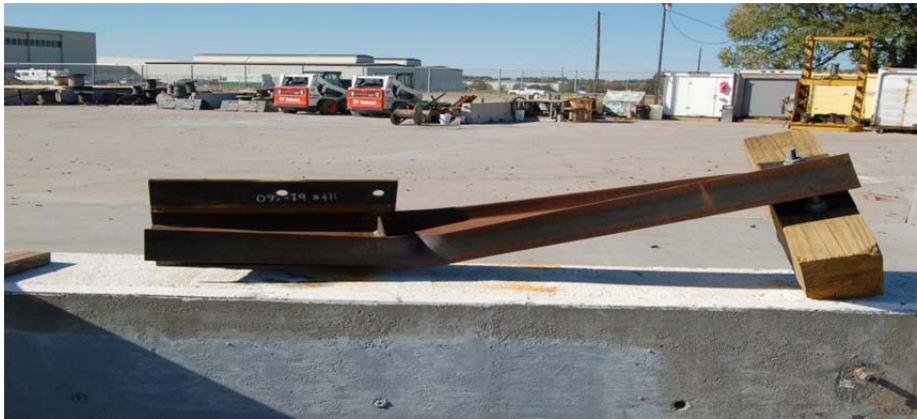
Figure 51. Post Assembly Damage, Test No. WAGTMP-4
