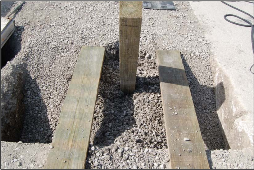
Post After Impact – Soil Displacement
