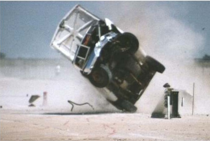
Figure 1. Example of Vehicle Pocketing in Rail, Test No. MWT-2 [1]
