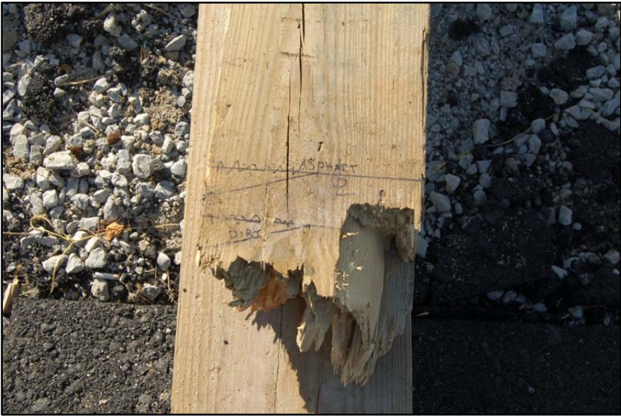
Post After Impact – Fracture surface
