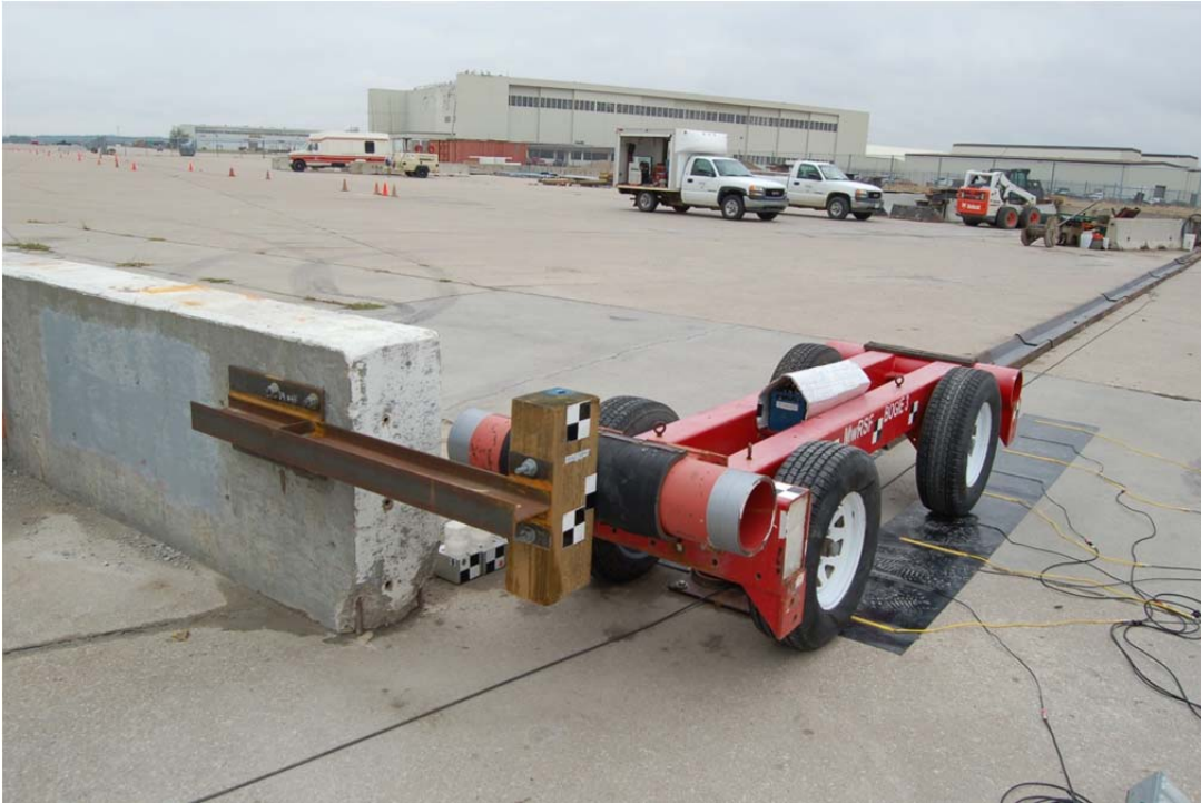
Figure 33. Rigid Frame Bogie on Guidance Track
