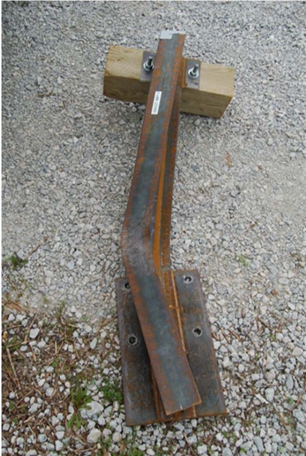
Figure 44. Post Assembly Damage, Test No. WAGTMP-1
