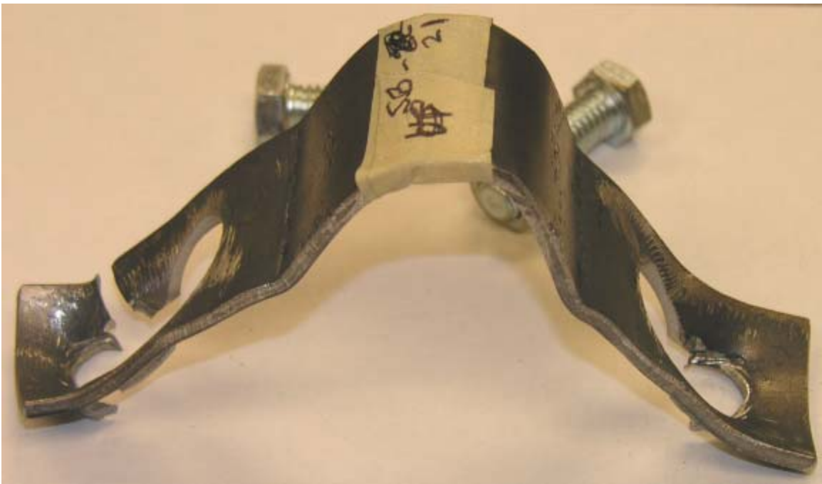
Figure B-4. Flat Keyway Brackets – Test No. SB-21: Lateral Loading
