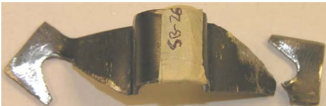
Figure B-6. Angled Slot Brackets – Test Nos. SB-25, SB-26: Lateral Loading
