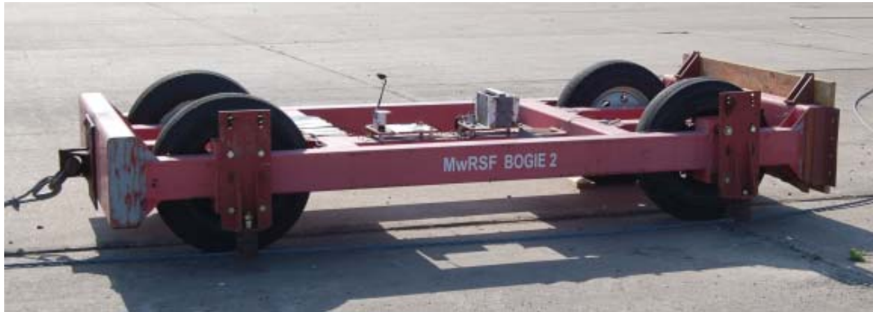
Figure 102. Bogie Used in Dynamic Testing
