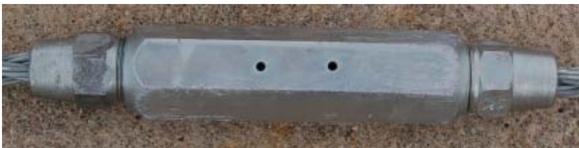
Figure 114. Cable Splice, Test No. 4CTB-6
