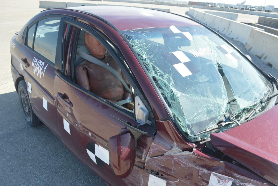
Figure 43. Vehicle Damage, Test No. H34BR-1
