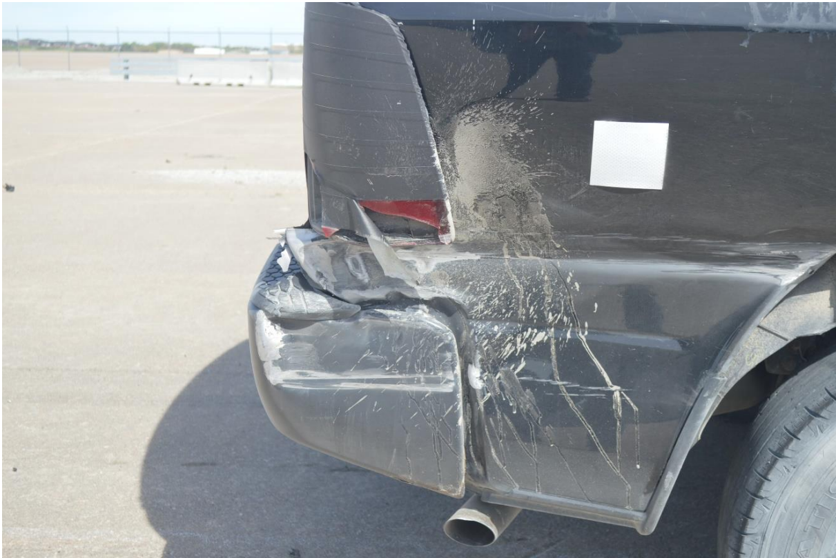
Figure 61. Vehicle Damage, Test No. H34BR-2
