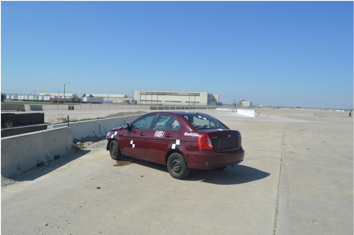
Figure 34. Vehicle Final Position and Trajectory Marks, Test No. H34BR-1
