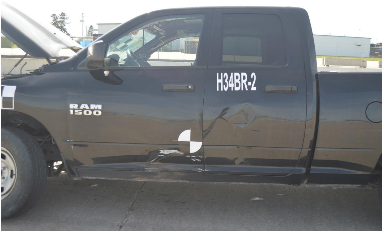
Figure 62. Vehicle Damage, Test No. H34BR-2
