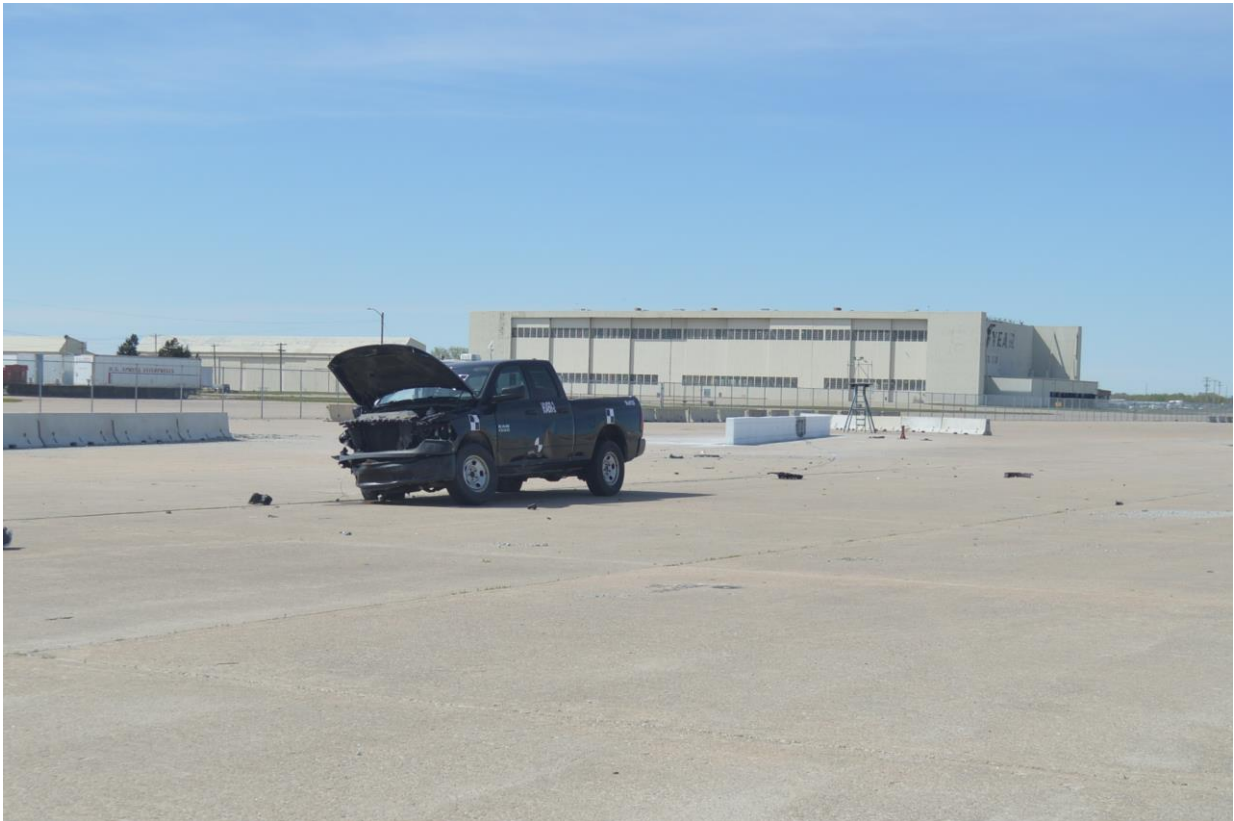
Figure 54. Vehicle Final Position & Trajectory Marks, Test No. H34BR-2
