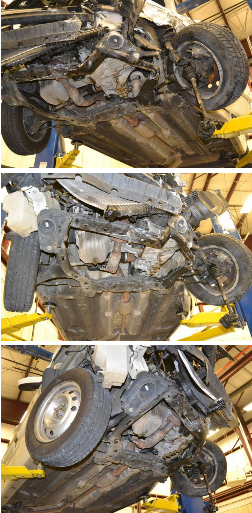
Figure 68. Undercarriage Damage, Test No. 34AGT-2
