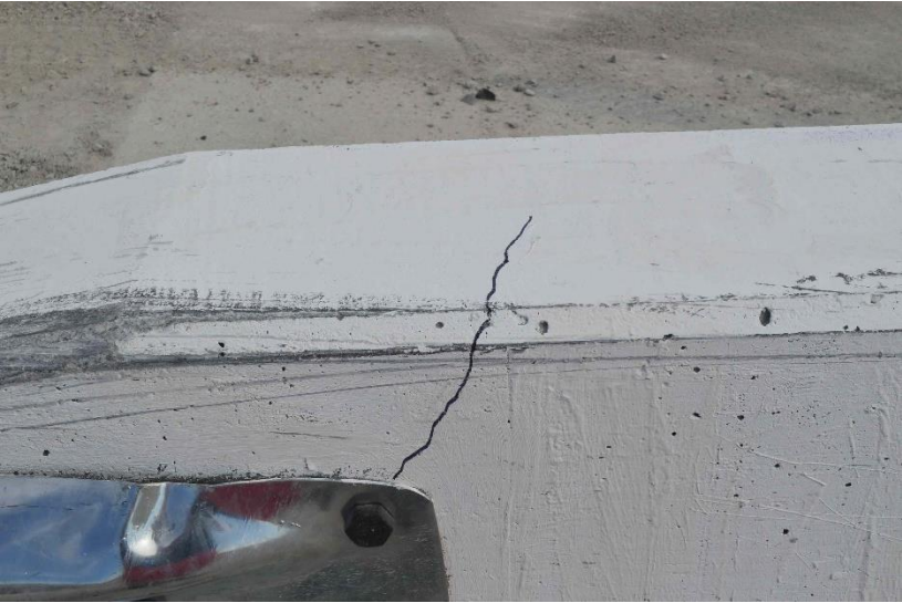
Figure 49. Buttress Damage, Test No. 34AGT-1
