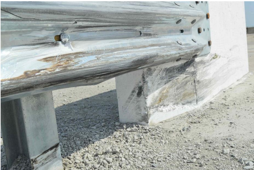
Figure 62. System Damage, Concrete Buttress, Test No. 34AGT-2
