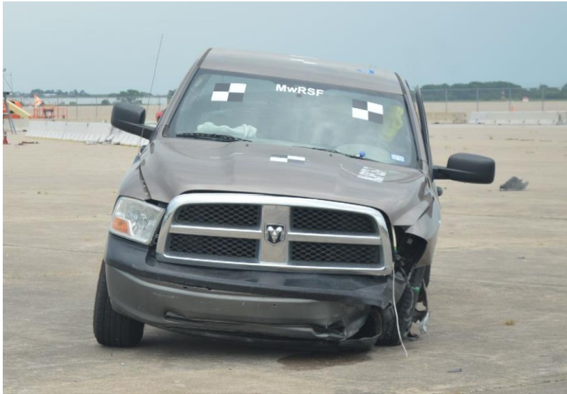
Figure 39. Vehicle Damage, Test No. NJPCB-7
