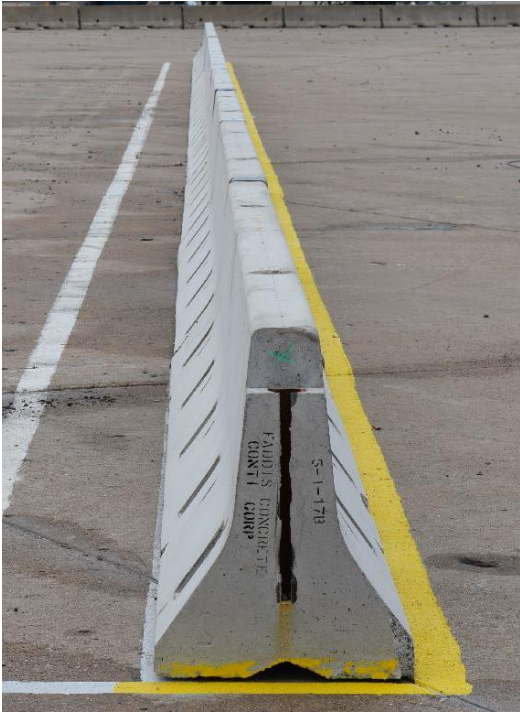
Figure 15. NJDOT PCB with Traffic-Side Pinned Configuration and Grouted Toes Test Installation, Test No. NJPCB-7
