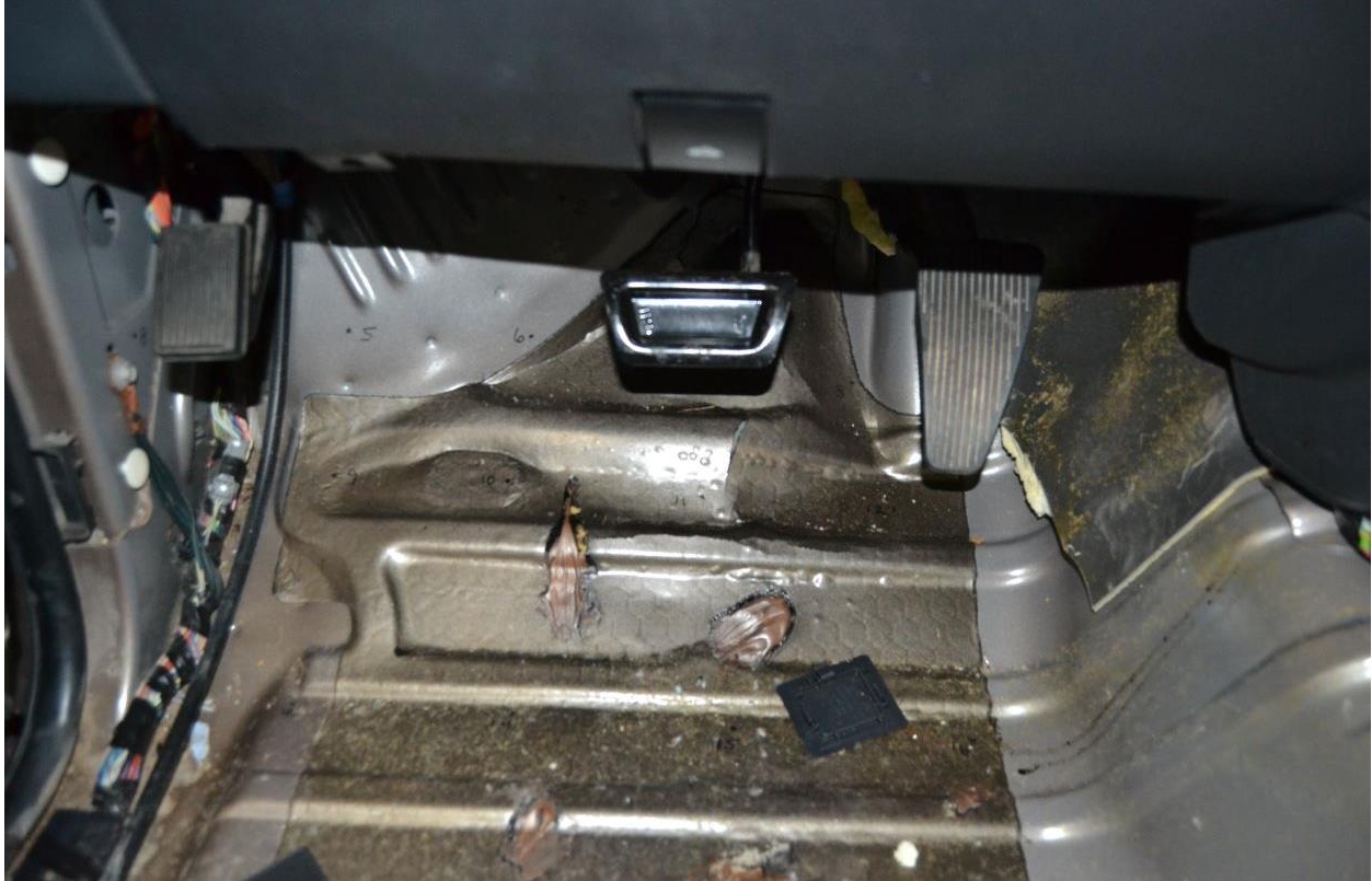
Figure 42. Occupant Compartment Deformation, Test No. NJPCB-7
