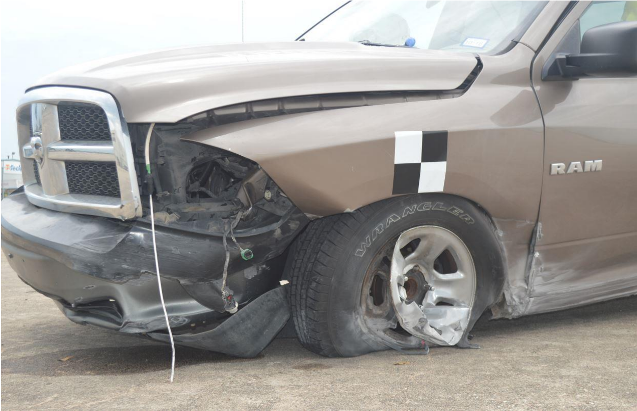
Figure 40. Vehicle Damage on Impact Side, Test No. NJPCB-7
