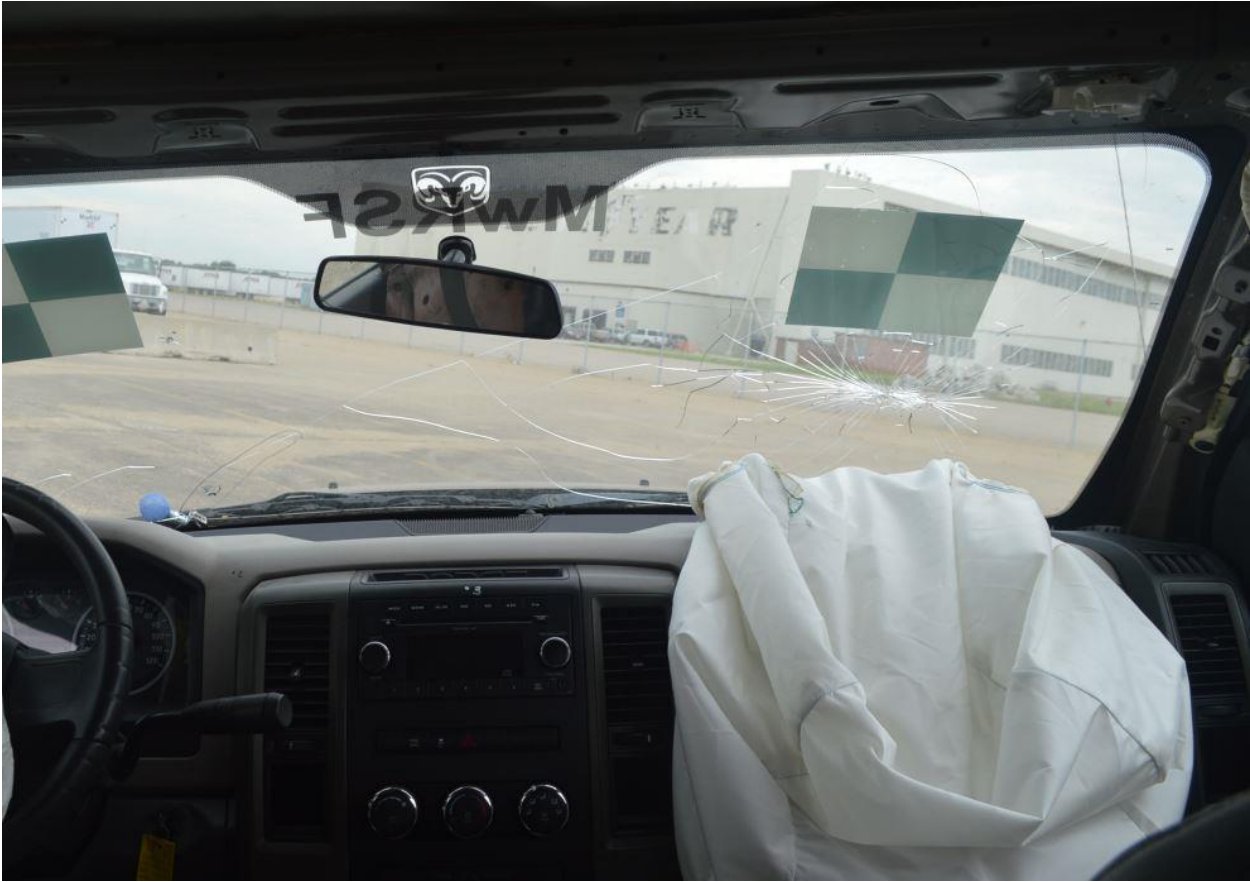
Figure 41. Vehicle Windshield Damage, Test No. NJPCB-7
