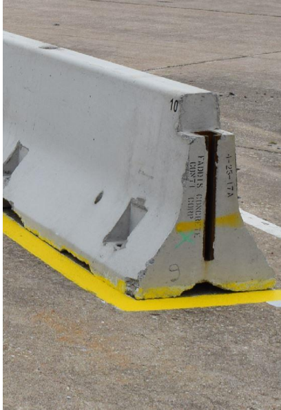
Figure 16. PCB Connection Key and Connection Socket, Test No. NJPCB-7
