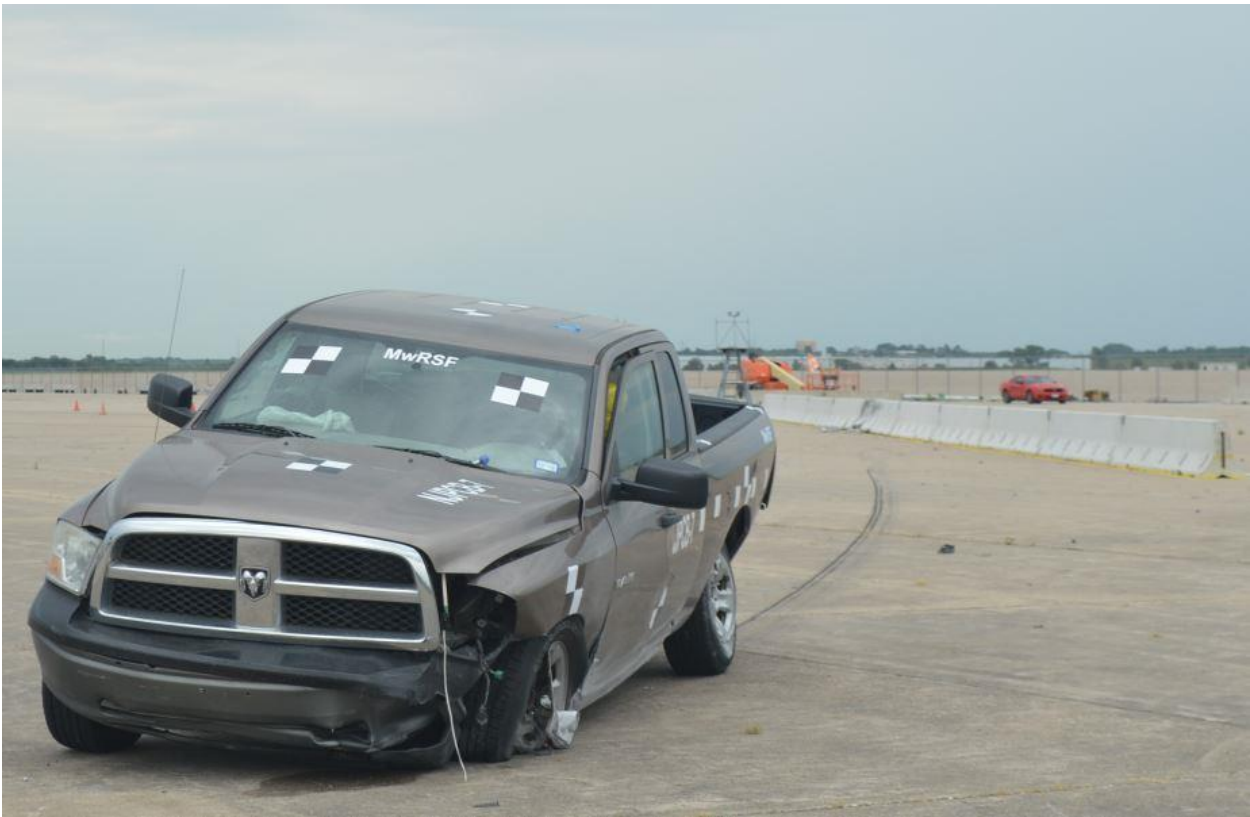
Figure 32. Vehicle Final Position and Trajectory Marks, Test No. NJPCB-7
