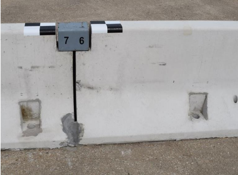
Figure 16. PCB Connection Key and Connection Socket, Test No. NJPCB-7
