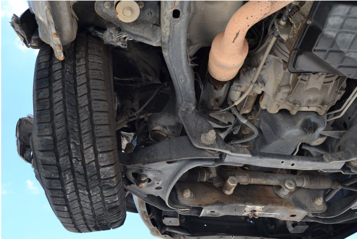
Figure 43. Undercarriage Damage, Test No. NJPCB-7
