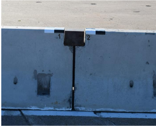
Figure 16. PCB Connection Key and Connection Socket, Test No. NJPCB-3
