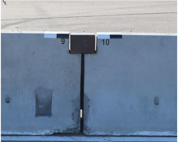
Figure 16. PCB Connection Key and Connection Socket, Test No. NJPCB-3
