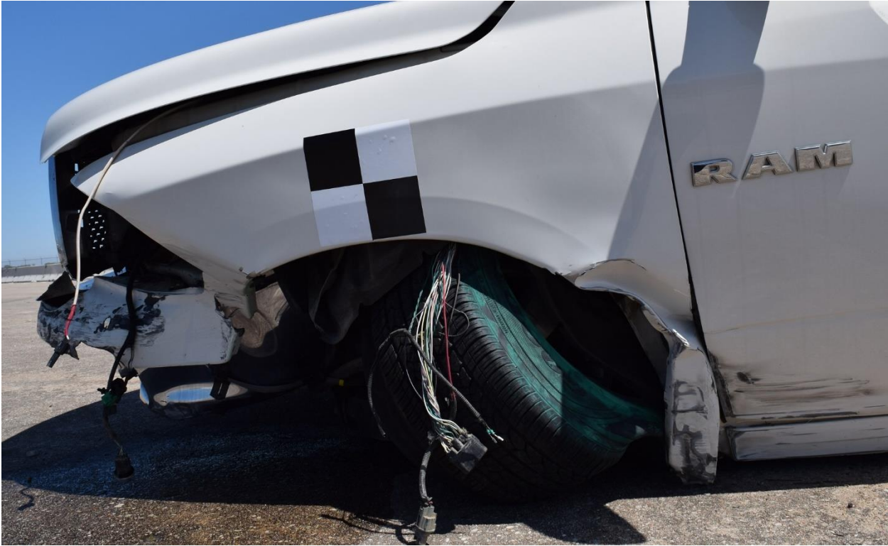
Figure 34. Vehicle Damage on Impact Side, Test No. NJPCB-3
