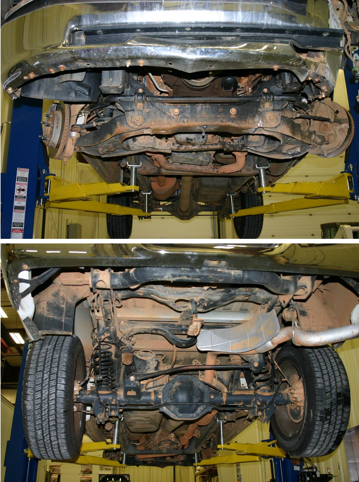
Figure 40. Undercarriage Damage, Test No. NJPCB-1
