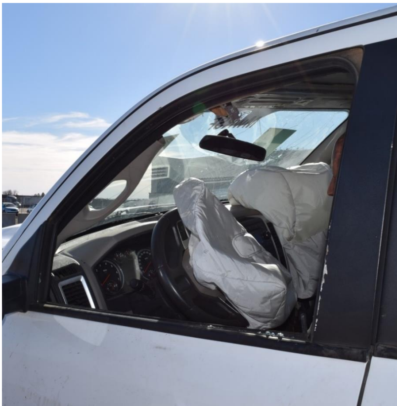
Figure 38. Vehicle Windshield and Window Damage, Test No. NJPCB-1
