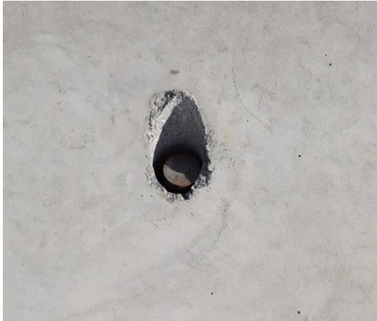
Figure 17. PCB Pin Anchor Recesses, Test No. NJPCB-1
