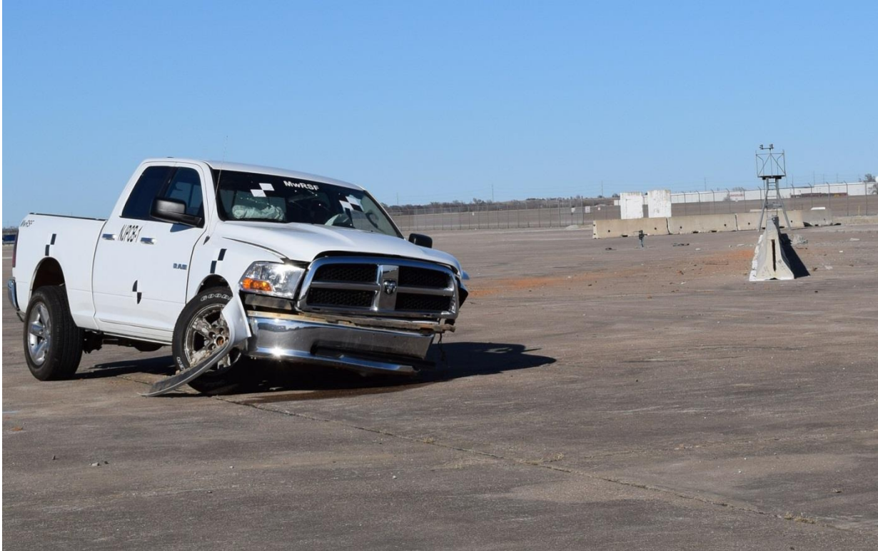
Figure 29. Vehicle Final Position and Trajectory Marks, Test No. NJPCB-1
