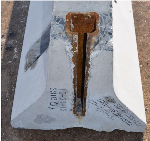
Figure 16. PCB Connection Key and Connection Socket, Test No. NJPCB-1
