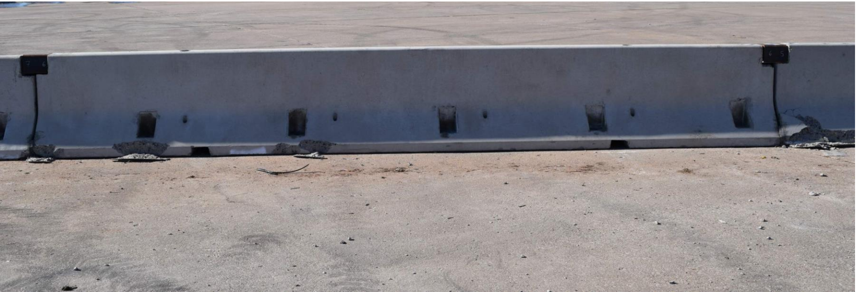
Figure 35. Barrier No. 6 – Traffic and Back Side Damage, Test No. NJPCB-1
