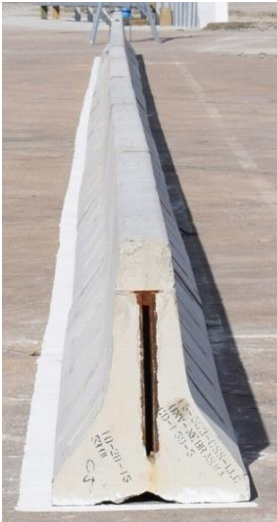
Figure 15. NJDOT PCB with Pinned Configuration and Grouted Toes Test Installation, Test No. NJPCB-1
