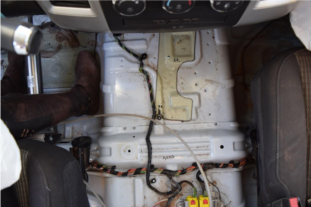
Figure 39. Occupant Compartment Deformation, Test No. NJPCB-1
