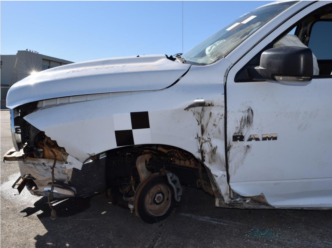
Figure 37. Vehicle Damage on Impact Side, Test No. NJPCB-1
