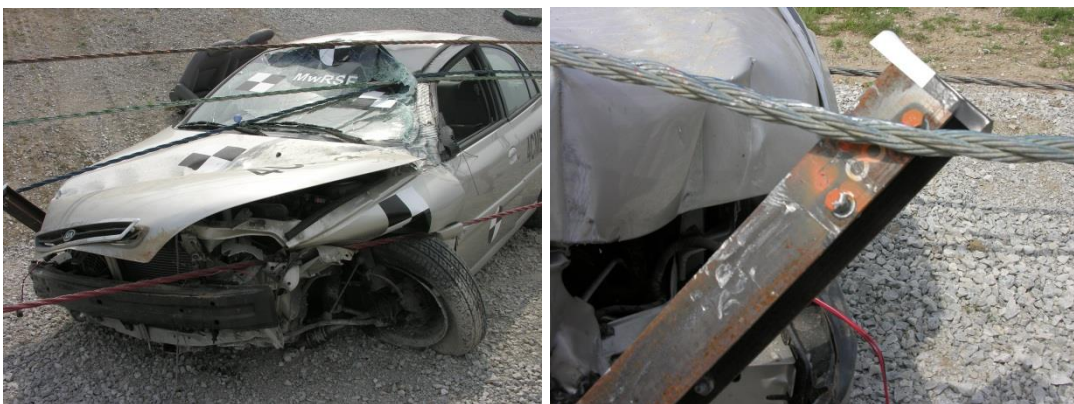
Figure 2. 1100C Full-Scale Crash Test Failure
