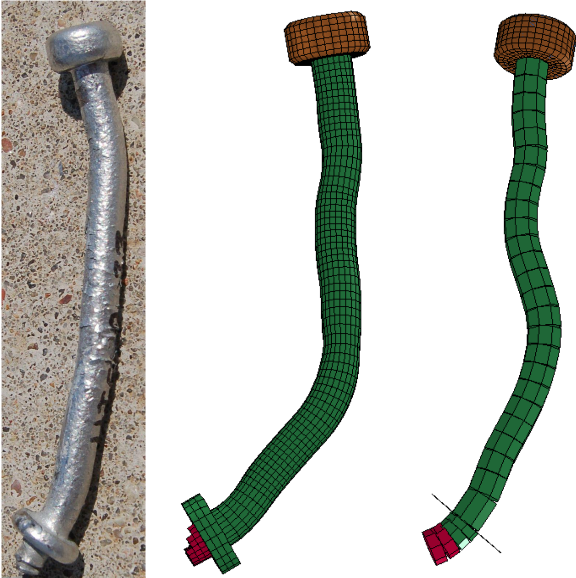
Figure 30. Comparison of Component Test with Solid Element and Beam Element Models
