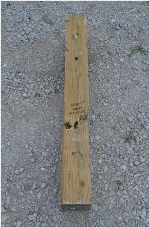
Figure 9. Post No. 25 Damage, Test No. MGSLs-2
