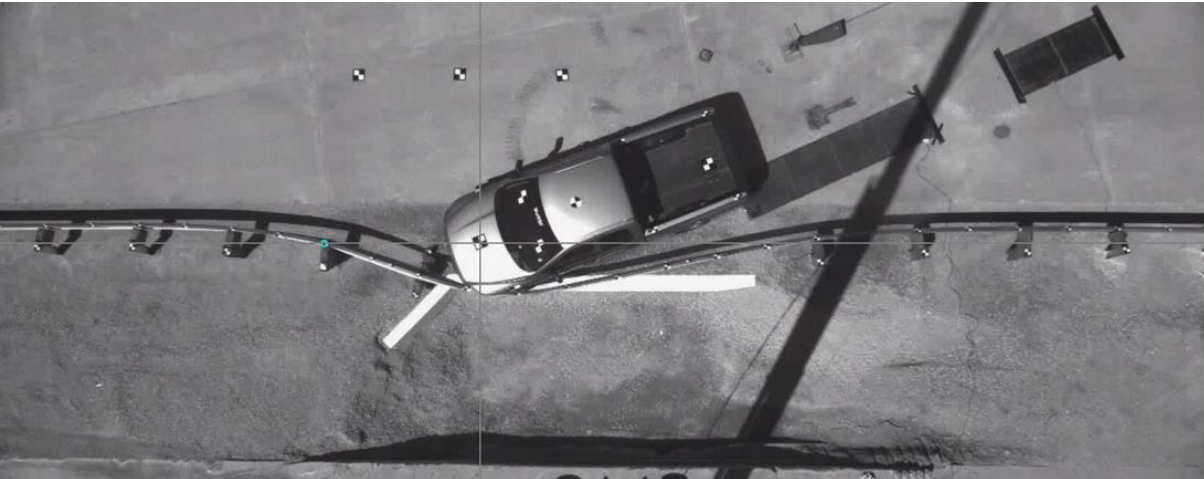
Fracture of Second CRT Downstream of Unsupported Span
