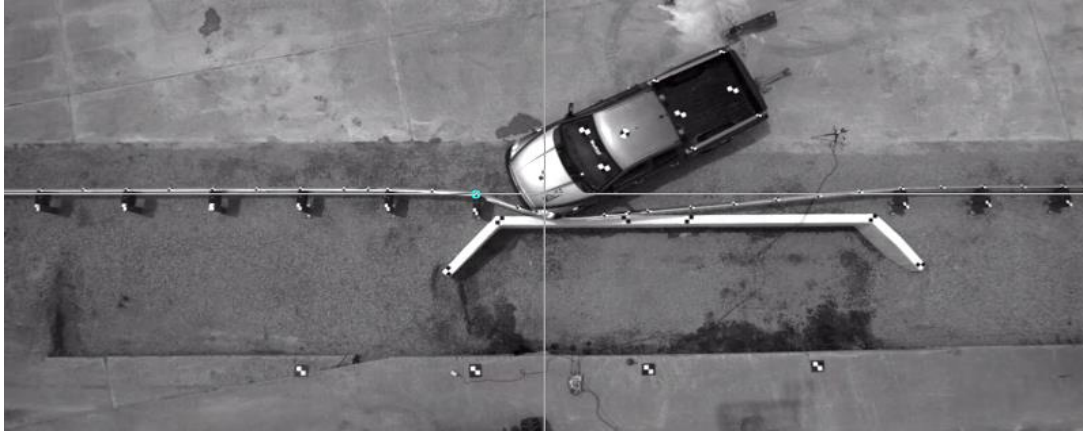
Fracture of First UBSP Downstream of Unsupported Span
