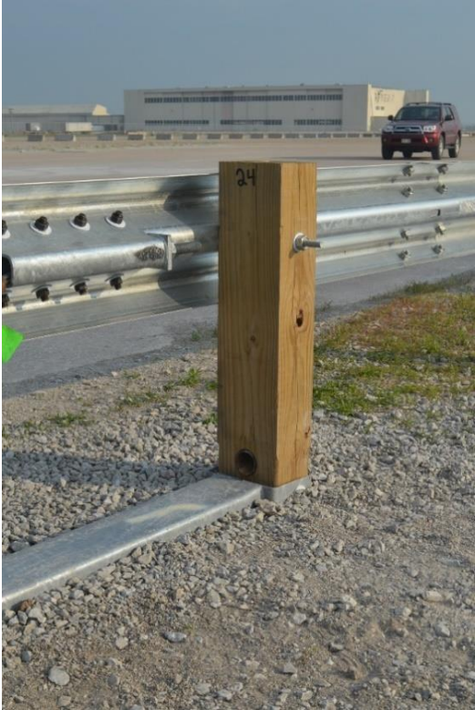
Figure 3. Long-Span End-Anchorage System, Test No. MGSL-2
