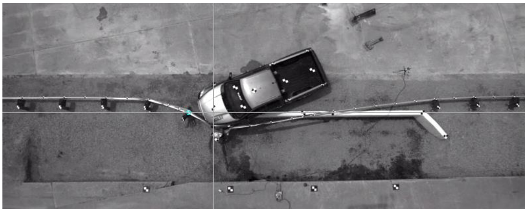
Fracture of Second UBSP Downstream of Unsupported Span
