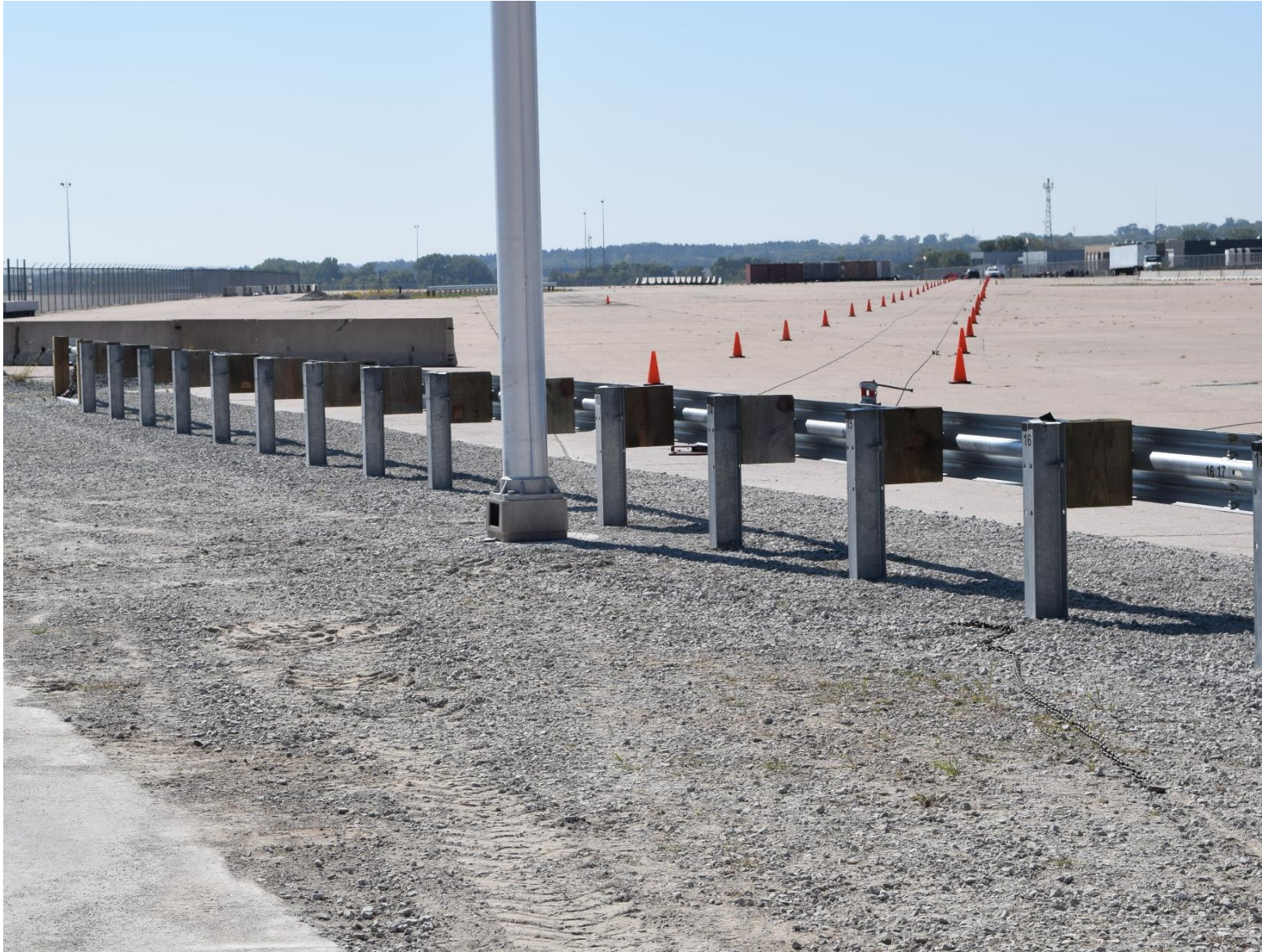
Figure 63. Test Installation, Test No. ILT-1
