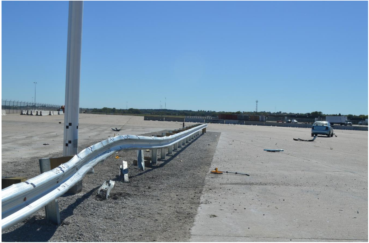
Figure 127. Vehicle Final Position and Trajectory Marks, Test No. ILT-2
