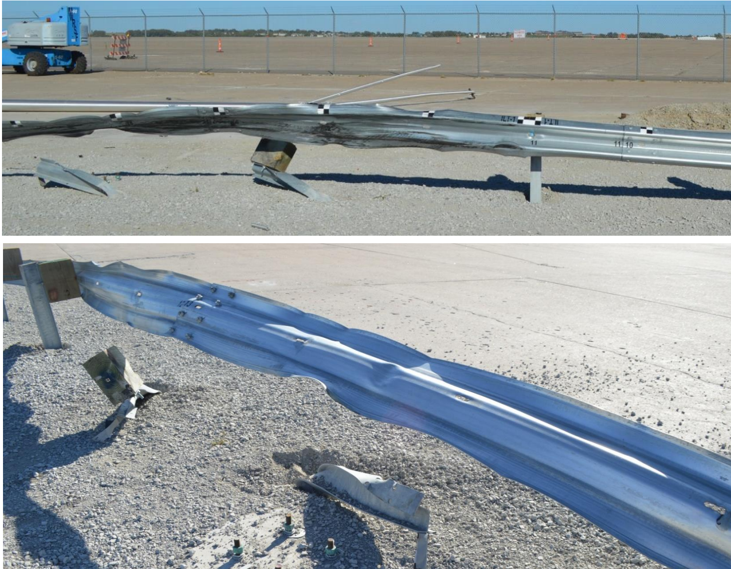
Figure 114. Rail Damage, Test No. ILT-1
