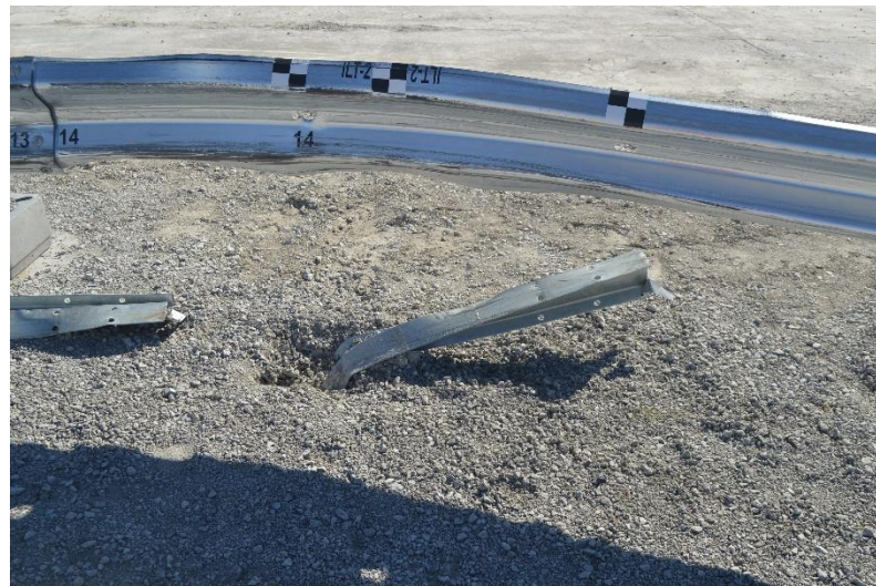
Figure 131. Post Nos. 12 through 15 Damage, Test No. ILT-2
