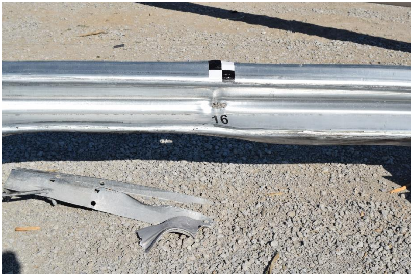
Figure 116. System Damage, Post Nos. 15 through 17 Damage, Test No. ILT-1
