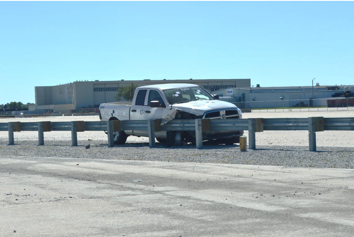
Figure 112. Vehicle Final Position and Trajectory Marks, Test No. ILT-1
