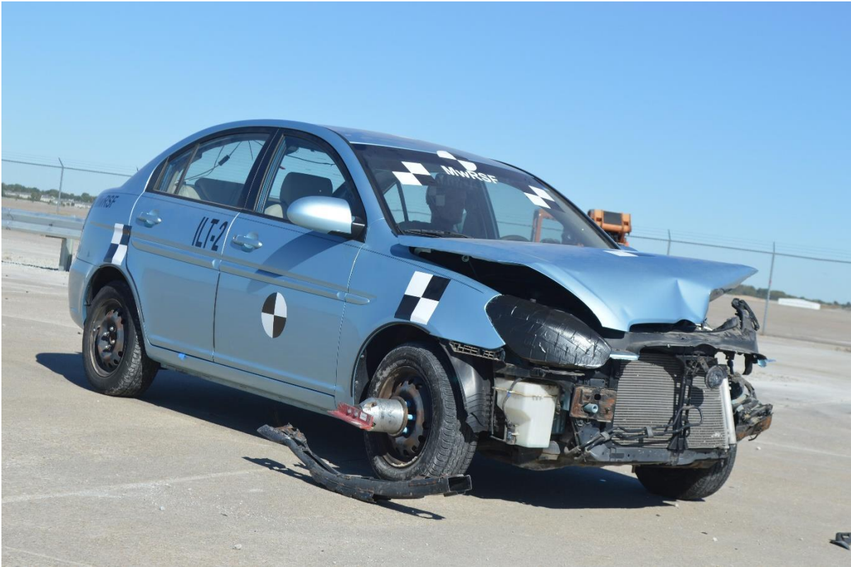
Figure 133. Vehicle Damage, Test No. ILT-2
