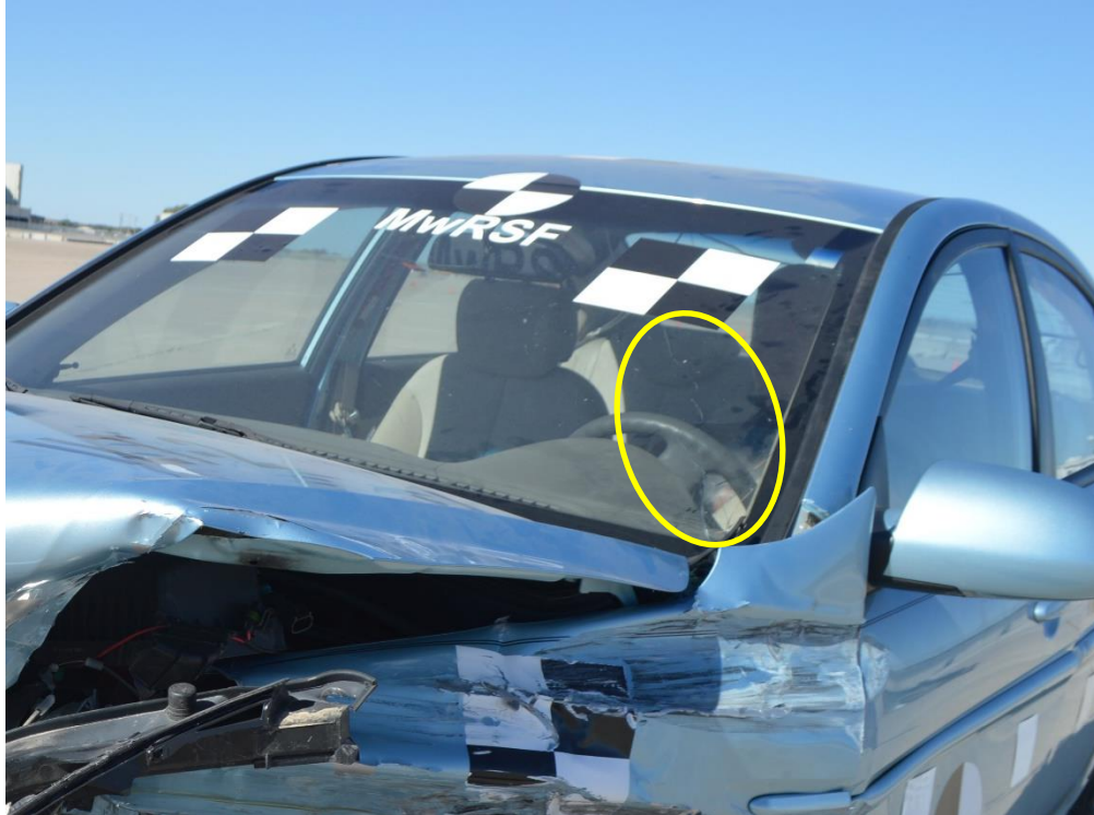
Figure 135. Vehicle Windshield Crack, Test No. ILT-2
