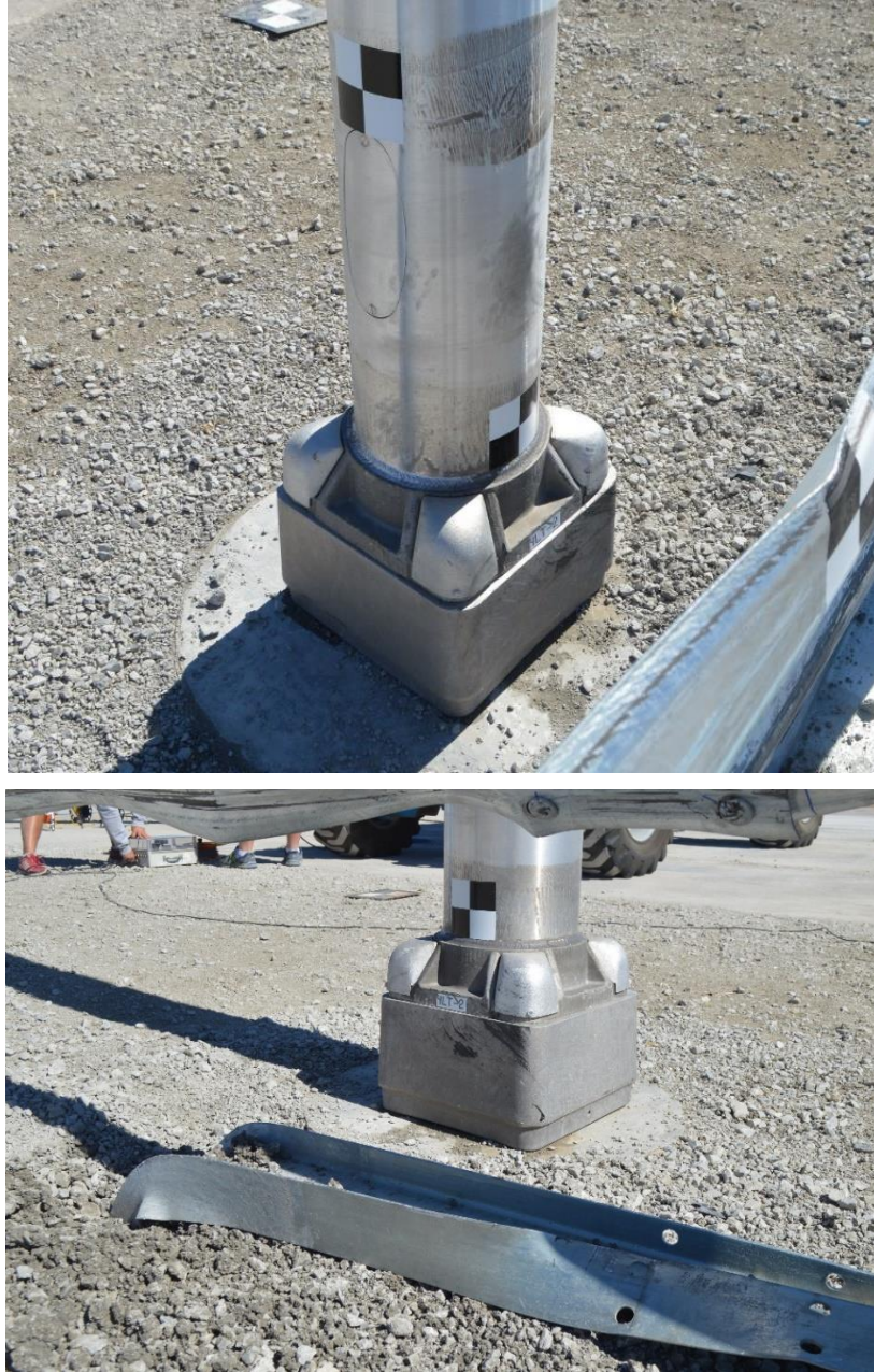
Figure 132. Pole Contact Marks, Test No. ILT-2
