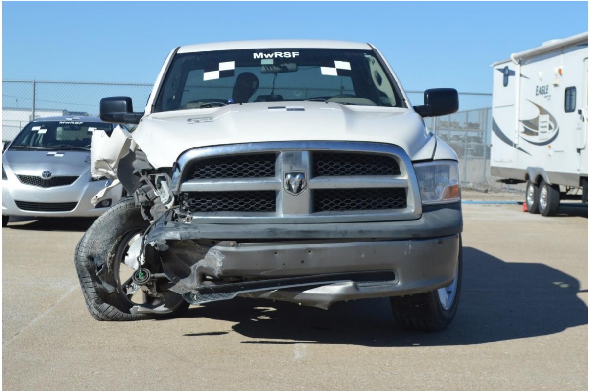
Figure 120. Vehicle Damage, Test No. ILT-1
