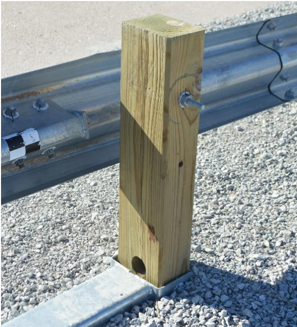
Figure 117. Upstream Anchor Damage, Test No. ILT-1
