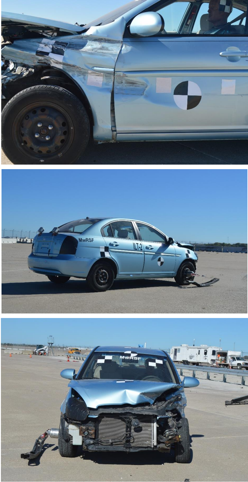
Figure 134. Vehicle Damage, Test No. ILT-2
