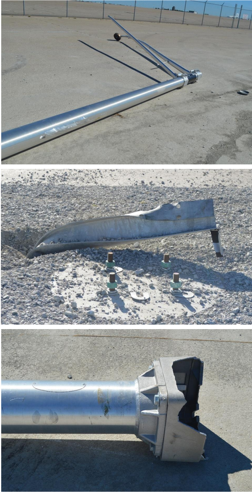
Figure 119. Pole Damage, Test No. ILT-1
