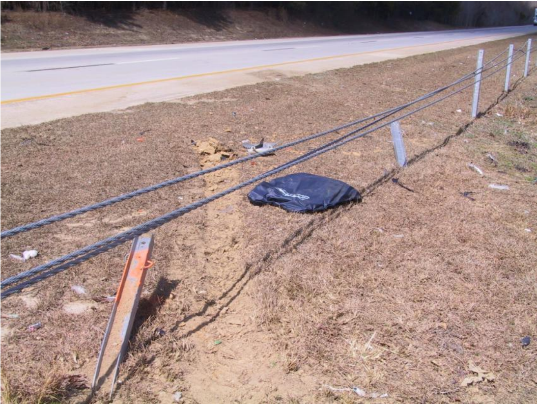
Figure 99. Diving Underride Penetration Crash in North Carolina
