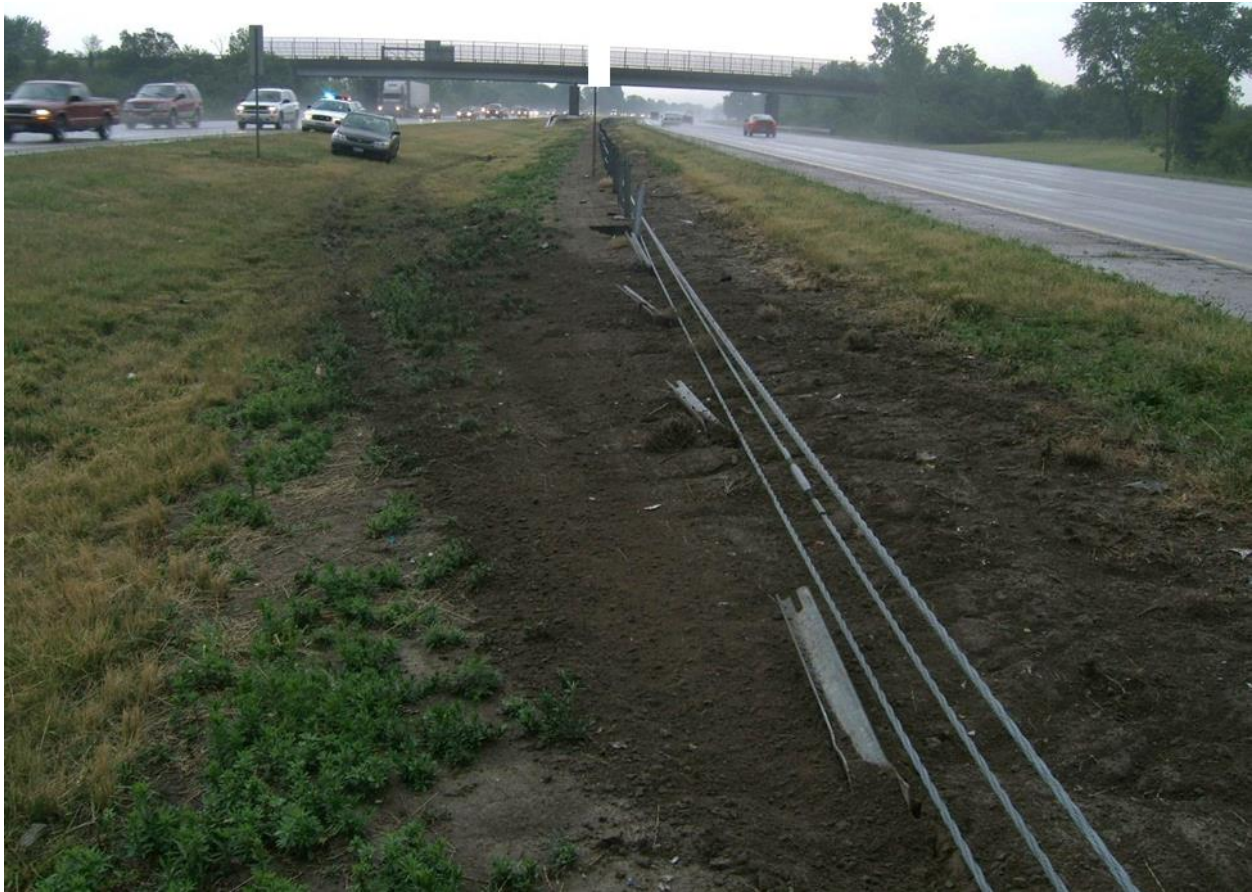
Figure 115. Crash Scene Photographs, Simulation No. 2
