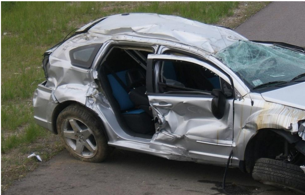
Figure 132. Example Rollover Crash Caused by Redirection on Back Slope (continued)
