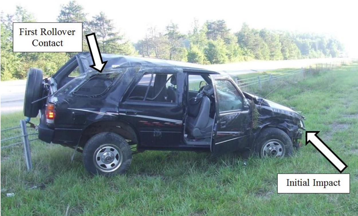
Figure 136. Third Example Rollover Crash Caused by High Orientation Angle at Impact
