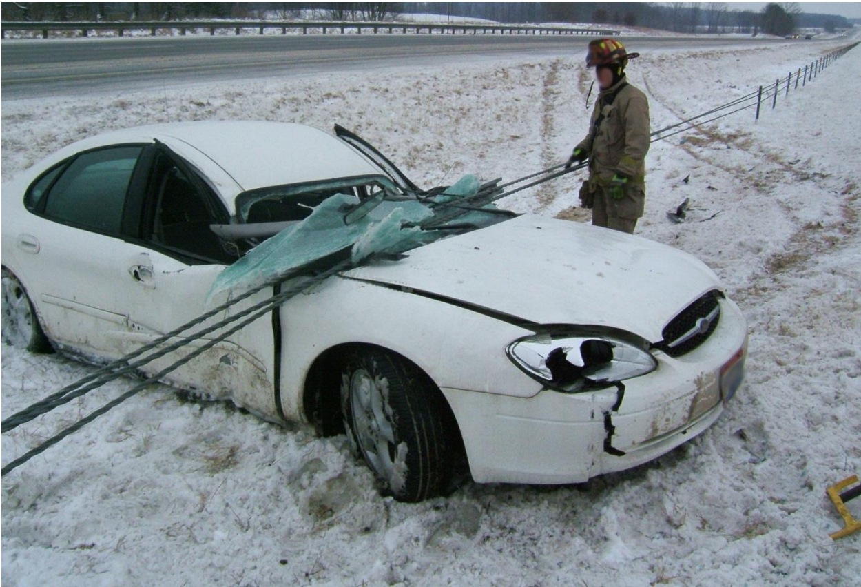
Figure 94. Diving Potential Underride Penetration Crash on Nucor NU-CABLE Barrier
