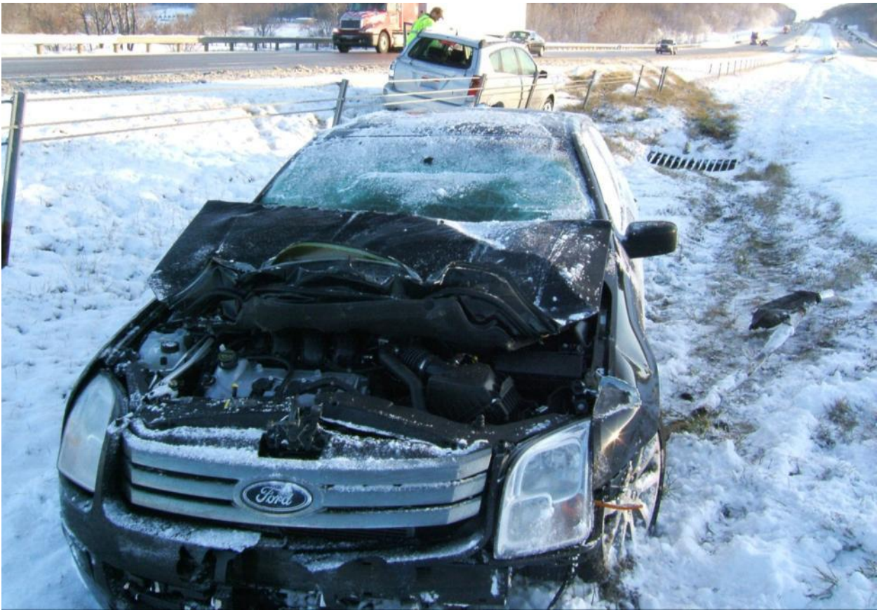
Figure 93. Diving Underride Penetration Crash on Nucor NU-CABLE Barrier
