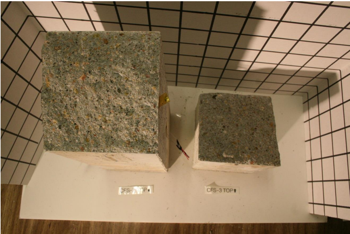
Figure 162. Additional Post-Test Damage, Test No. CFS-3 [10-in. (254-mm) Span]
