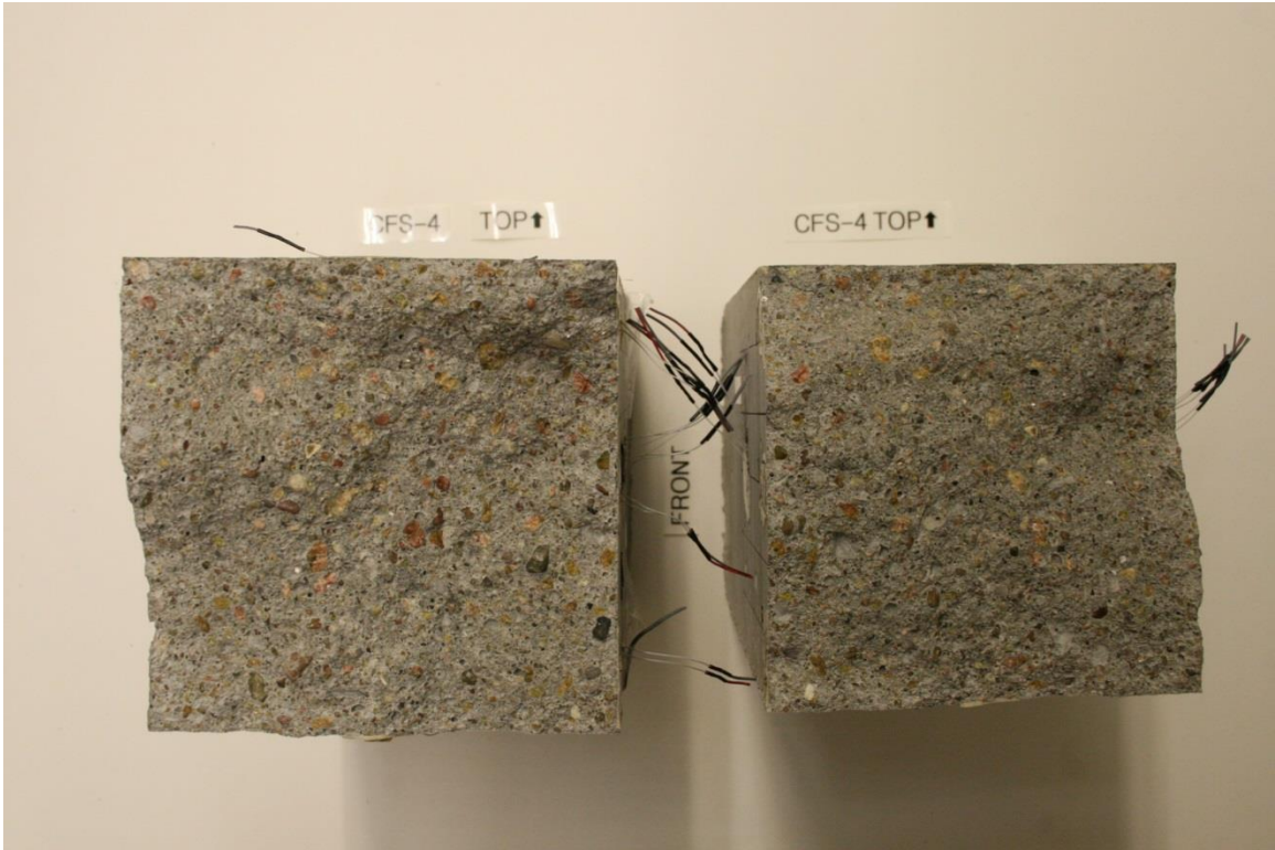
Figure 173. Additional Post-Test Damage, Test No. CFS-4 [11-in. (279-mm) Span]
