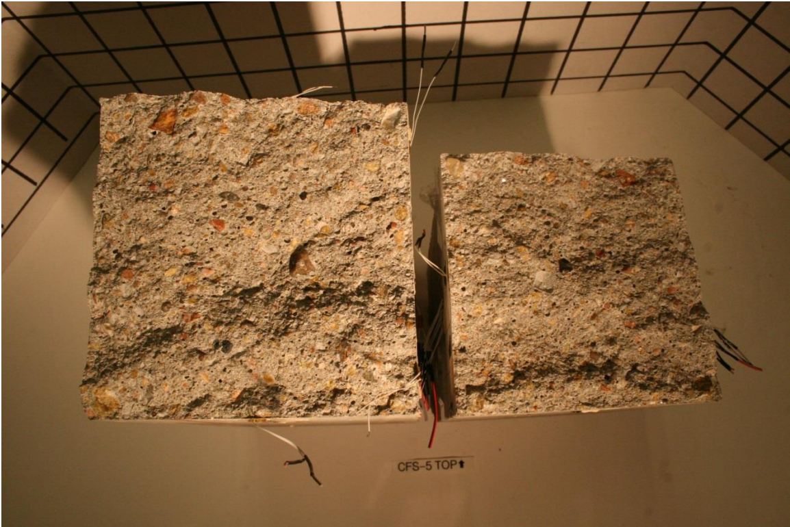
Figure 186. Additional Post-Test Damage, Test No. CFS-5 [10-in. (254-mm) Span]
