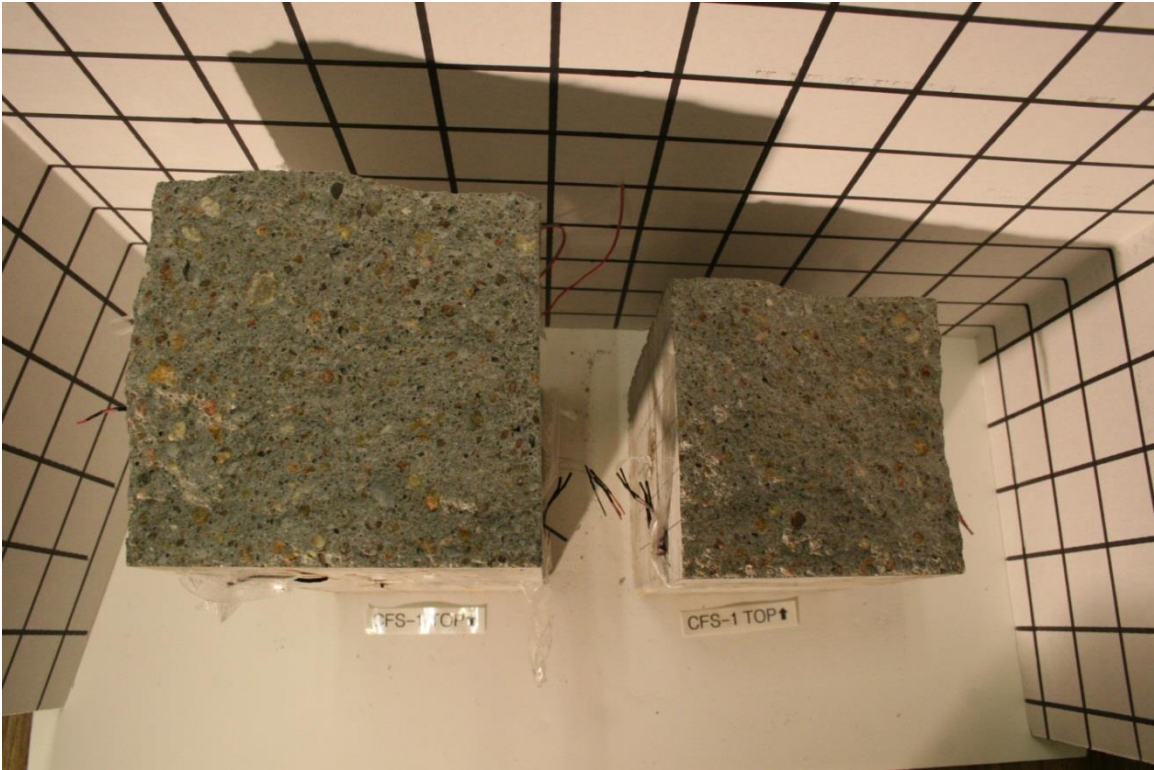
Figure 139. Additional Post-Test Damage, Test No. CFS-1 [18-in. (457-mm) Span]
