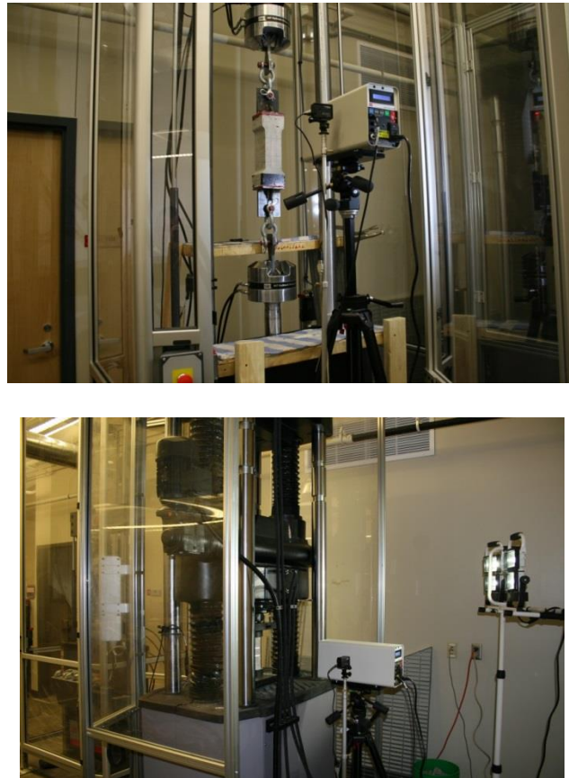
Figure 101. Typical GoPro Digital Video Camera Setup
