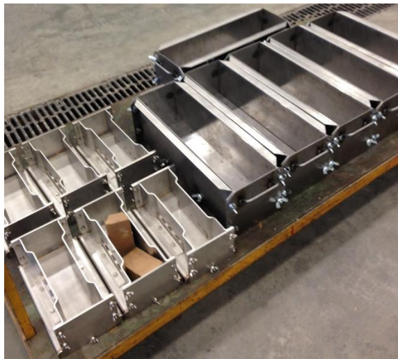
Figure 91. Metal Molds for Tension, Flexure, and Shear Concrete Specimens
