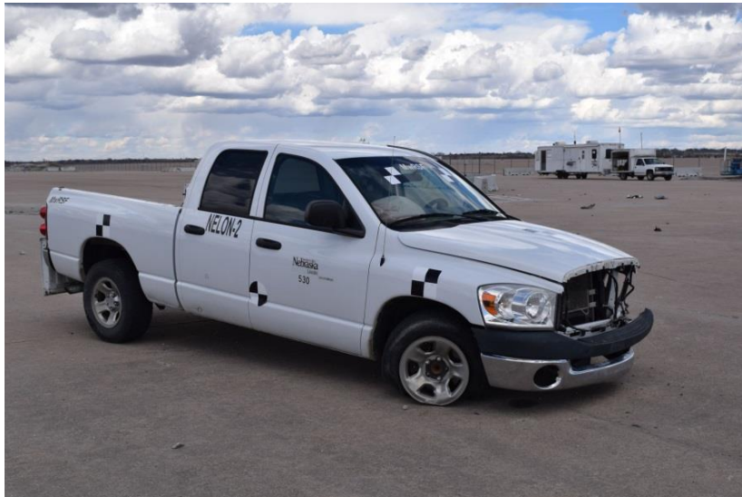
Figure 97. Vehicle Damage, Test No. NELON-2
