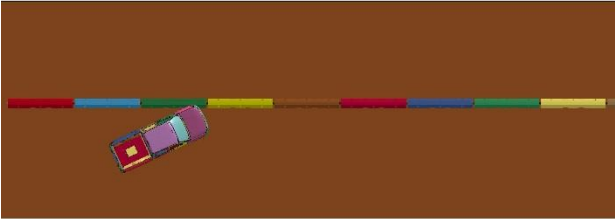
(c) impact US of joint between barrier nos. 3 and 4
