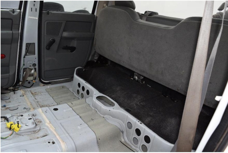
Figure 82. Occupant Compartment Damage, Test No. NELON-1
