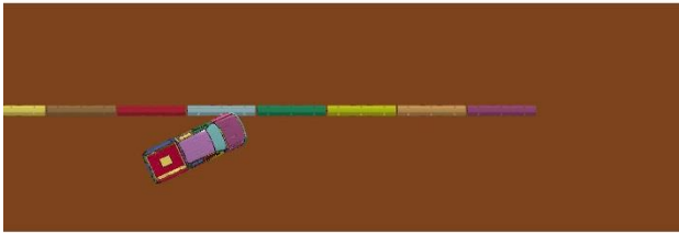
(d) impact US of joint between barrier nos. 12 and 13
