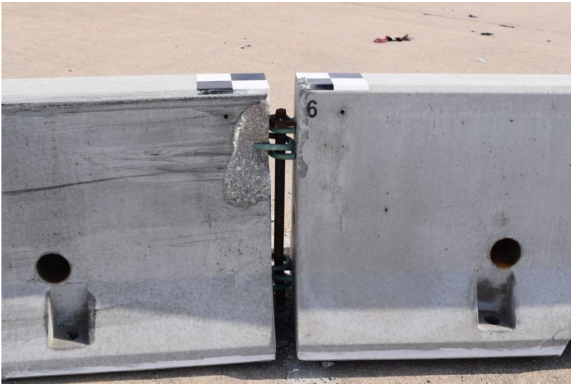
Figure 77. Barrier No. 5 Damage, Test No. NELON-1
