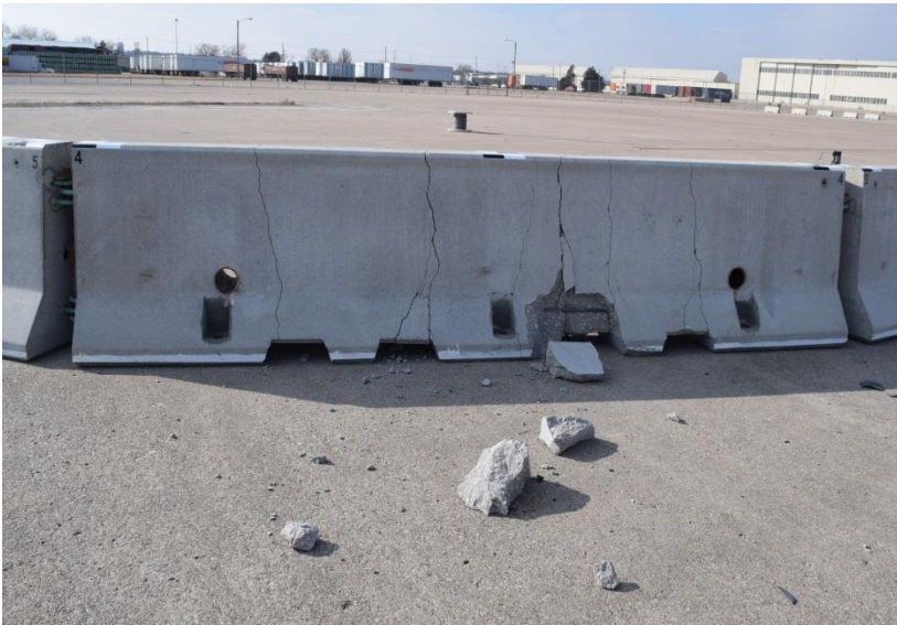
Figure 76. Barrier No. 4 Damage, Test No. NELON-1
