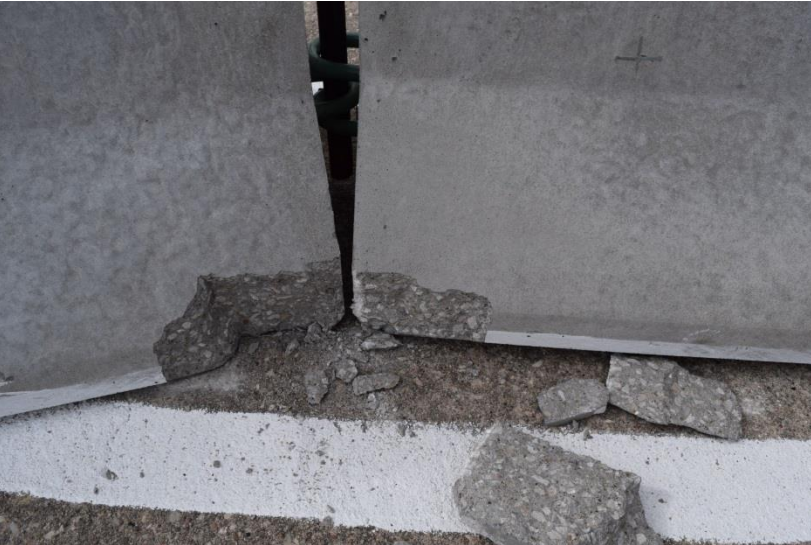
Figure 74. Barrier Nos. 1 and 2 Damage, Test No. NELON-1
