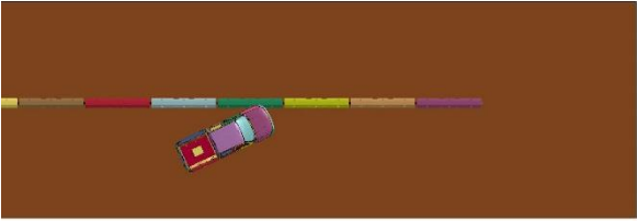
(e) impact US of joint between barrier nos. 13 and 14
