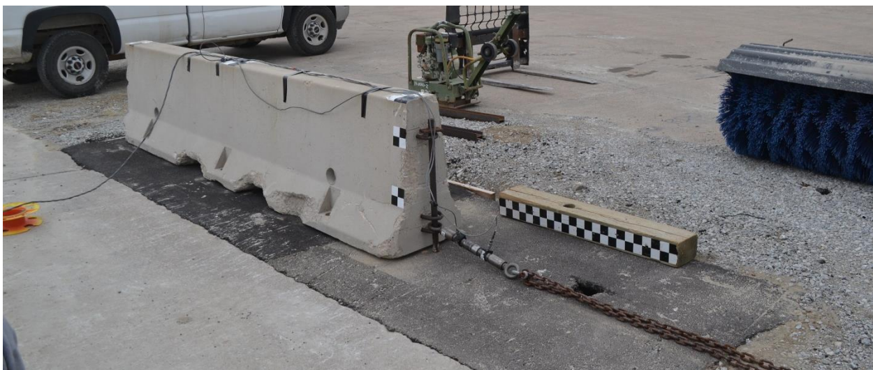
Figure 1. Quasi-Static Pull Test Setup, Test No. TCBFA-1
