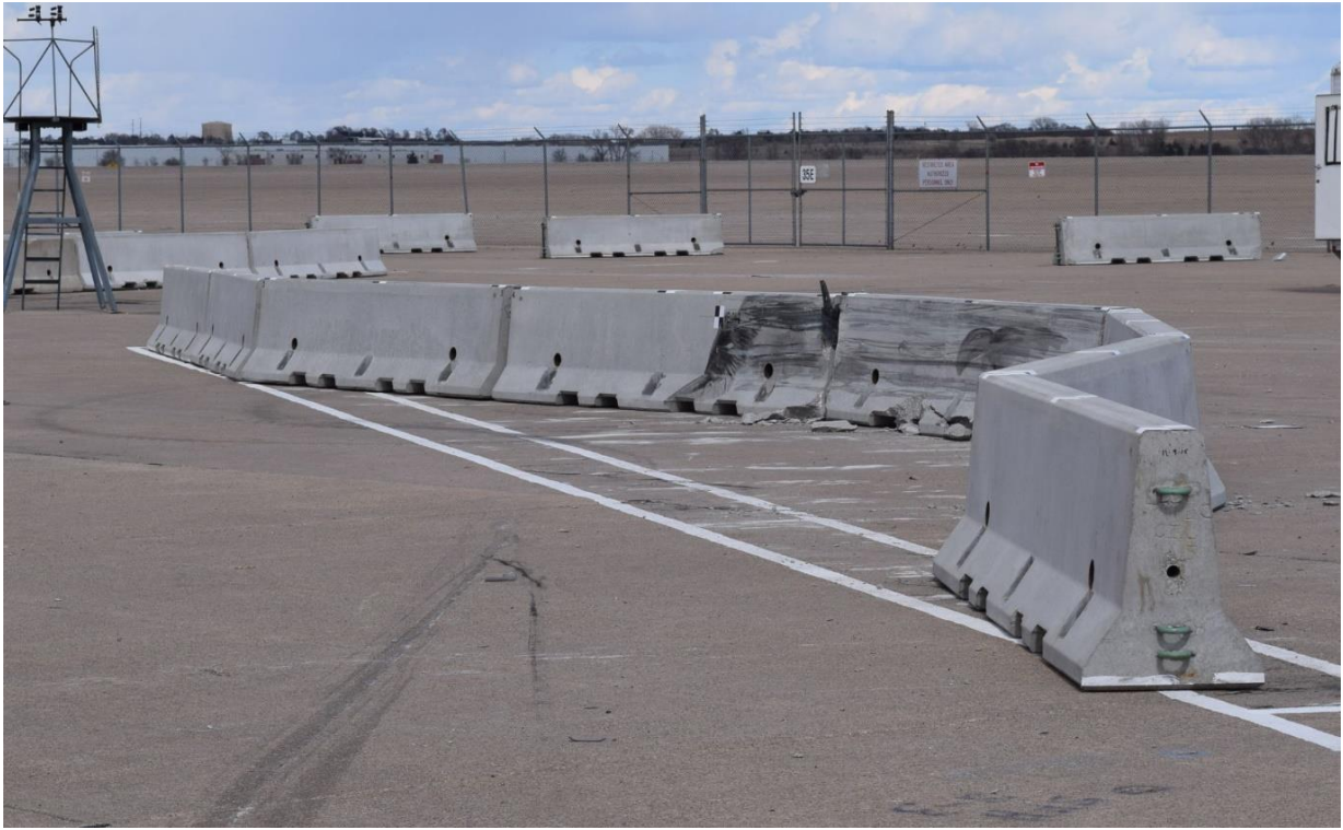
Figure 91. System Deflection and Damage, Test No. NELON-2
