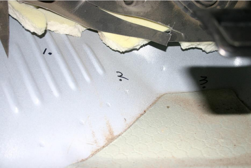
Figure 99. Occupant Compartment Damage, Test No. NELON-2
