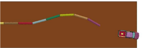
(e) impact US of joint between barrier nos. 13 and 14
