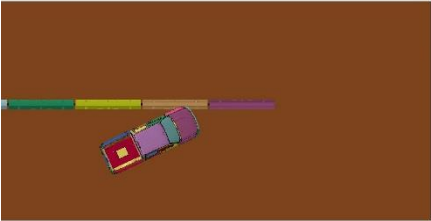
(g) impact US of joint between barrier nos. 15 and 16
