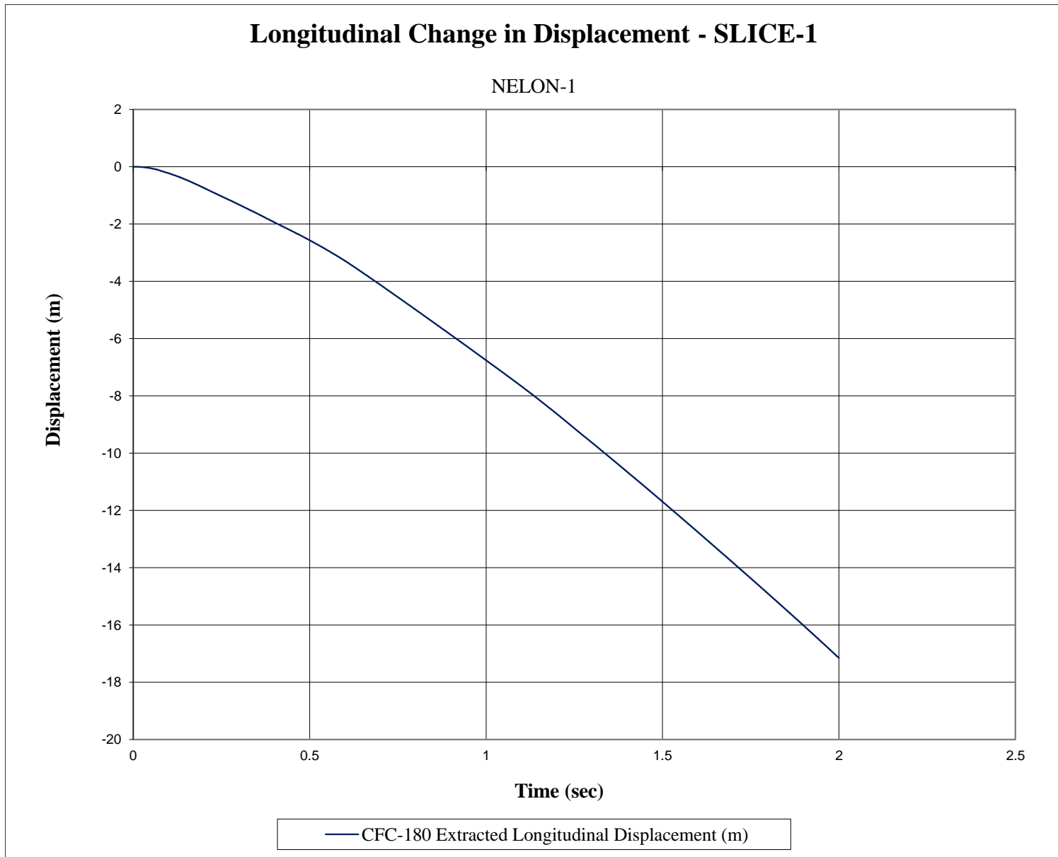
Figure D-3. Longitudinal Occupant Displacement (SLICE-1), Test No. NELON-1
