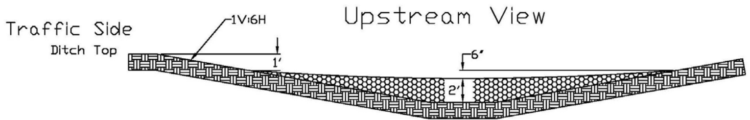
Figure 7. Preliminary Design Guideline - Rock Check Dam Schematic
