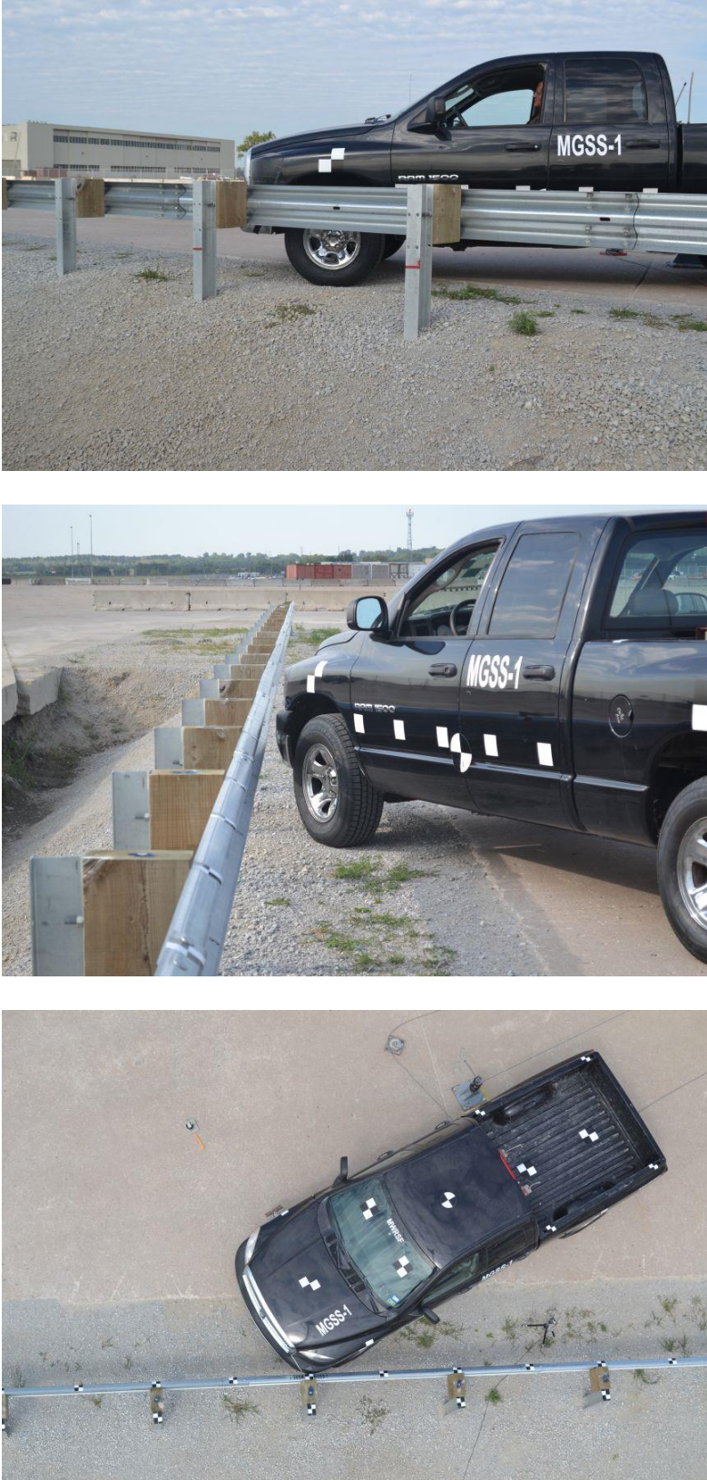
Figure 24. Impact Location, Test No. MGSS-1
