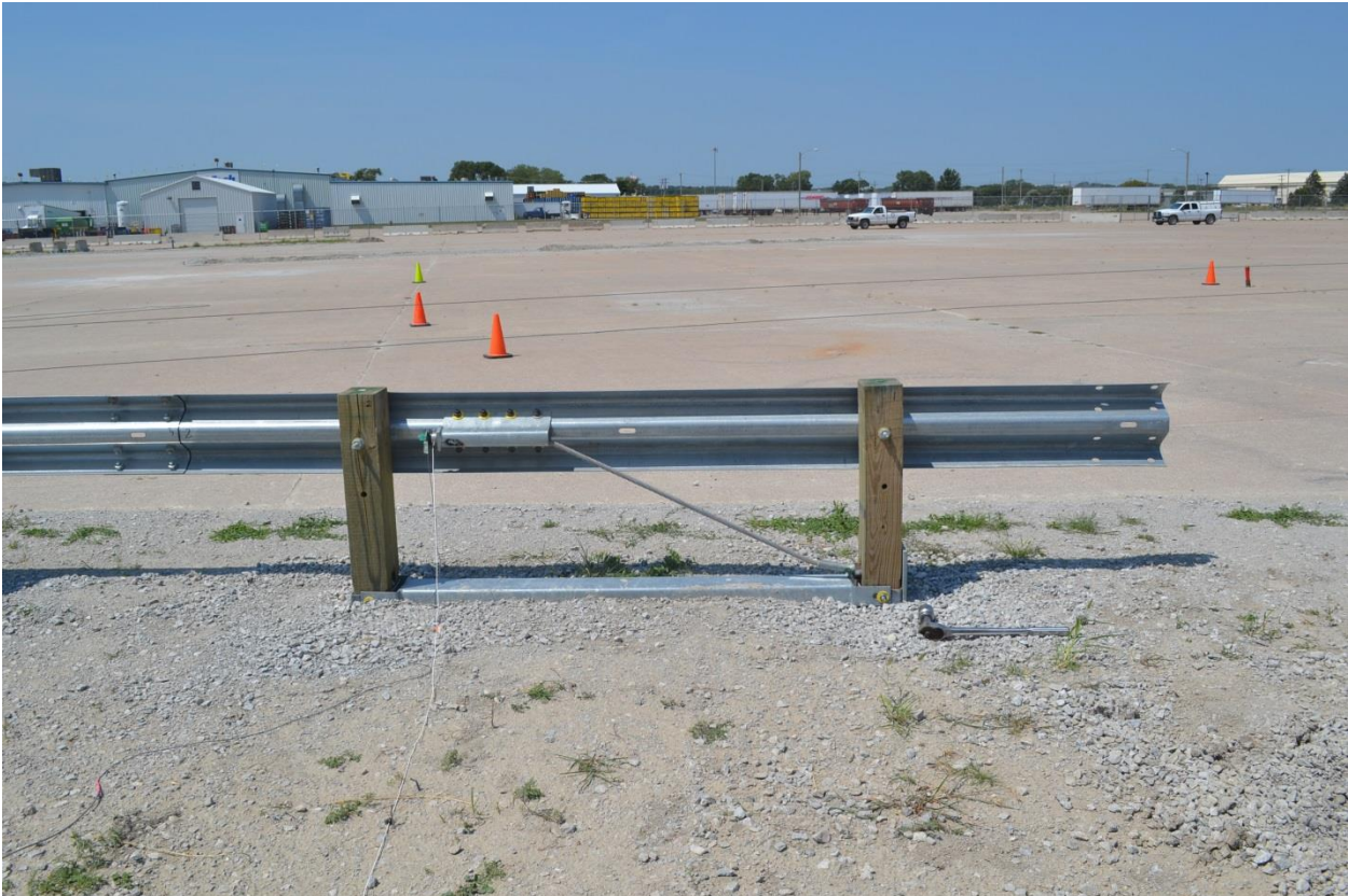
Figure 18. Load Cell Placement, Test No. MGSS-1
