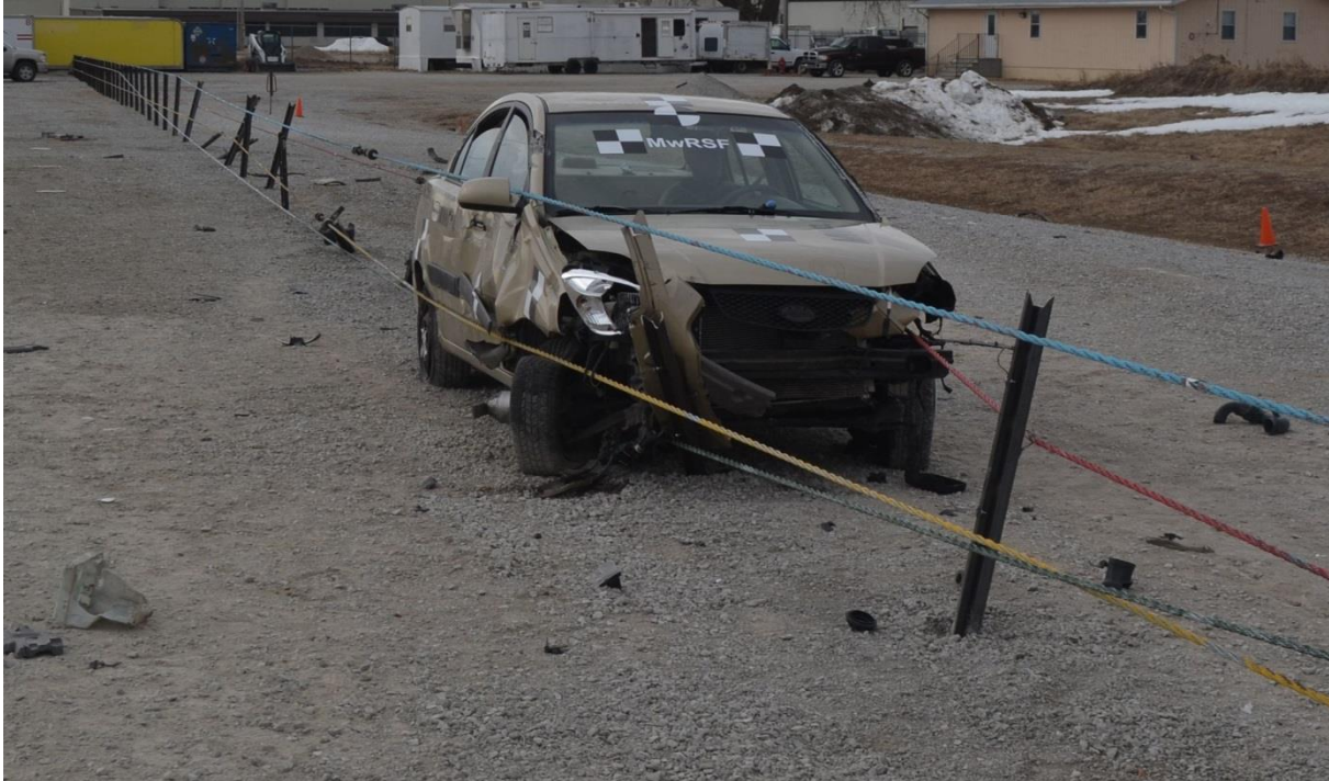
Figure 147. Vehicle Final Position and Trajectory Marks, Test No. MWP-7
