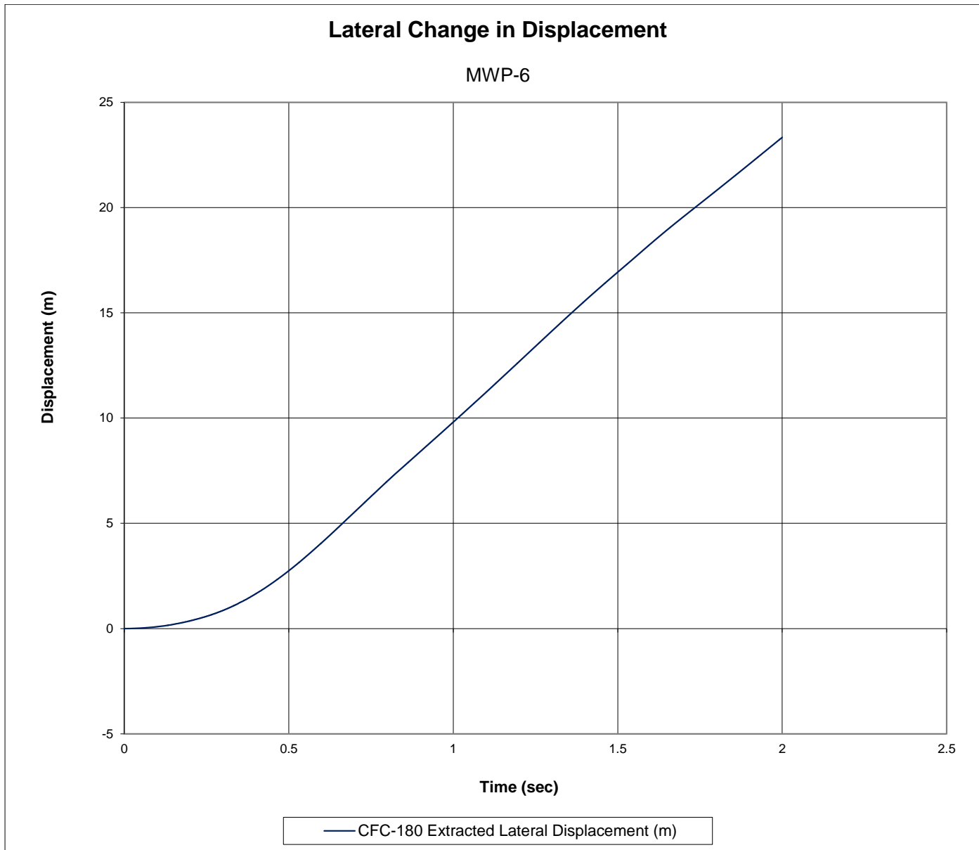
Figure G-14. Lateral Occupant Displacement (SLICE 2), Test No. MWP-6
