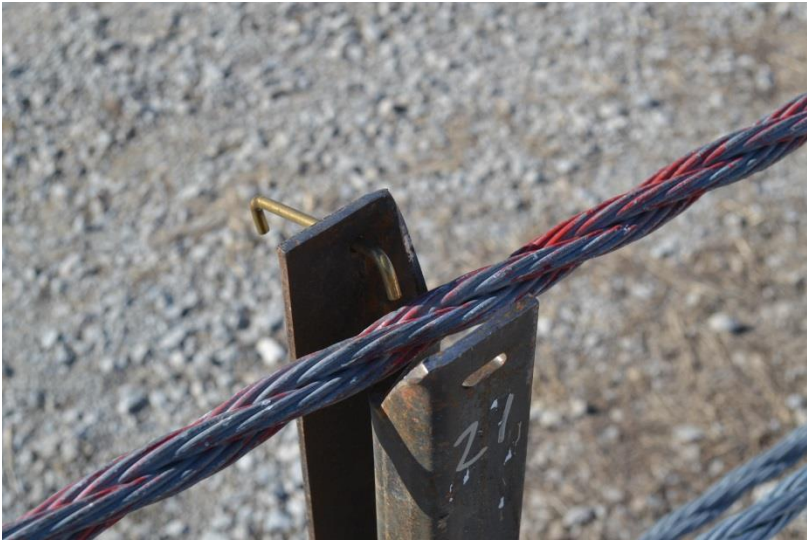
Figure 151. System Damage, Brass Rods, Test No. MWP-7
