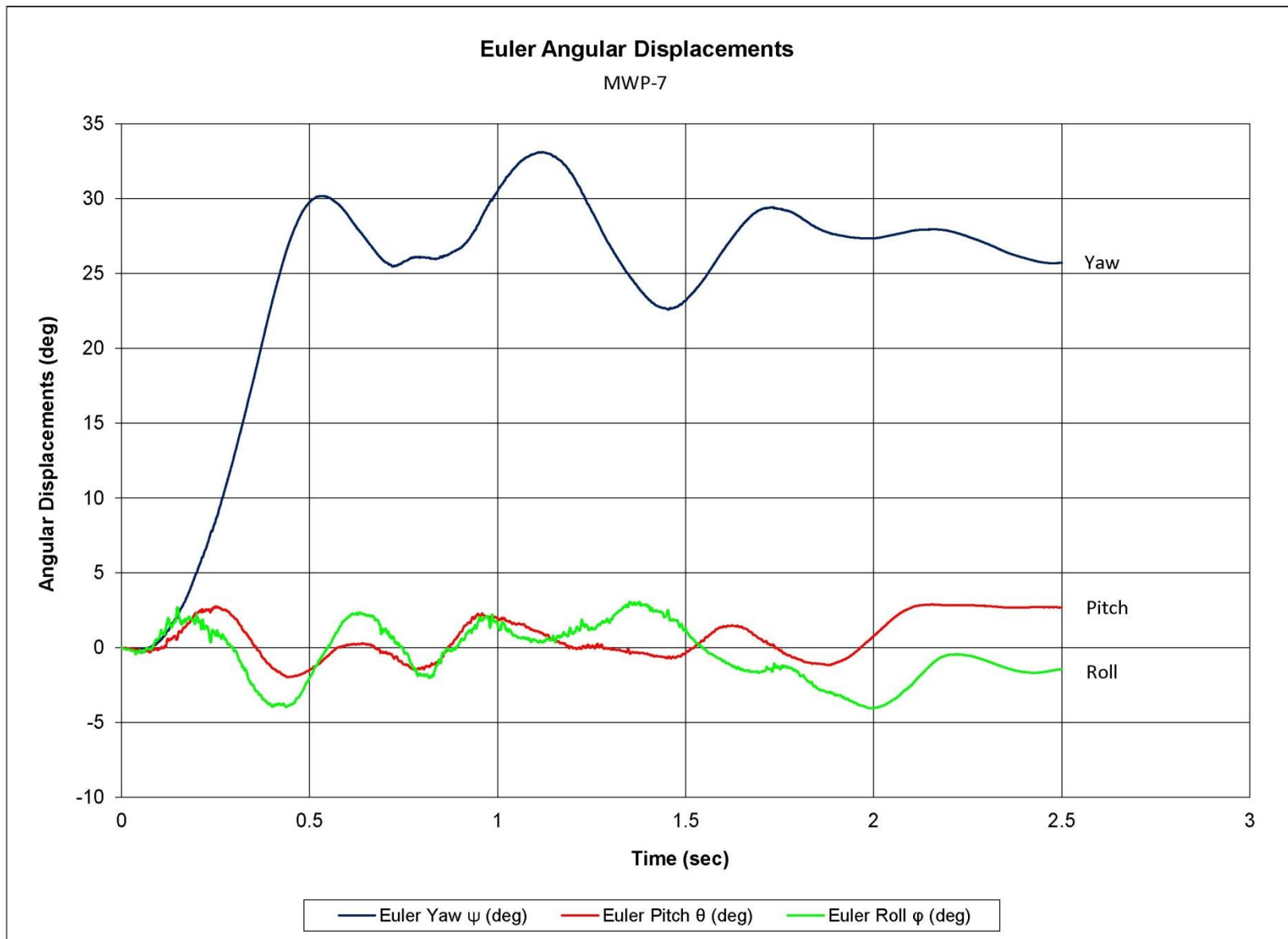
Figure I-15. Vehicle Angular Displacements (SLICE 2), Test No. MWP-7
