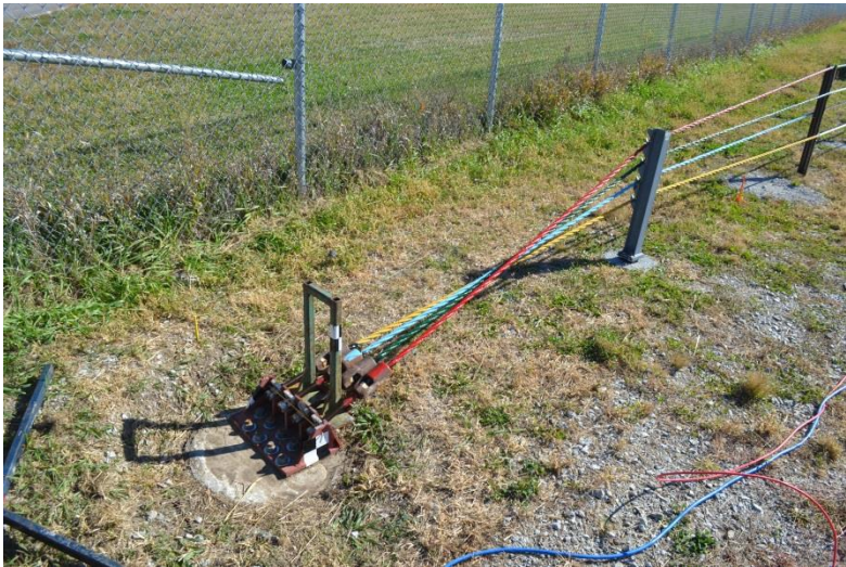
Figure 50. System Damage, End Anchorages, Test No. MWP-4
