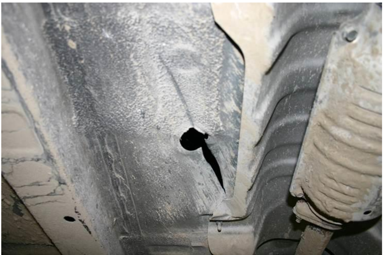
Figure 108. Occupant Compartment Penetration, Test No. MWP-6
