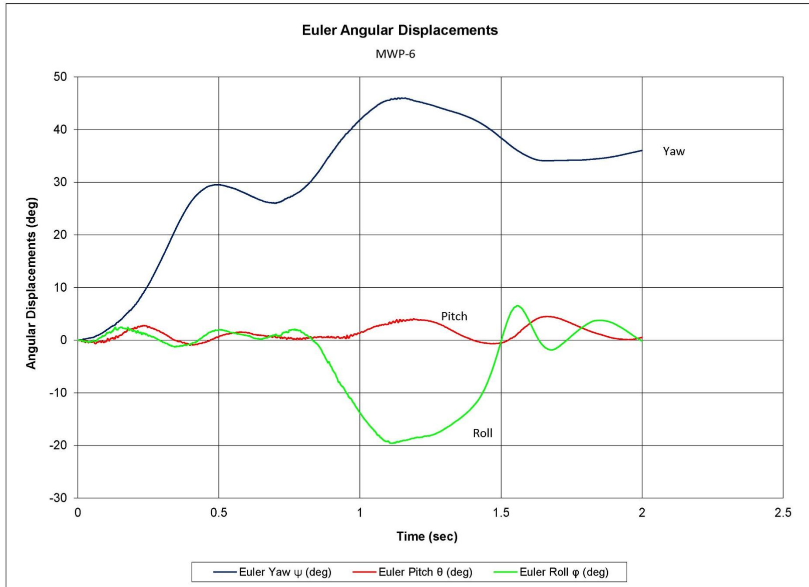
Figure G-7. Vehicle Angular Displacements (SLICE 1), Test No. MWP-6
