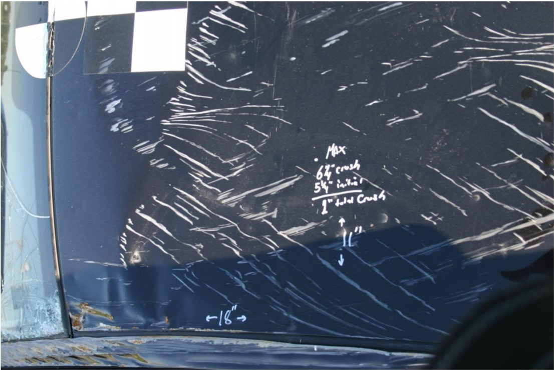
Figure D-11. Roof Deformation Documentation, Test No. MWP-6
