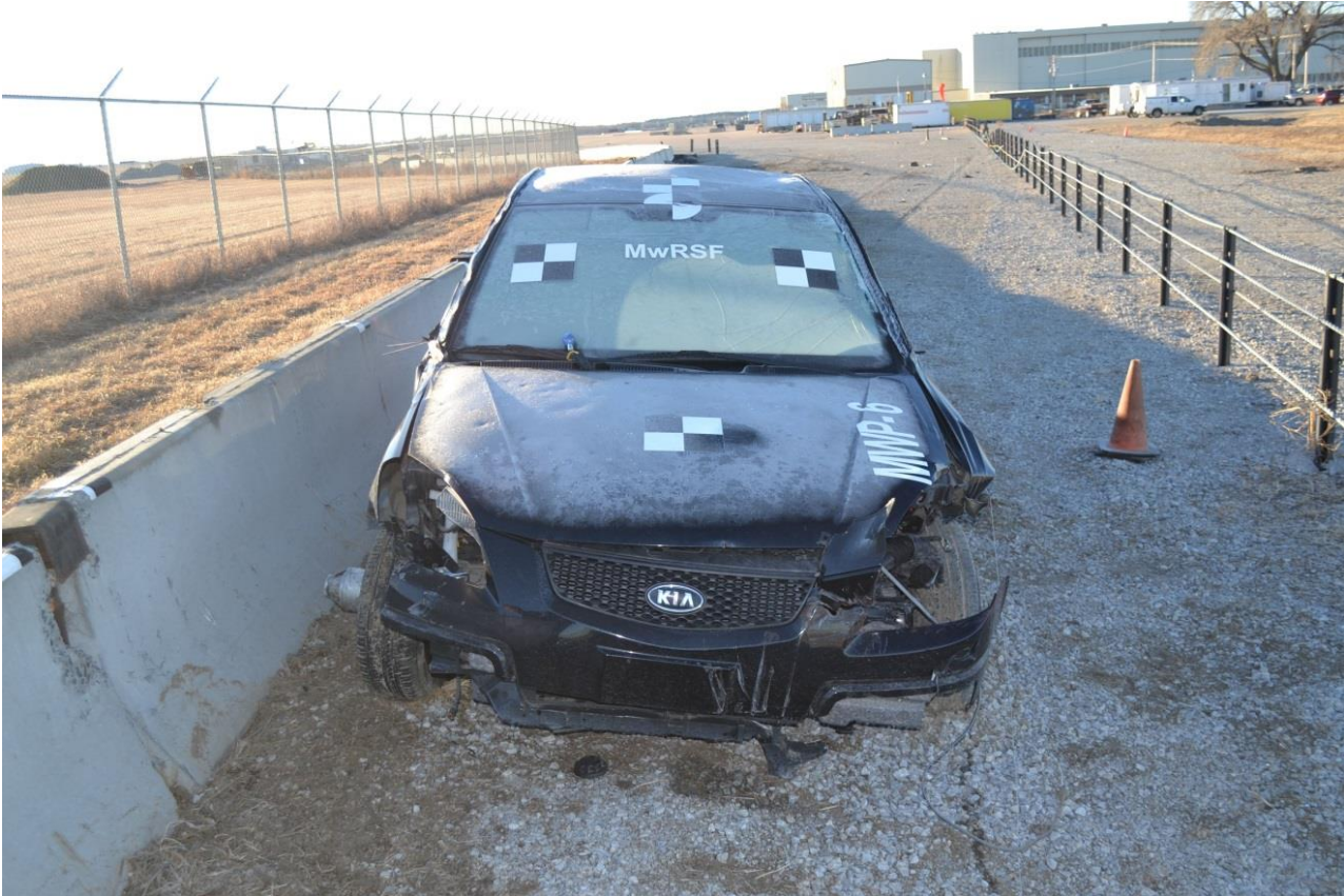
Figure 95. Vehicle Final Position and Trajectory Marks, Test No. MWP-6
