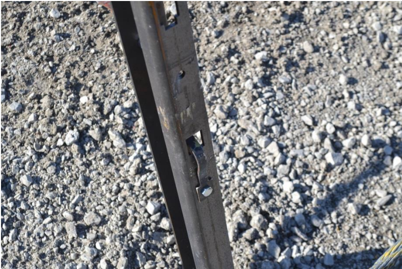
Figure 150. System Damage, Cable Brackets, Test No. MWP-7
