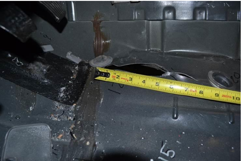
Figure 107. Occupant Compartment Damage, Test No. MWP-6
