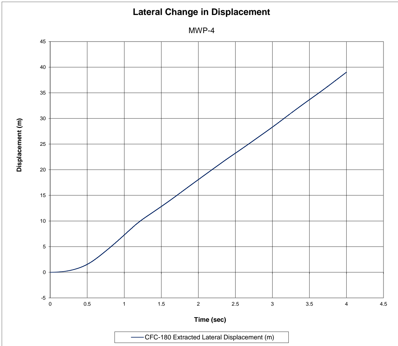
Figure E-14. Lateral Occupant Displacement (SLICE 2), Test No. MWP-4
