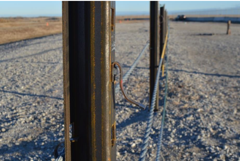
Figure 98. System Damage, Cable Brackets, Test No. MWP-6
