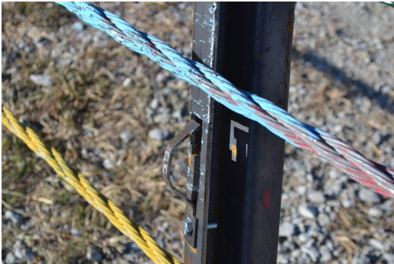
Figure 51. System Damage, Cable Brackets, Test No. MWP-4
