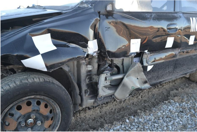
Figure 106. Vehicle Damage, Test No. MWP-6
