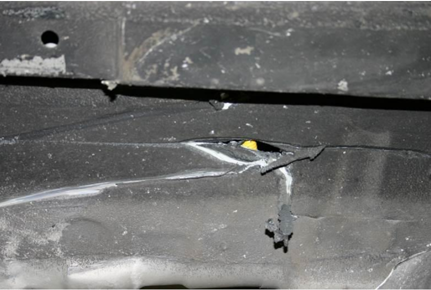
Figure 162. Occupant Compartment Damage, Test No. MWP-7
