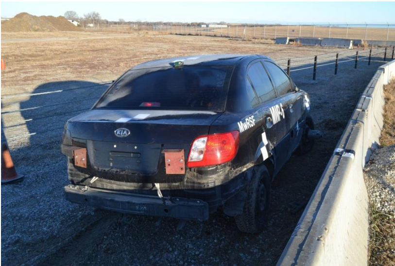
Figure 105. Vehicle Damage, Test No. MWP-6
