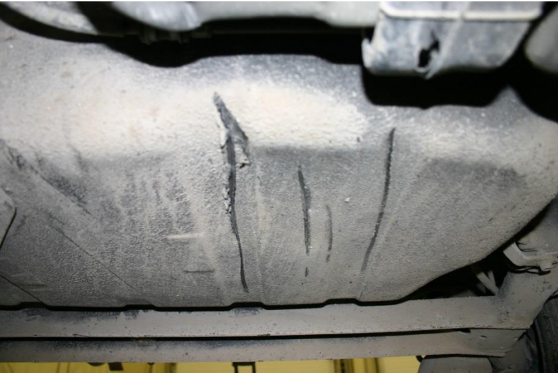
Figure 110. Additional Undercarriage Damage, Test No. MWP-6
