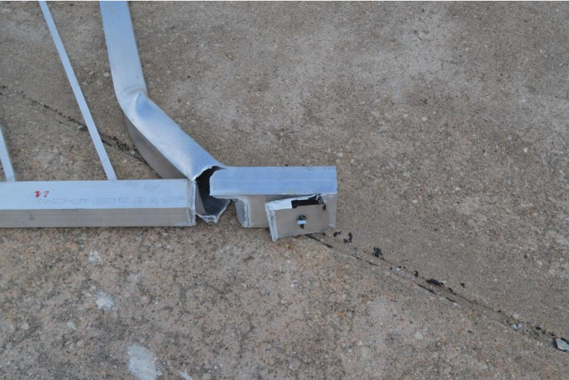
Figure 141. Second Panel Damage, Run No. WIPR-2, Test No. WIPR-2-2
