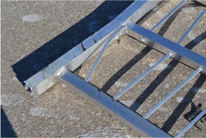
Figure 202. Panel No. 6 Damage, Test No. APR-2
