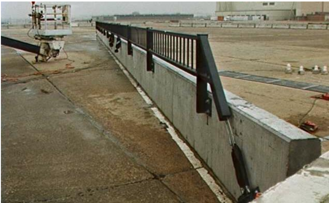
Figure 6. Minnesota Combination Traffic and Pedestrian Barrier [10]
