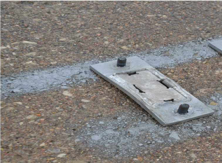
Figure 200. Panel No. 4 Damage, Test No. APR-2
