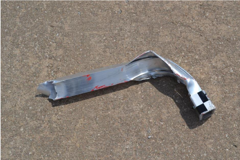
Figure 140. First Panel Damage, Run No. WIPR-2, Test No. WIPR-2-2
