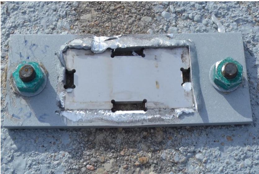
Figure 185. Panel No. 14 Damage, Test No. APR-1
