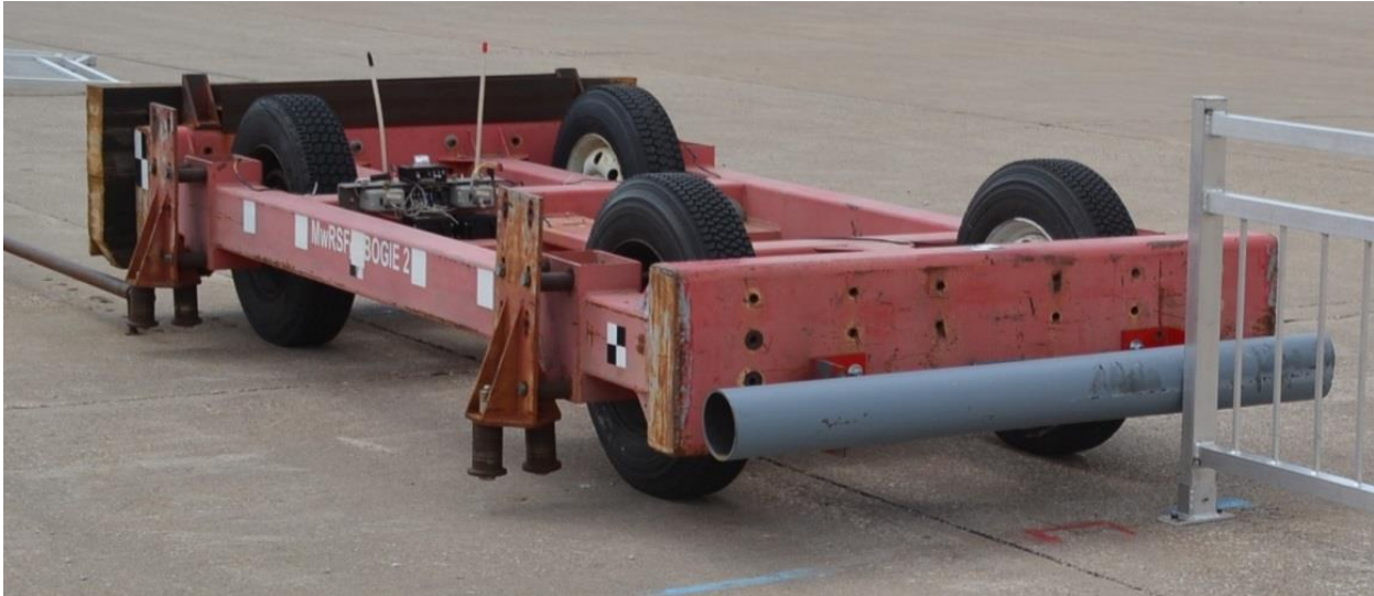
Figure 127. Rigid-Frame Bogie Vehicle on Guidance Track
