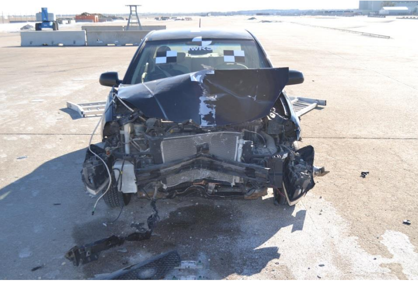
Figure 207. Vehicle Damage, Test No. APR-2
