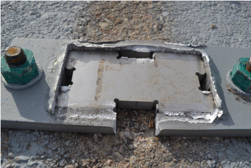
Figure 186. Panel No. 15 Damage, Test No. APR-1
