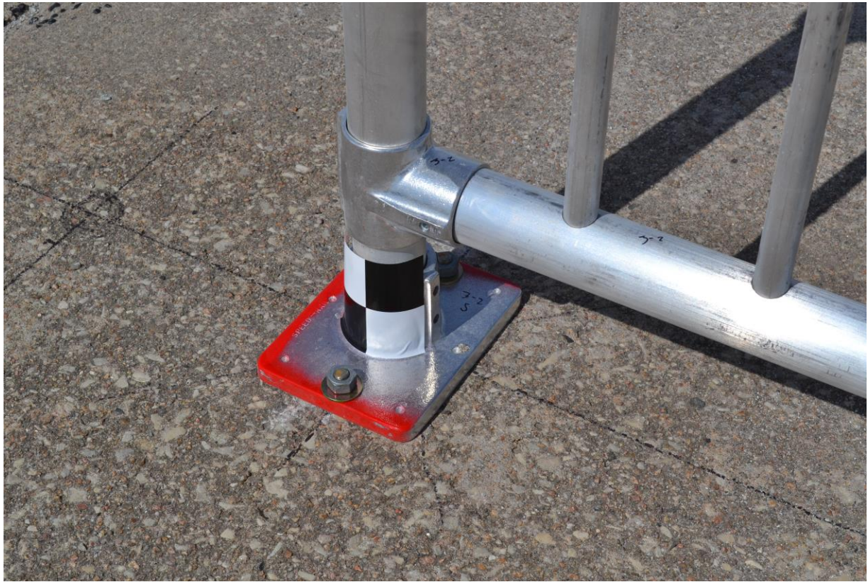
Figure 142. System Panels and Anchor, Run No. WIPR-3
