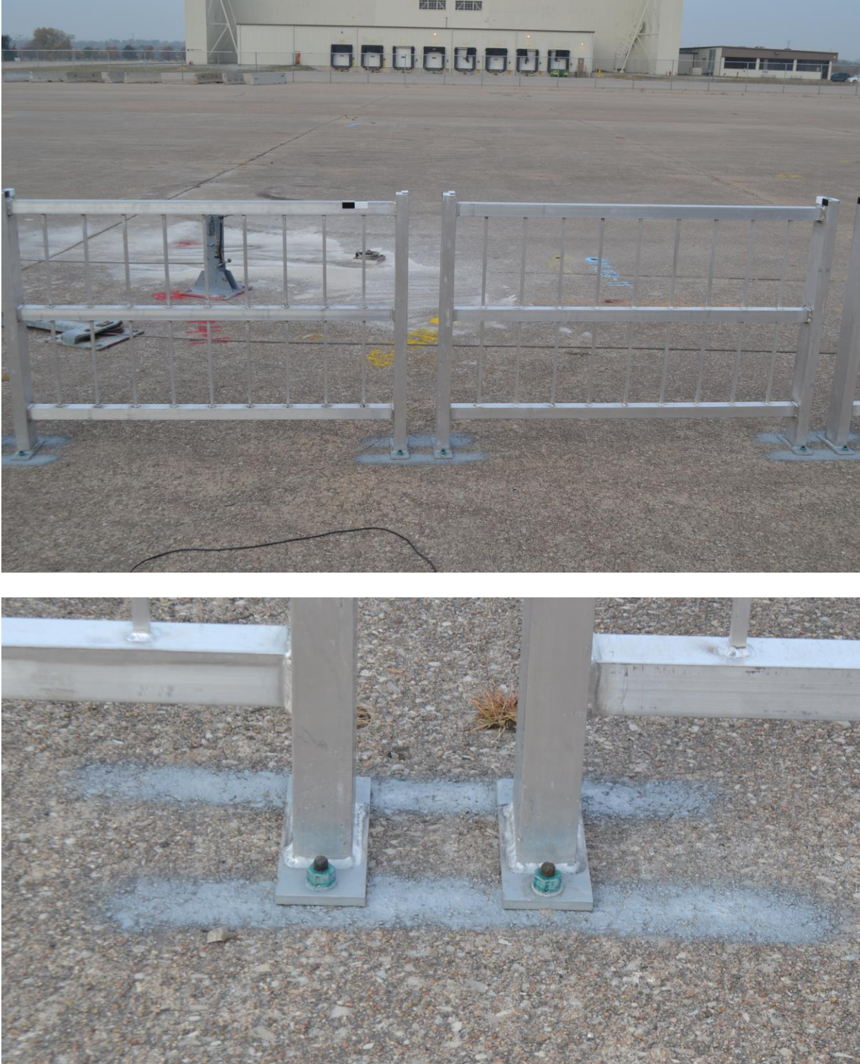
Figure 173. System Panels and Anchors, Test No. APR-1
