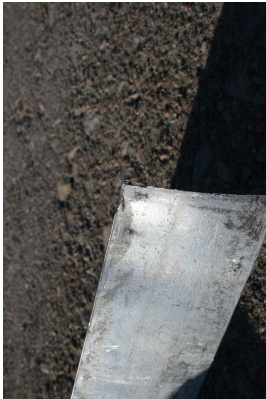
Figure 76. System Damage – Fractured Energy Absorber Tape, Test No. IRA-1
