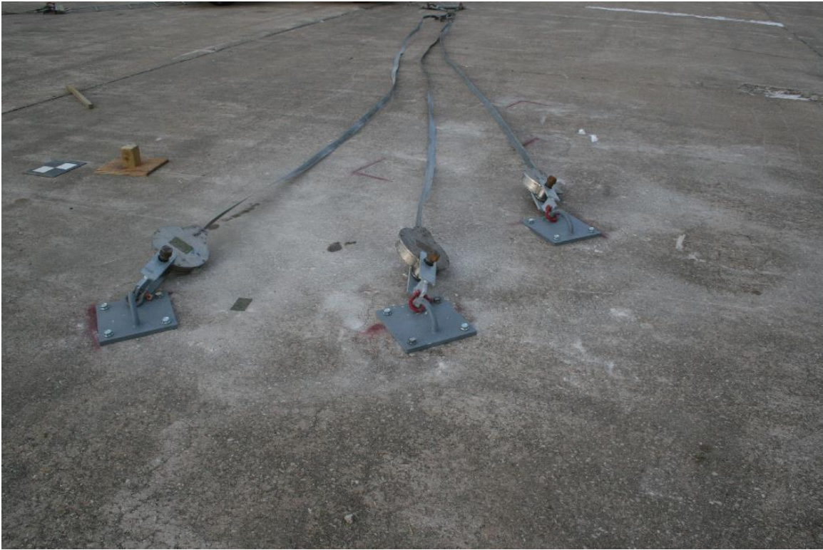
Figure 85. System Damage, Test No. IRA-2
