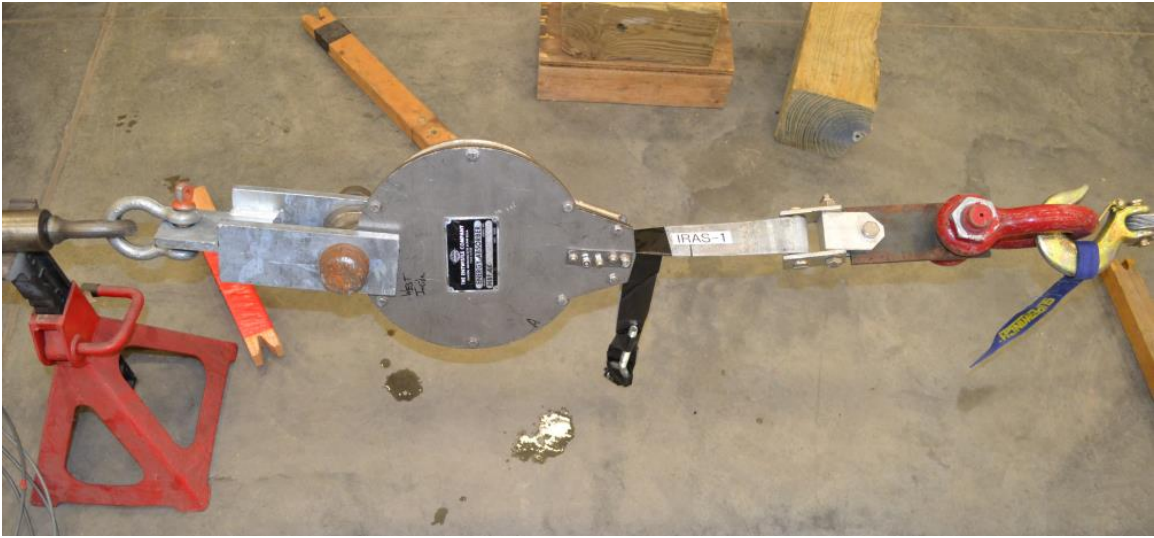
Figure 33. Energy Absorber Component Testing, Test No. IRAS-1
