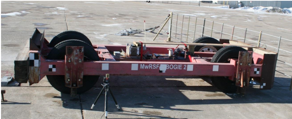
Figure 37. Rigid-Frame Bogie on Guidance Track
