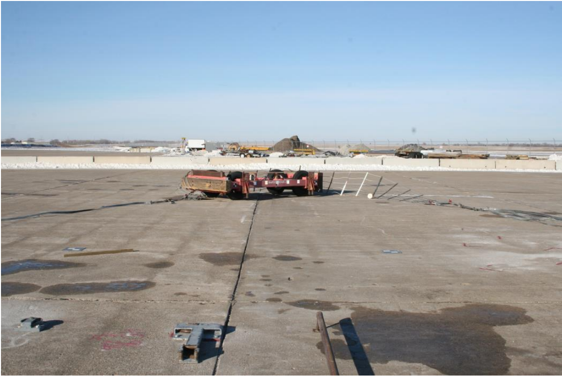
Figure 74. Vehicle Final Position and Trajectory Marks, Test No. IRA-1
