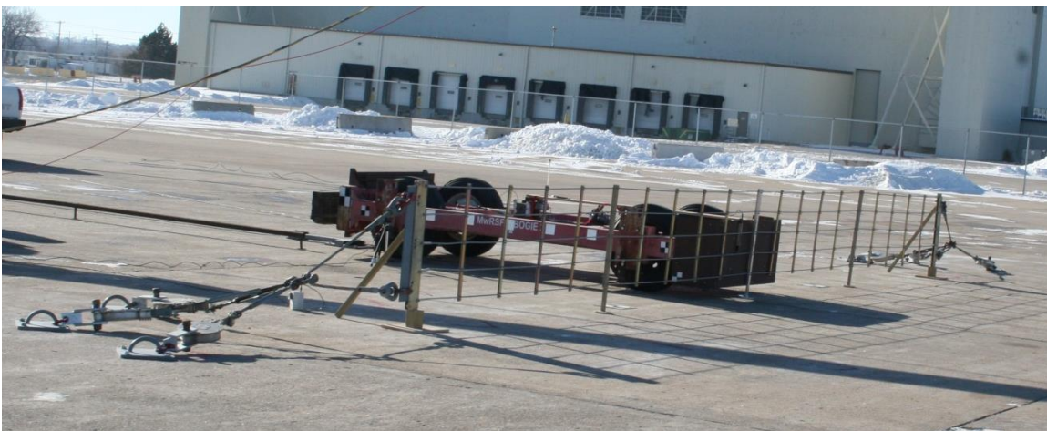
Figure 131. Modified Dragnet Vehicle Arresting Barrier, Test No. IRA-4
