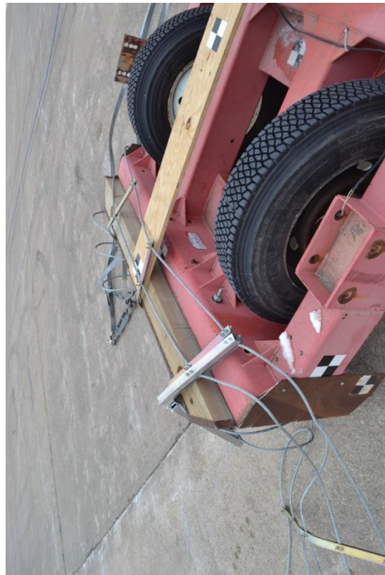
Figure 119. System and Vehicle Damage – Fractured Support Post, Test No. IRA-3
