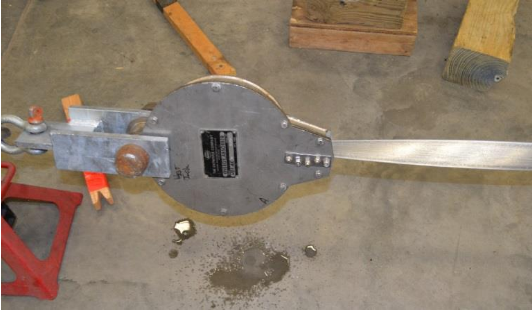
Figure 35. Energy Absorber Component Testing, Test No. IRAS-2
