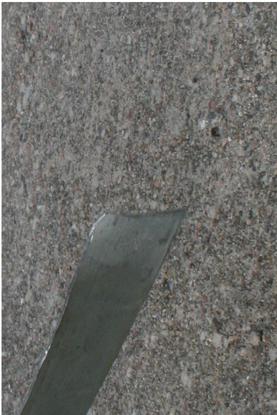
Figure 86. System Damage – Fractured Energy Absorber Tape, Test No. IRA-2
