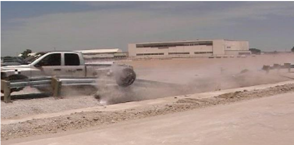
Figure 34. Sequentials – Test No. LSC-2 and LS-DYNA Simulation with Silverado-v2-SF
