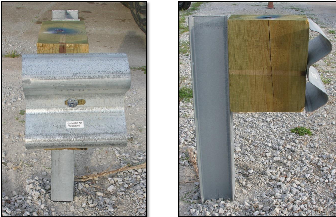
Figure 114. Test Setup to Measure Guardrail Bolt Torque
