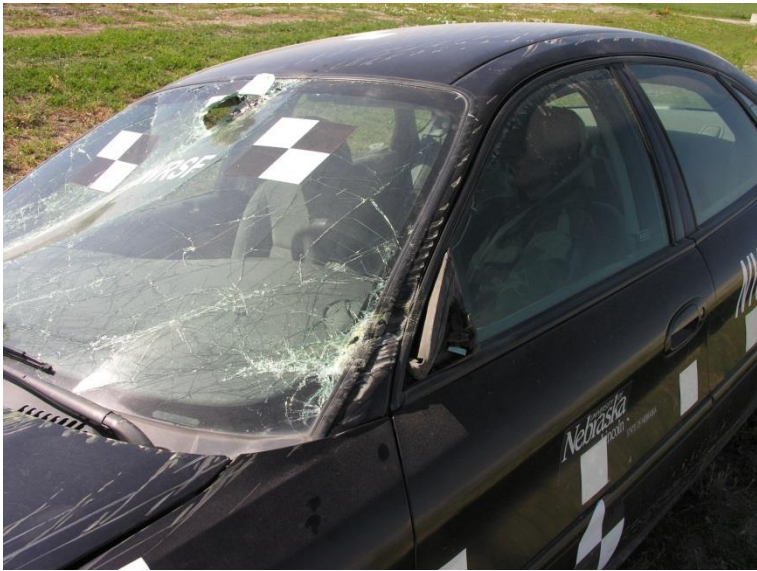
Figure 53. Vehicle Damage, Test No. NYJ-1
