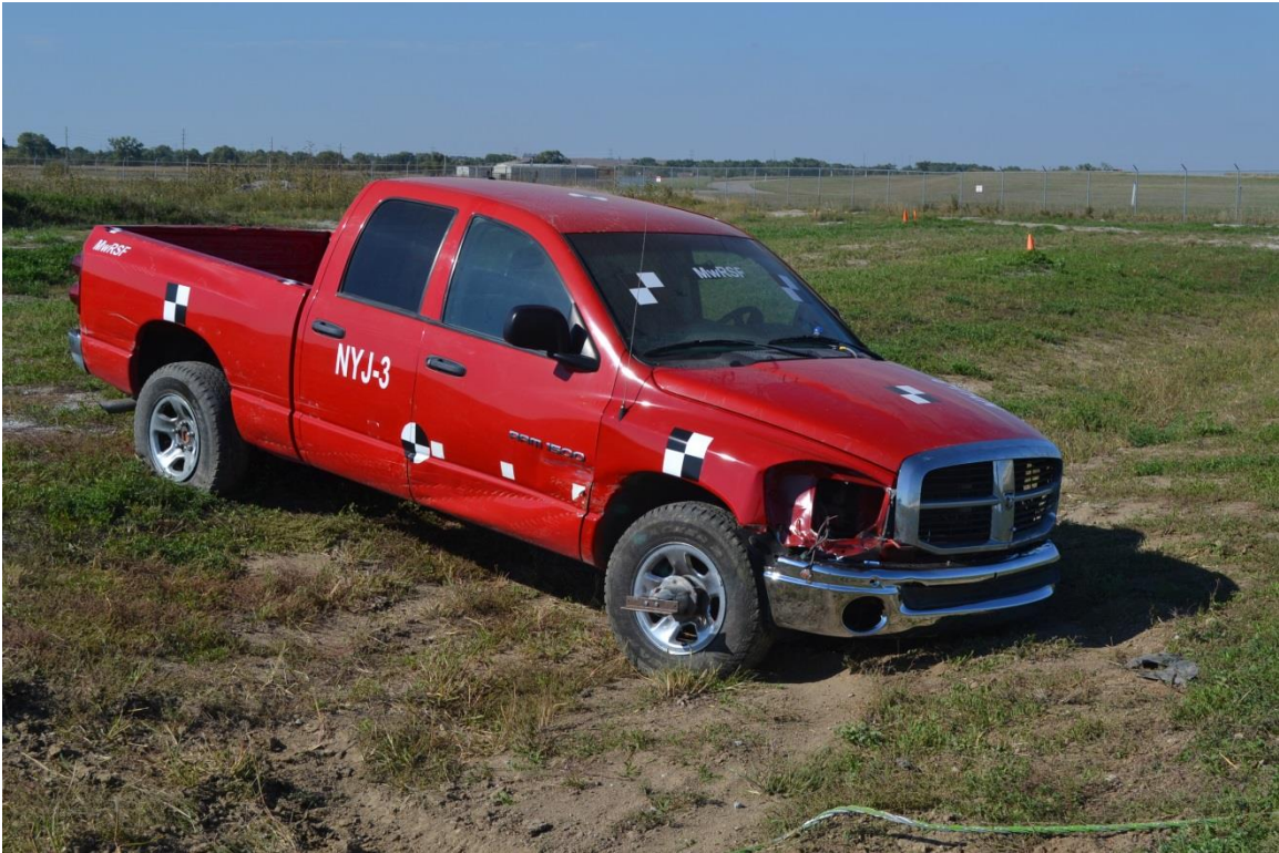
Figure 98. Vehicle Damage, Test No. NYJ-3
