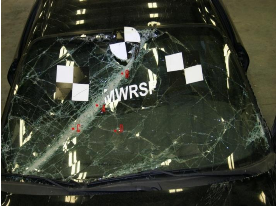
Figure E-7. Windshield Crush, Test No. NYJ-1
