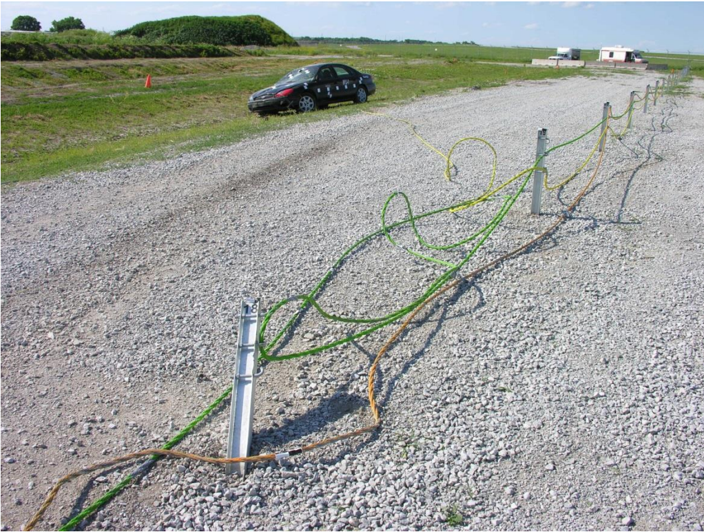
Figure 47. Post Damage in Impact Region, Test No. NYJ-1
