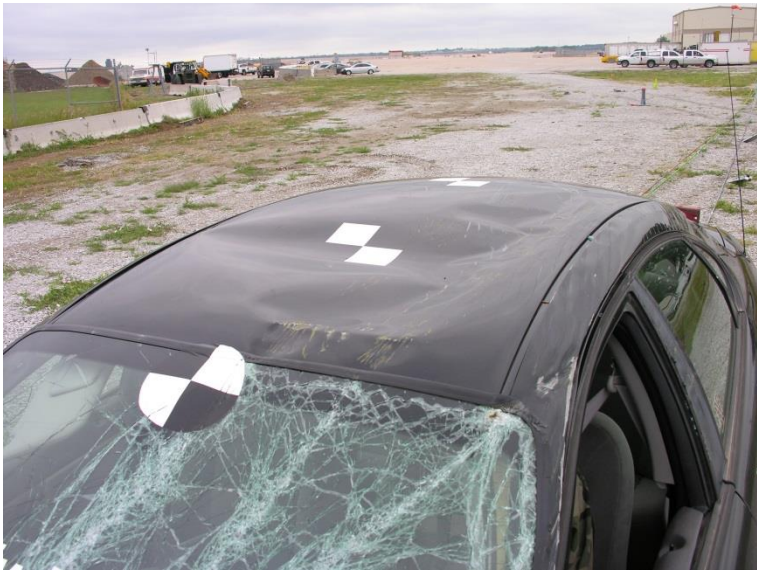
Figure 85. Vehicle Damage, Test No. NYJ-2
