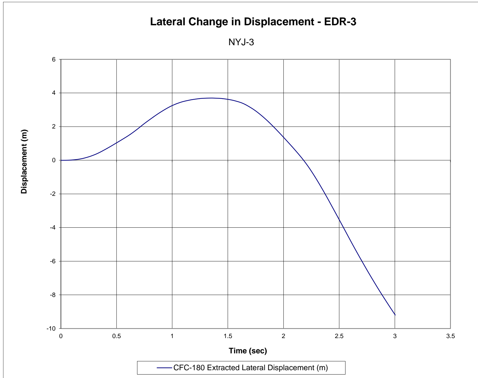
Figure H-22. Lateral Occupant Displacement (EDR-3), Test No. NYJ-3
