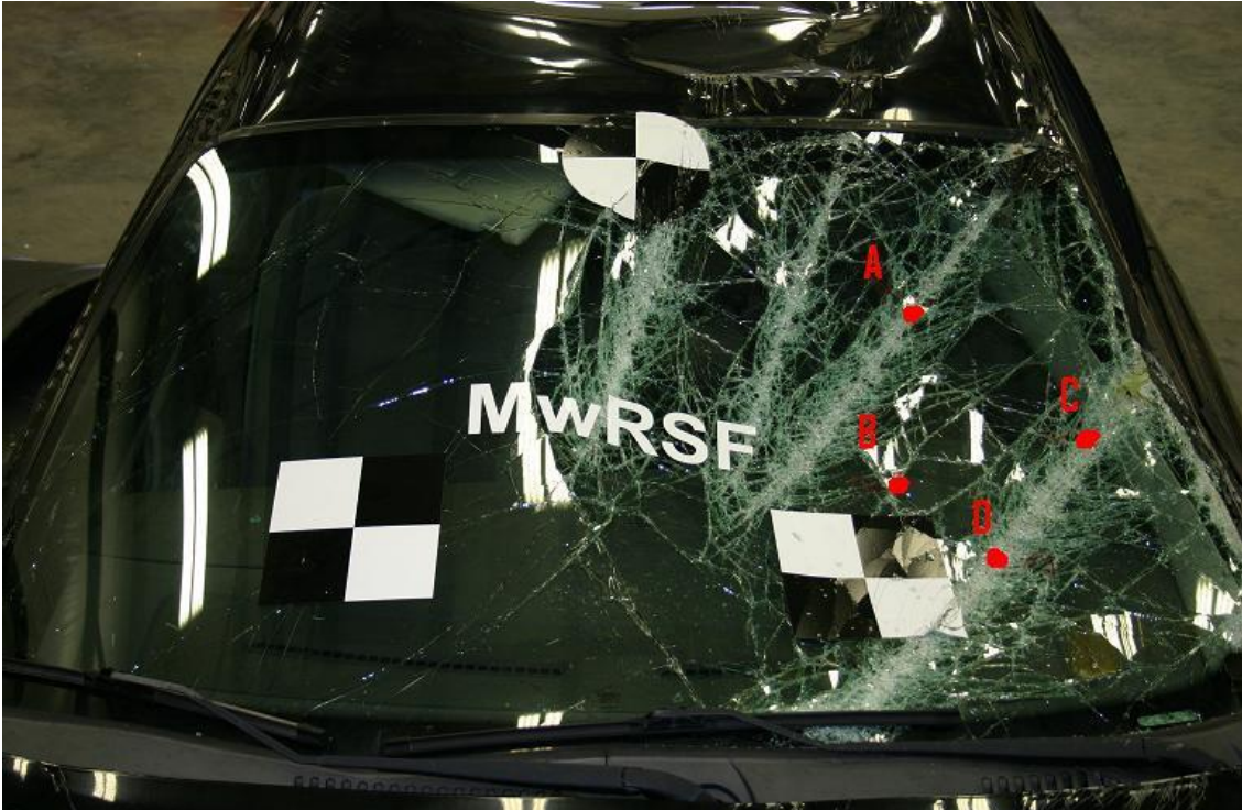
Figure E-14. Windshield Crush, Test No. NYJ-2
