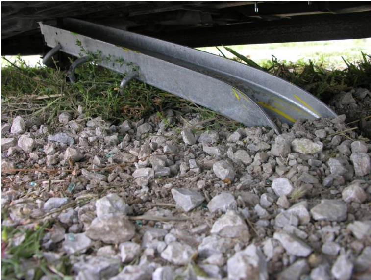
Figure 83. Post Damage for Post Nos. 19, 20, 21, and 40, Test No. NYJ-2
