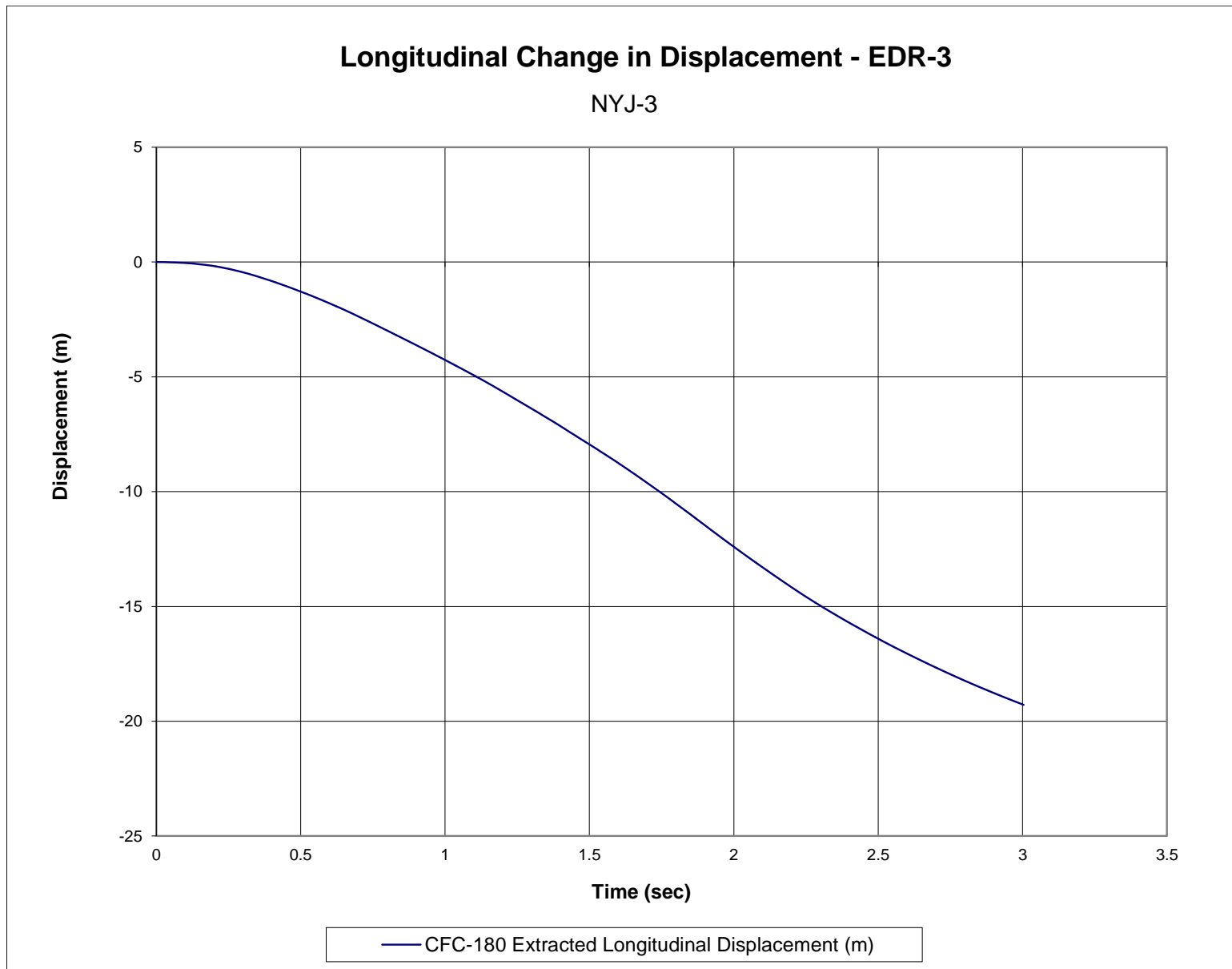
Figure H-19. Longitudinal Occupant Displacement (EDR-3), Test No. NYJ-3
