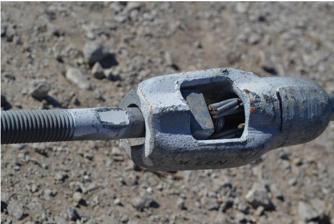
Figure 97. Cable End Fitting Damage, Test No. NYJ-3
