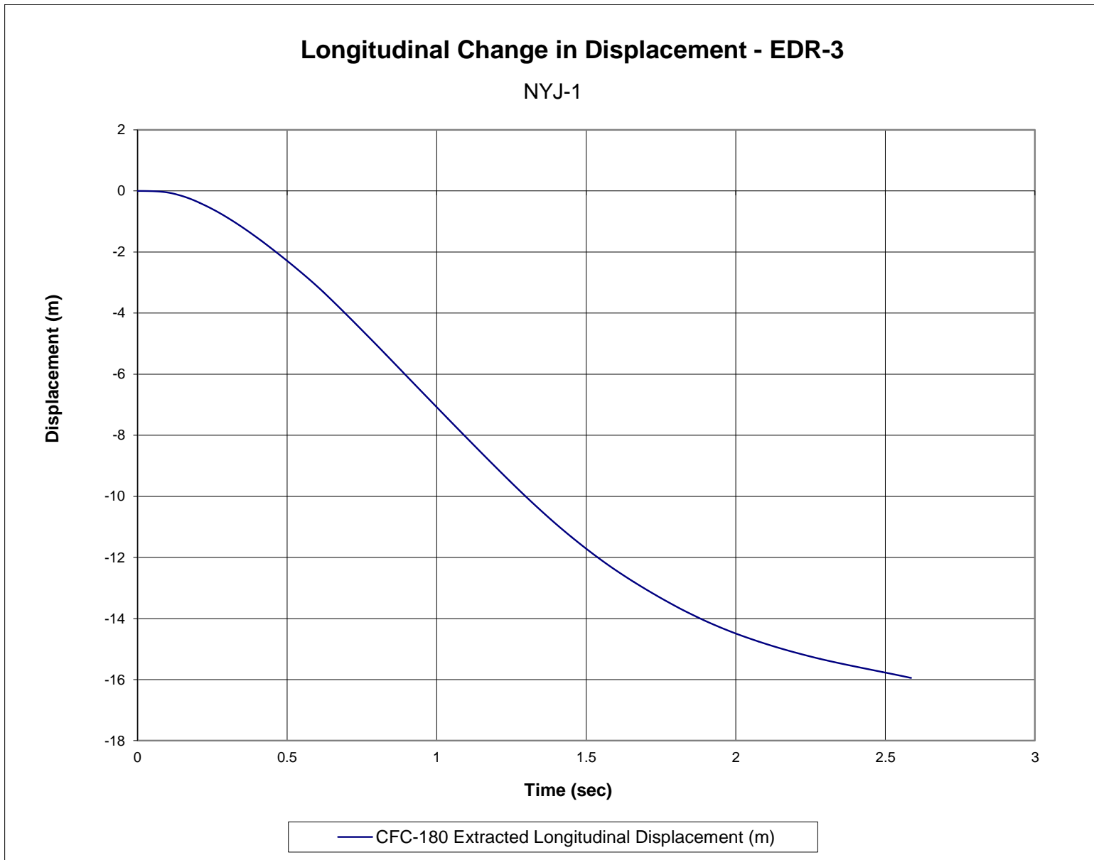
Figure F-19. Longitudinal Occupant Displacement (EDR-3), Test No. NYJ-1
