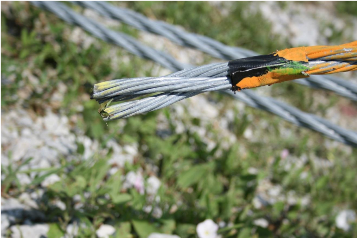
Figure 50. Hardware Fractures and Frayed Cable, Test No. NYJ-1
