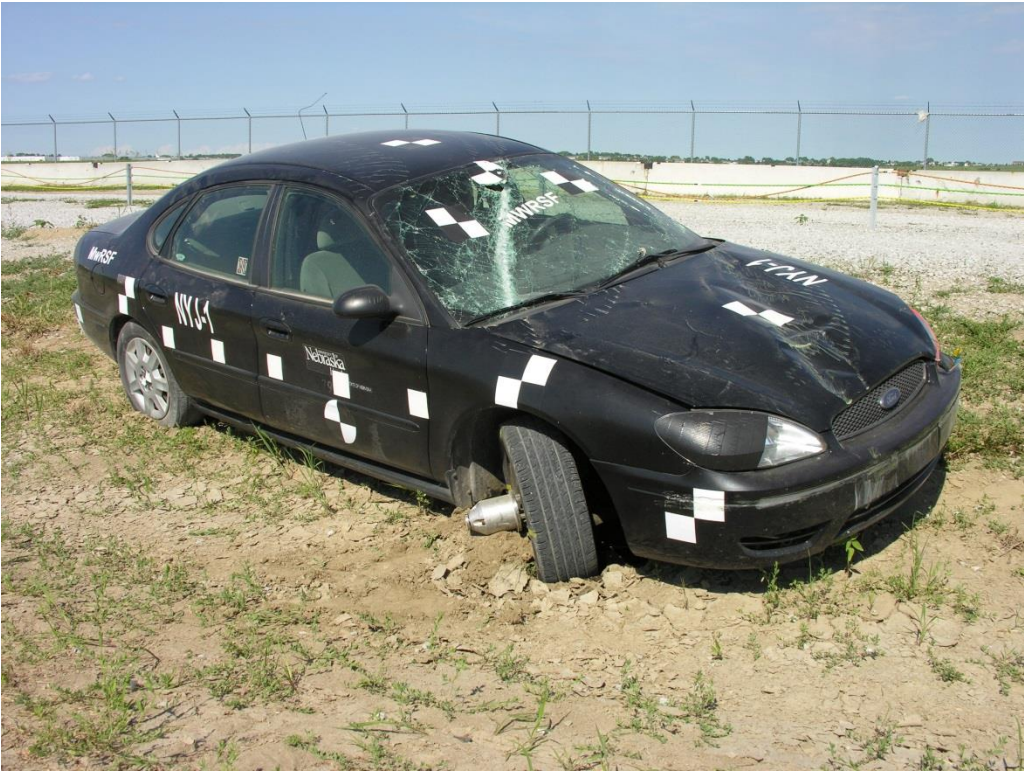
Figure 54. Vehicle Damage, Test No. NYJ-1
