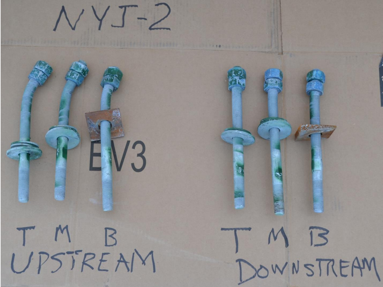
Figure 88. Top, Middle, and Bottom Cable Barrier Termination Threaded Rods for Upstream and Downstream Anchors
