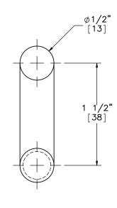
Note: For testing purposes, the j-bolt may be fabricated from ASTM A36 round bar stock which is bent and threads cut and then galvanized.
