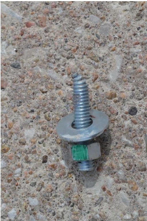
Figure 30. Fractured Bolts, Test No. UBSPB-6
