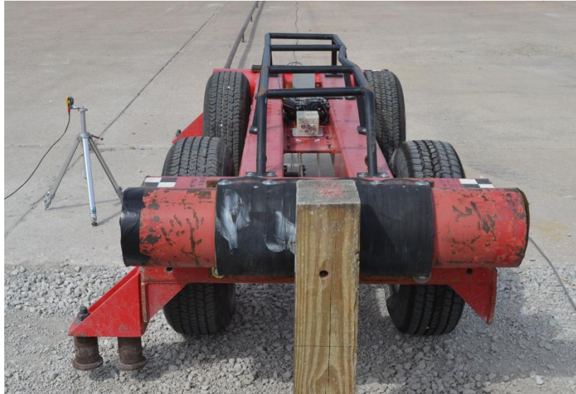
Figure 2. Rigid Frame Bogie and Guidance Track
