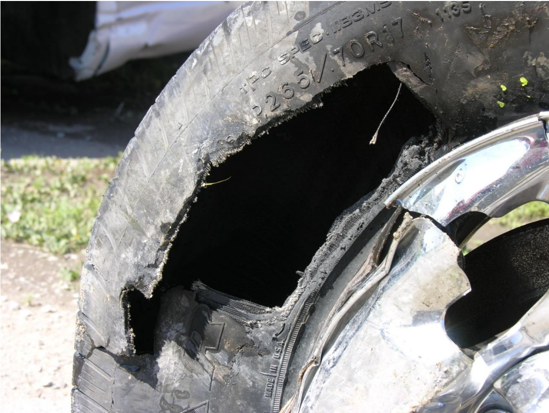
Figure 8. Outside of Wheel Damage, Test No. PCMB-1
