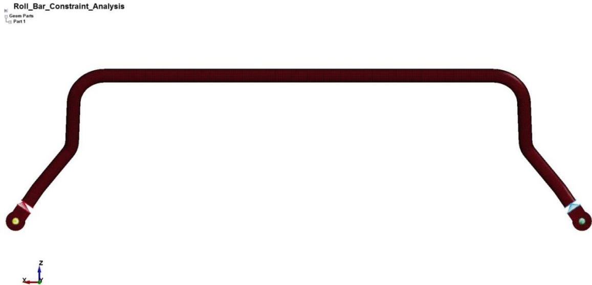
Figure B-3. Simulated Anti-Roll Bar, Pins, and Lower Control Arms
