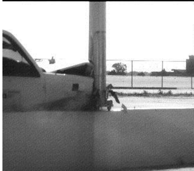
Figure 34. Fender Impact with a Rigid Pole [11]
