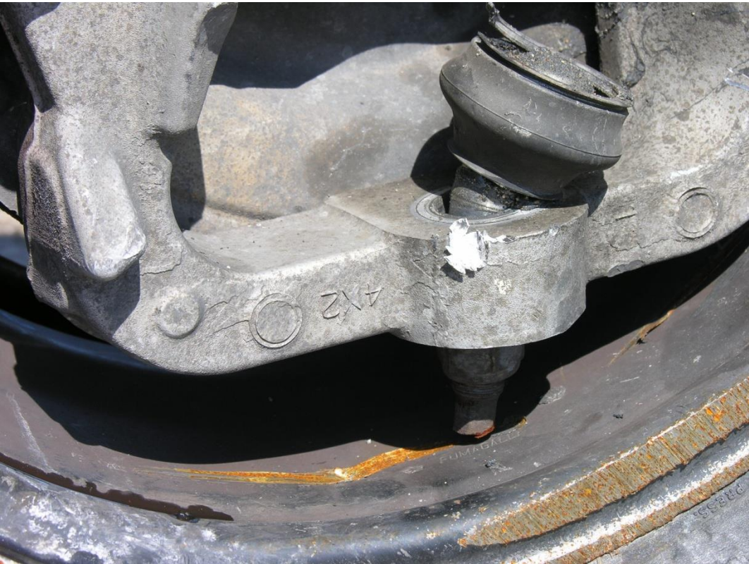
Figure 7. Inside of Wheel Damage, Test No. PCMB-1
