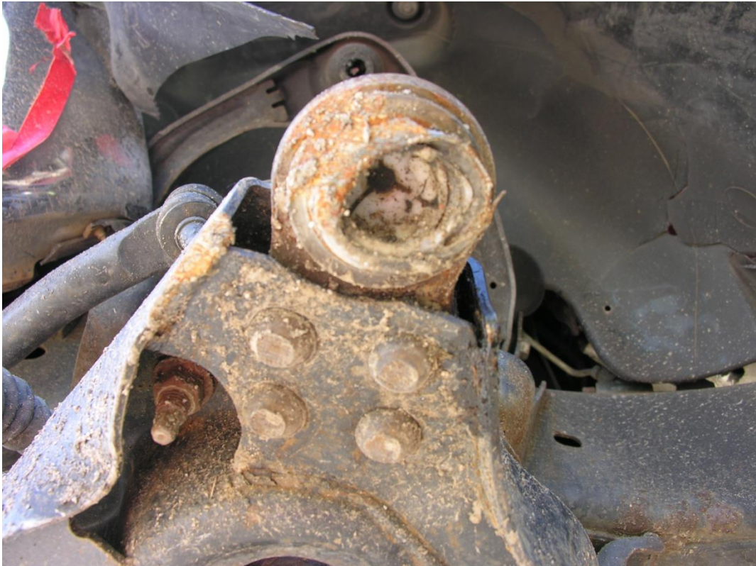
Figure 9. Lower Control Arm Damage, Test No. PCMB-1
