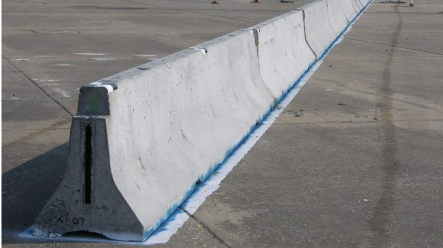
a) Free-Standing Temporary Concrete Barriers
