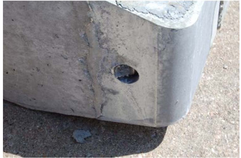
Figure 161. Component Damage – Short Rail Segment, Test No. PCRB-5
