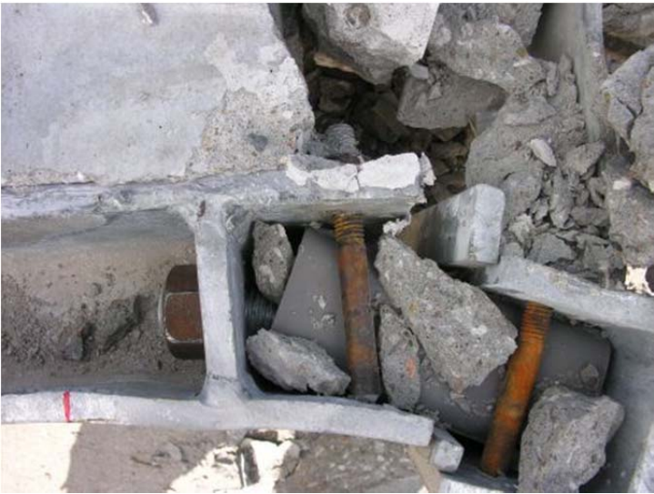
Figure 87. Component Damage - Front Pocket Assembly, Test No. PCRB-2
