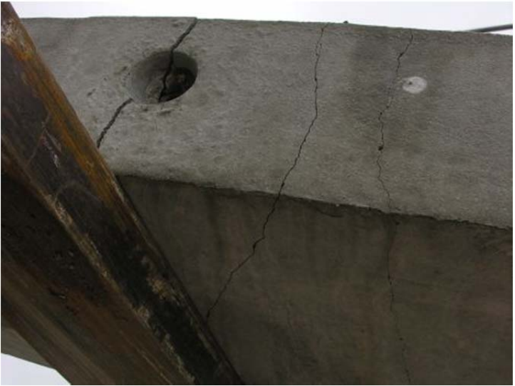
Figure 150. Rail Tension Cracks and Damage to Bottom of Joint, Test No. PCRB-3
