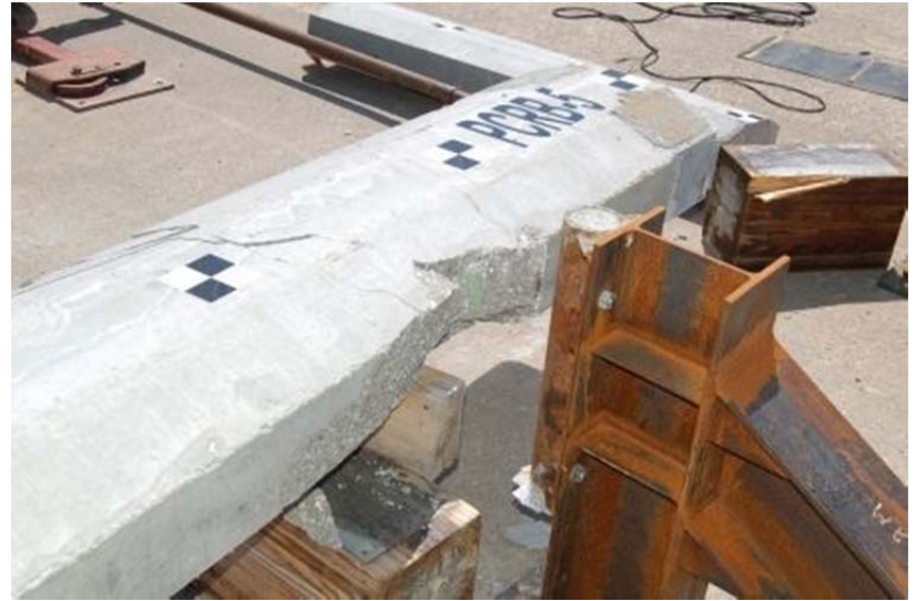
Figure 160. Component Damage, Test No. PCRB-5
