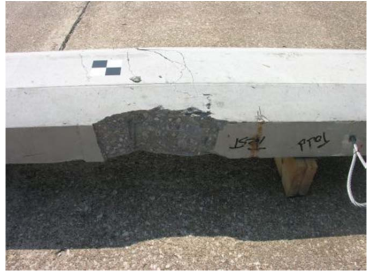
Figure 81. Bending Damage of Long Rail Segment, Test No. PCRB-1
