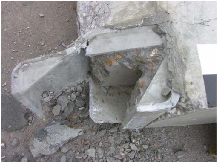
Figure 80. Component Damage – Short Rail Segment, Test No. PCRB-1
