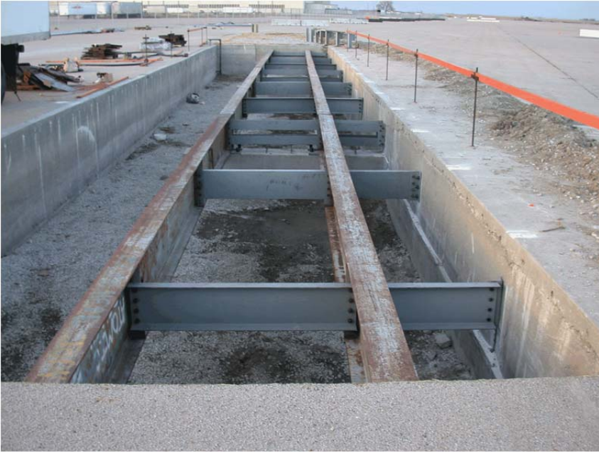
Figure 210. MwRSF Simulated Bridge Test Pit
