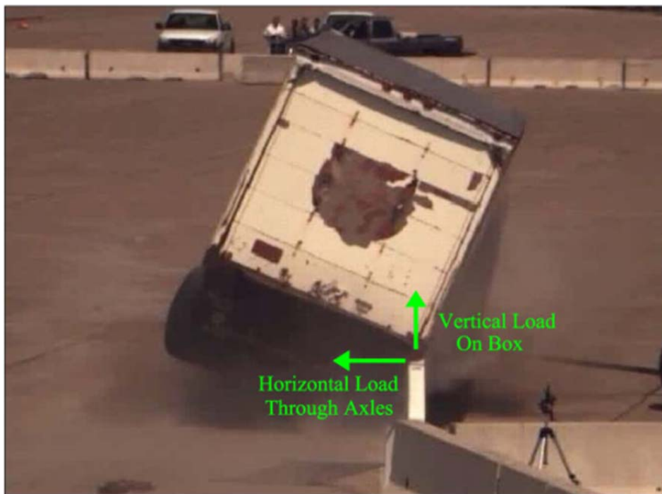
Figure 3. Barrier Forces Acting on Single-Unit Truck During Impact
