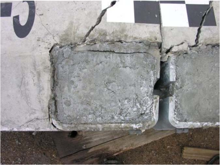
Figure 149. Component Damage – Steel Pockets, Test No. PCRB-3
