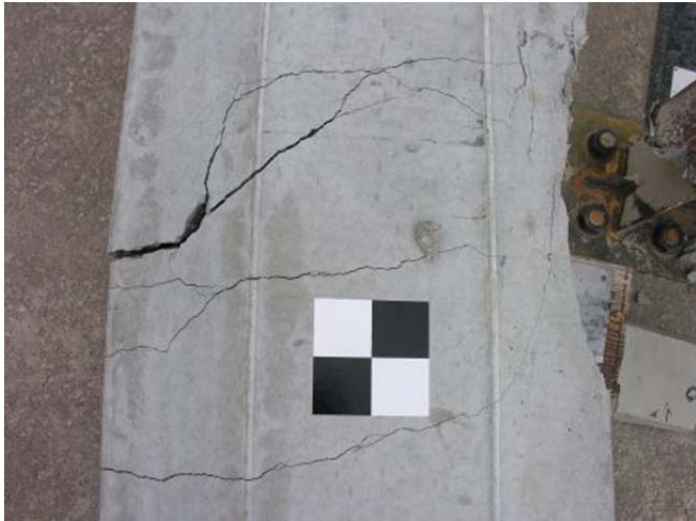
Figure 81. Bending Damage of Long Rail Segment, Test No. PCRB-1
