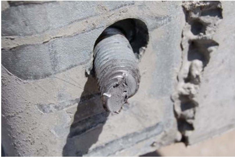
Figure 162. Component Damage – Long Rail Segment, Test No. PCRB-5
