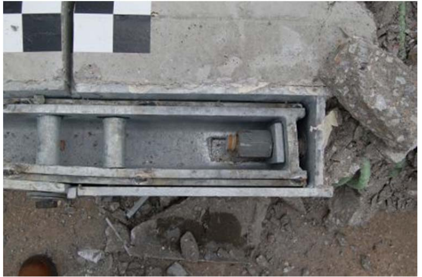
Figure 155. Component Damage – Steel Pockets, Test No. PCRB-4
