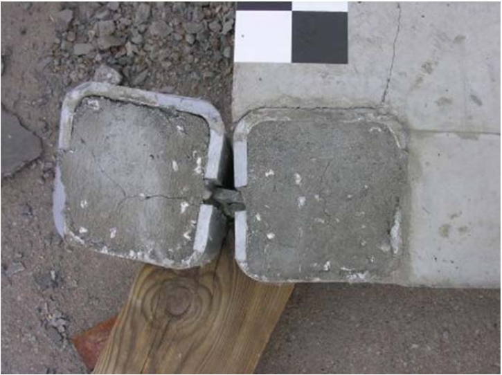
Figure 80. Component Damage – Short Rail Segment, Test No. PCRB-1
