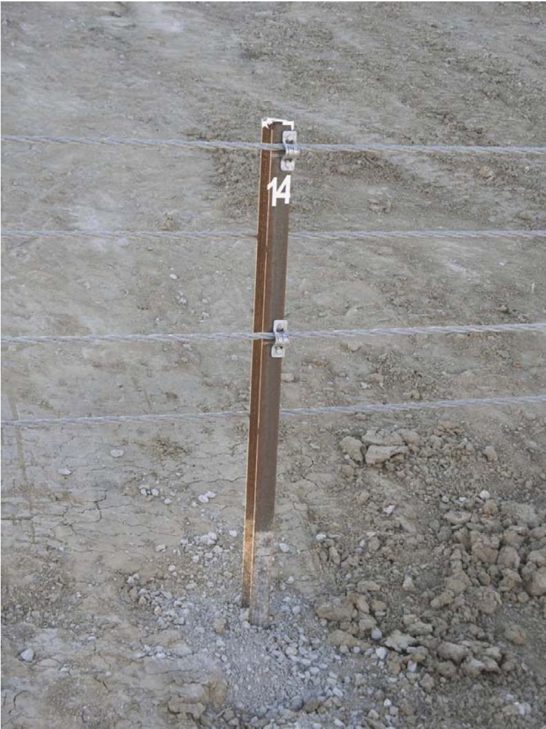
Figure 73. Post Nos. 14 and 15 Damage, Test No. 4CMB-3
