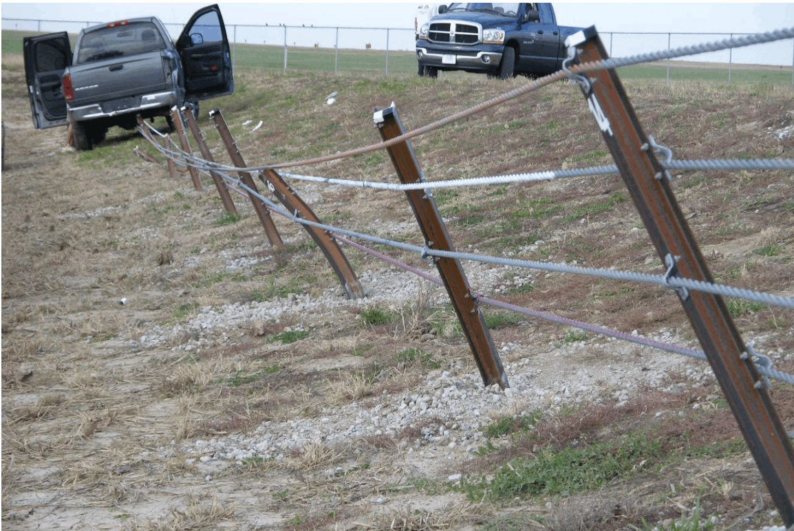
Figure 40. System Damage, Test No. 4CMB-1
