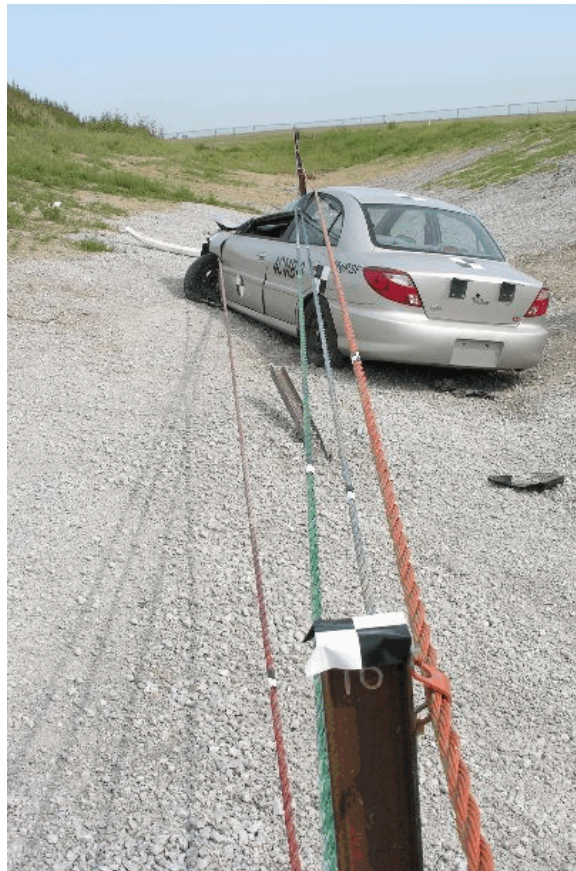
Figure 104. Vehicle Final Position and Trajectory Marks, Test No. 4CMB-3
