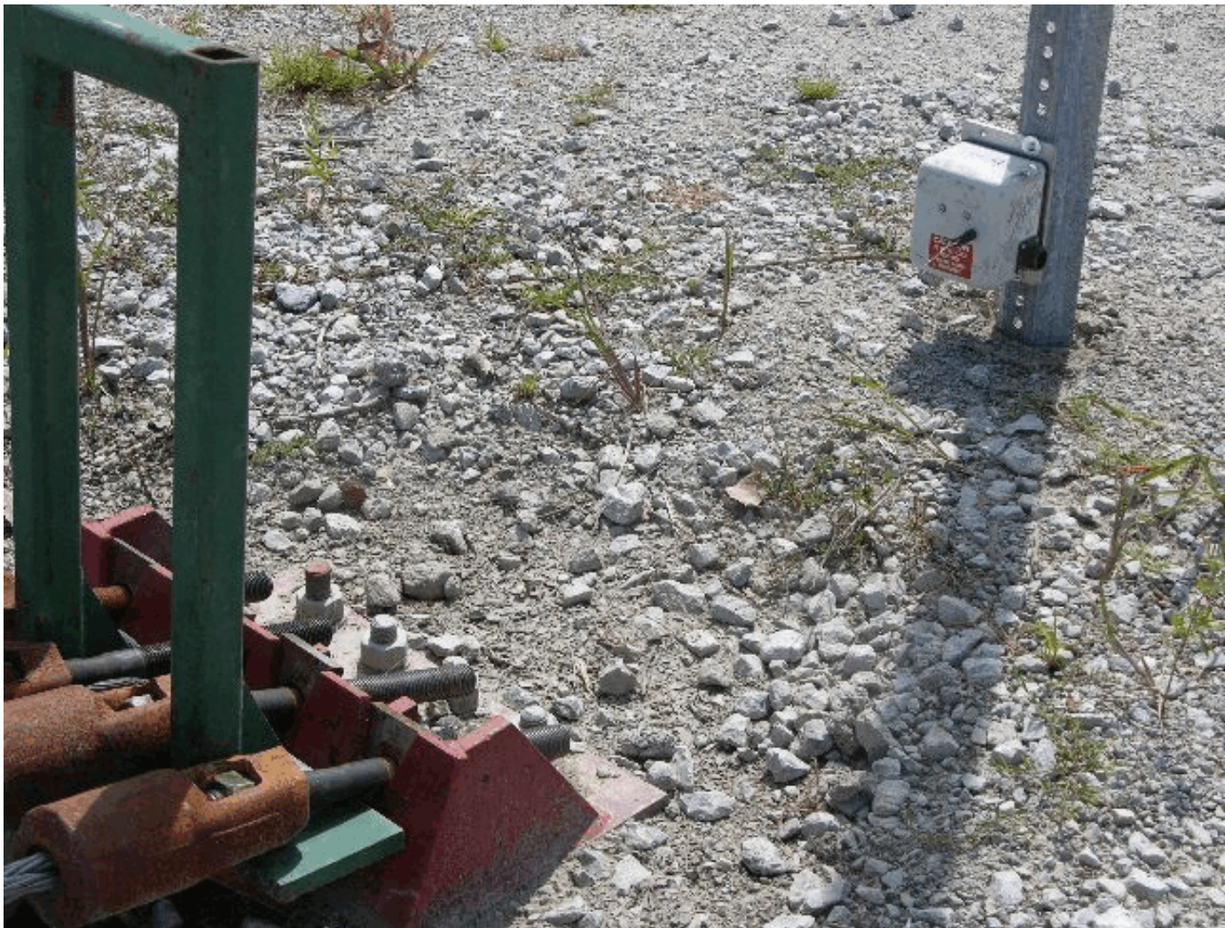
Figure 33. Typical String Potentiometer Positioning
