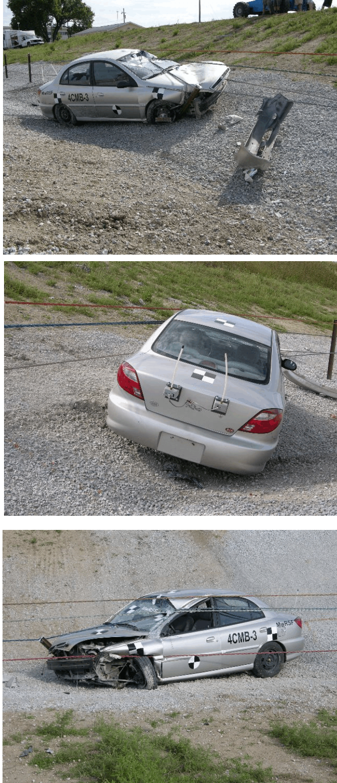
Figure 109. Vehicle Damage, Test No. 4CMB-3
