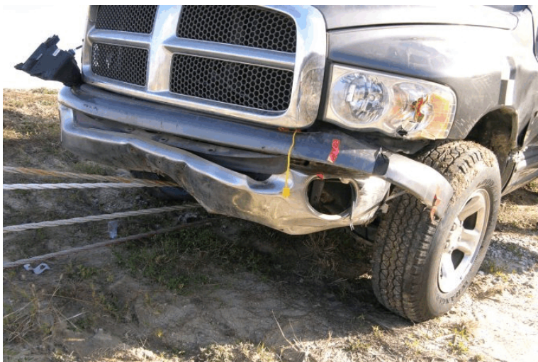
Figure 45. Vehicle Damage, Test No. 4CMB-1
