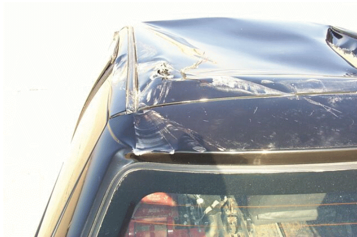
Figure 32. Vehicle Roof Damage, Test MI-1
