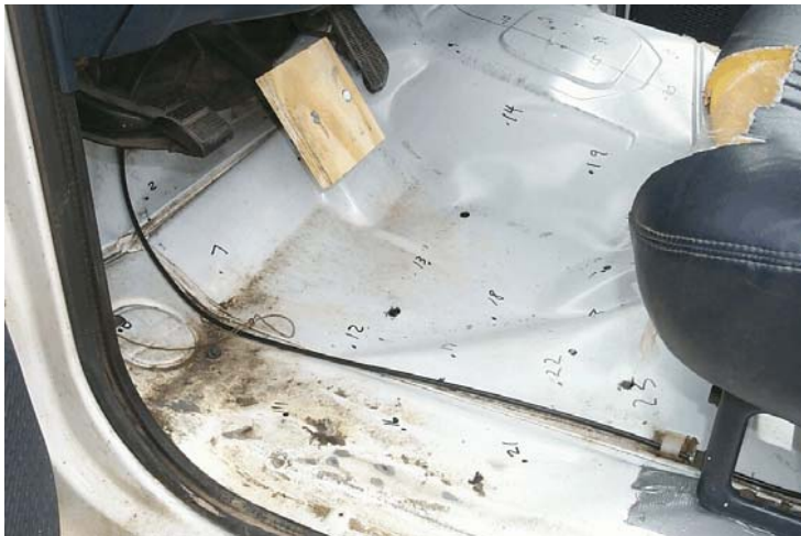
Figure 32. Occupant Compartment Deformations, Test HTB-1
