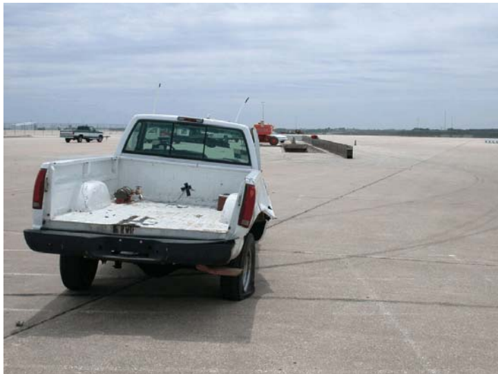
Figure 49. Vehicle Final Position and Trajectory Marks, Test HTB-2
