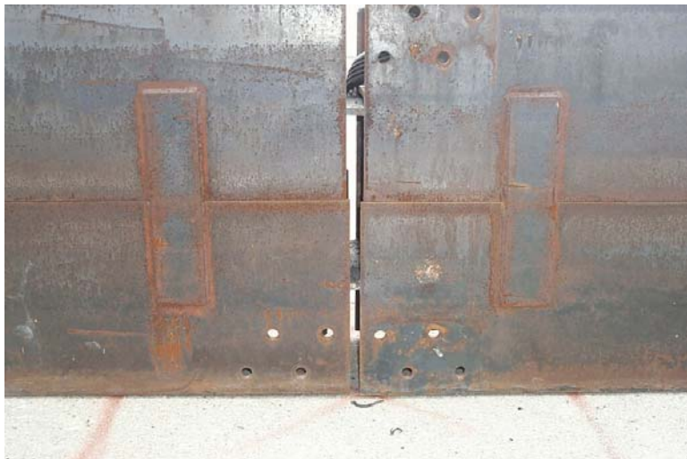
Figure 25. Steel H-section Barrier System Damage, Test HTB-1
