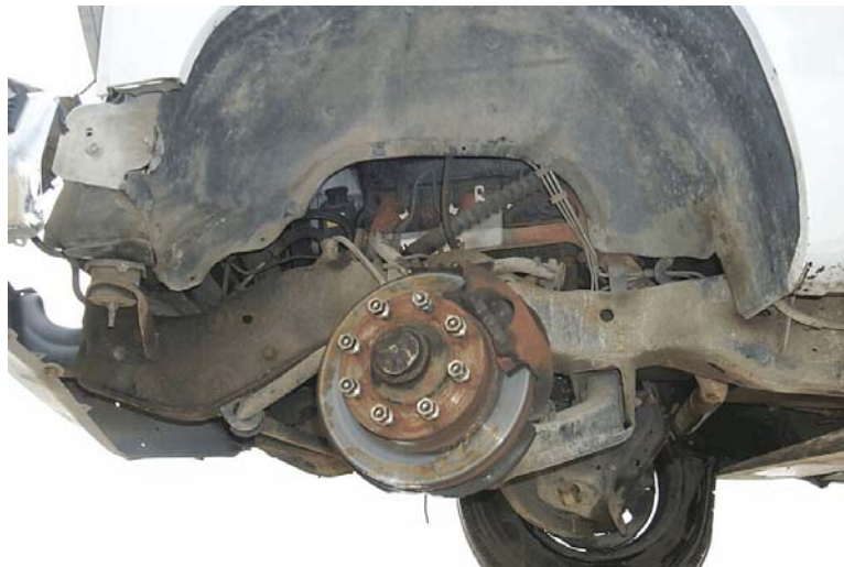
Figure 31. Undercarriage Vehicle Damage, Test HTB-1
