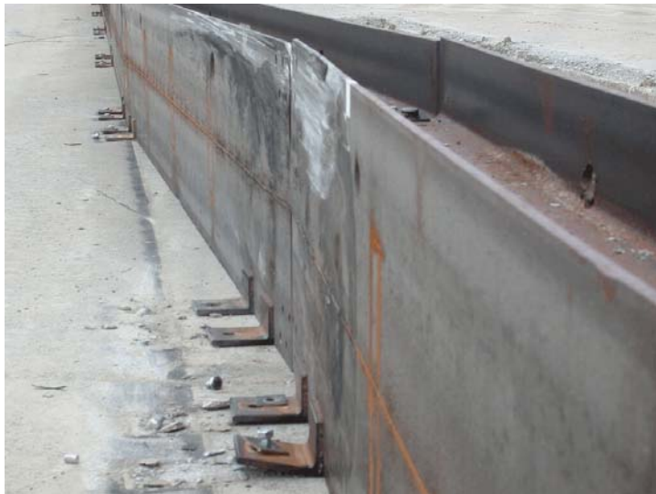
Figure 51. Steel H-section Barrier System Damage, Test HTB-2
