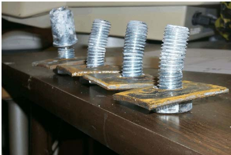
Figure 27. Tie-Down Anchor Bolt Damage, Test HTB-1
