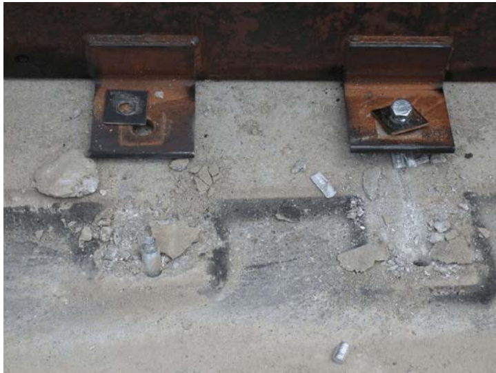
Figure 54. Tie-Down Anchor Damage, Test HTB-2
