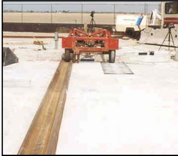
Figure 5. Bogie Positioned in the Guide Track Configuration
