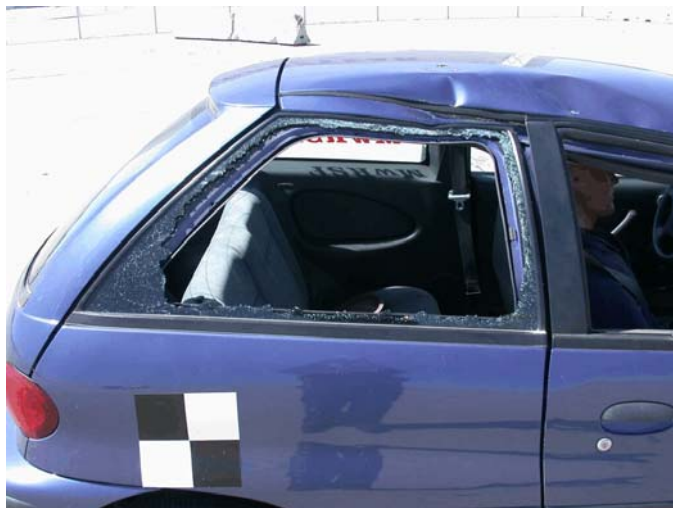
Figure 24. Vehicle Front-End and Right-Side Windows Damage, Test MI-4
