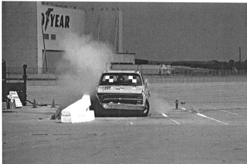
FIGURE 17. Full-Scale Vehicle Crash Test, Test NTBR-1
