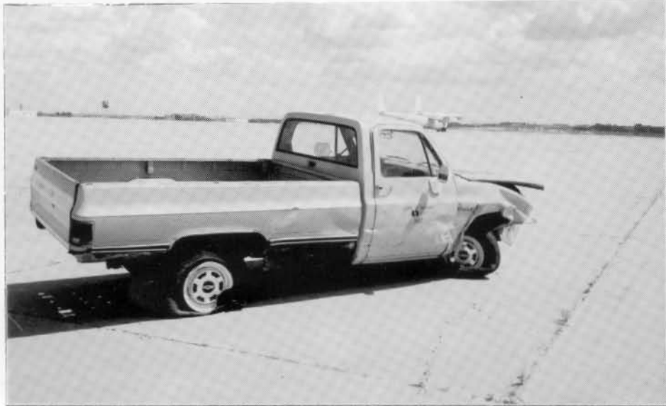
FIGURE 35. Vehicle Damage, NEOCR-1
