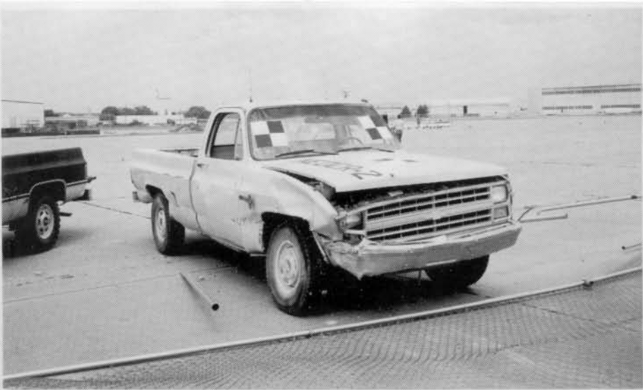
FIGURE 40. Vehicle Damage, NEOCR-2
