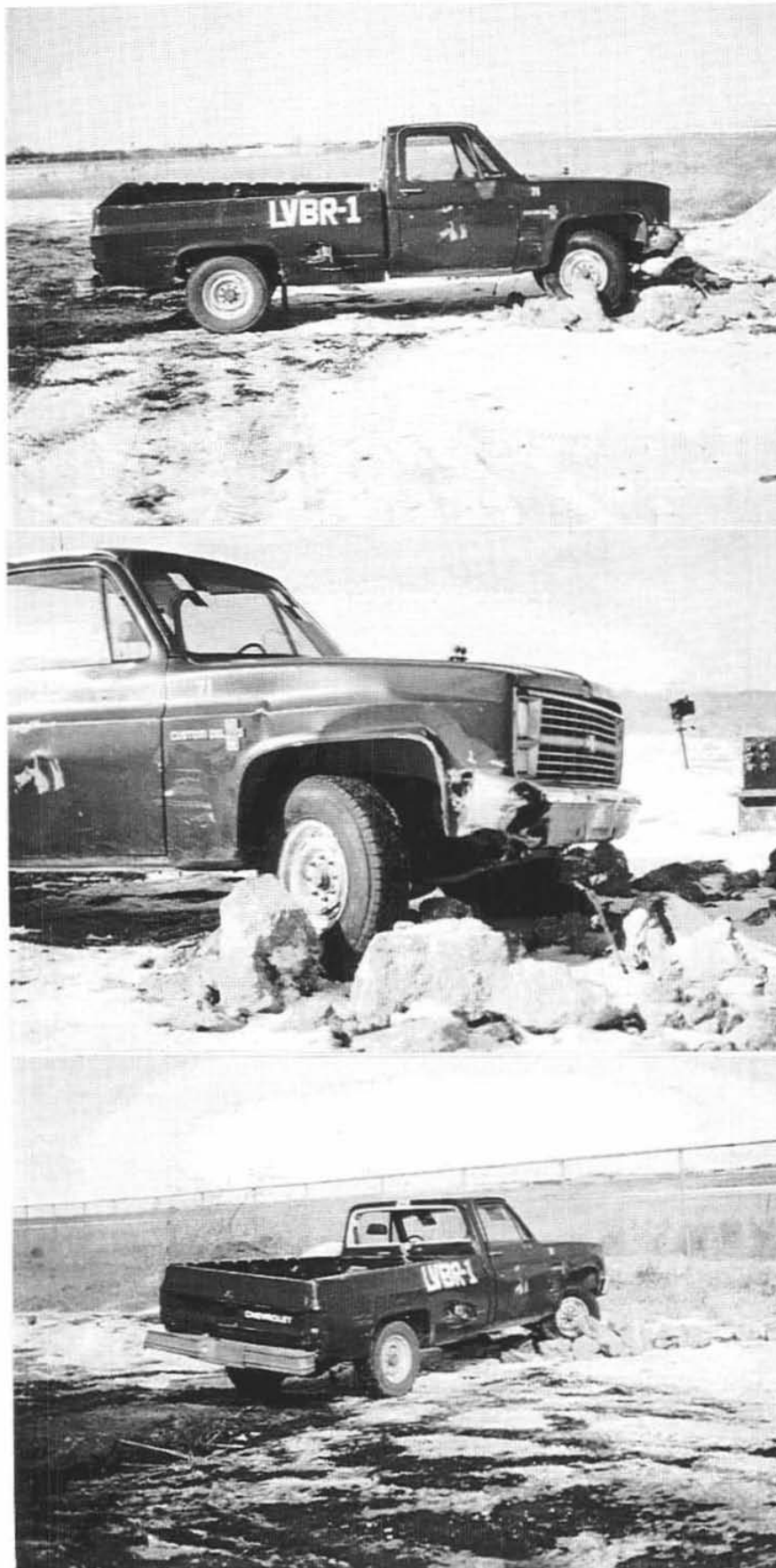
Figure 20. Vehicle Damage, Test LVBR-1
