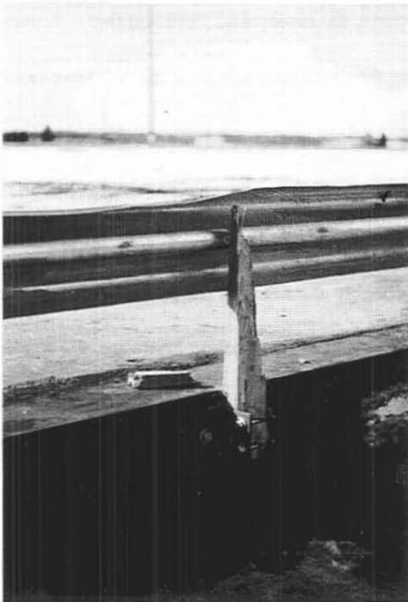
Figure 23. Bridge Post Damage, Test LVBR-1
