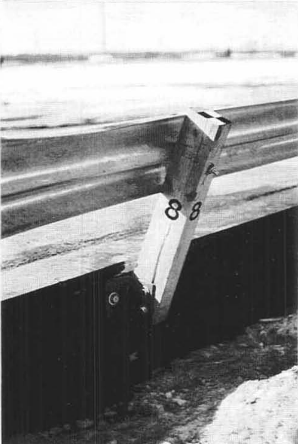
Figure 22. Bridge Post Damage, Test LVBR-1
